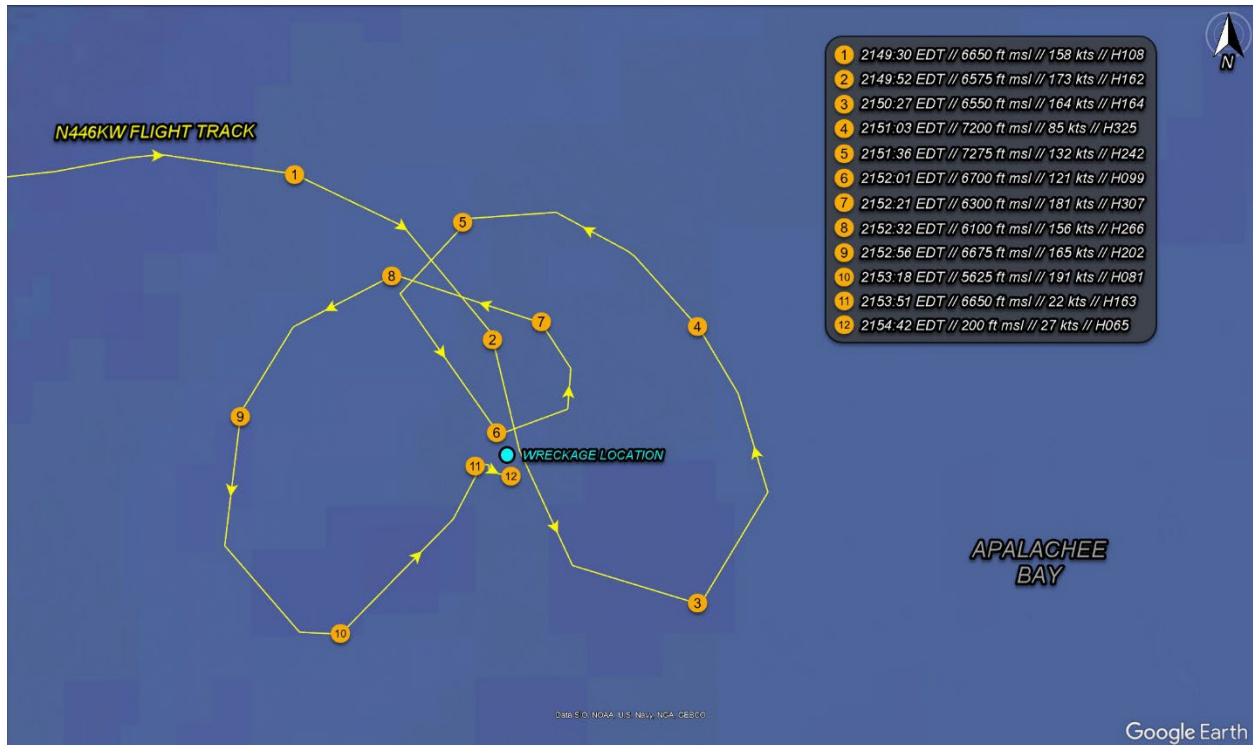
Figure 3. The final segment of the accident flight track of N446KW from an overhead view. Data was overlaid onto satellite imagery, with key flight track information labeled for awareness.
