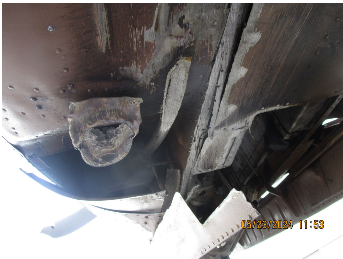
Photograph 2 - View of skid damage through skin to stringers and frames (Courtesy of FAA)
