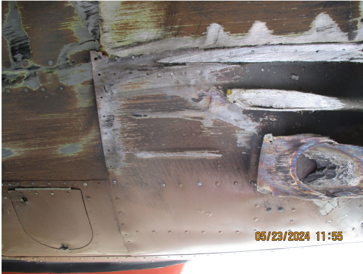
Photograph 3 - View of skid damage through skin to stringers and frames (Courtesy of FAA)
