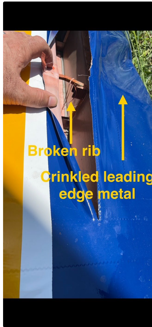
Photograph 4 - Wing rib damage (Courtesy of FAA)
