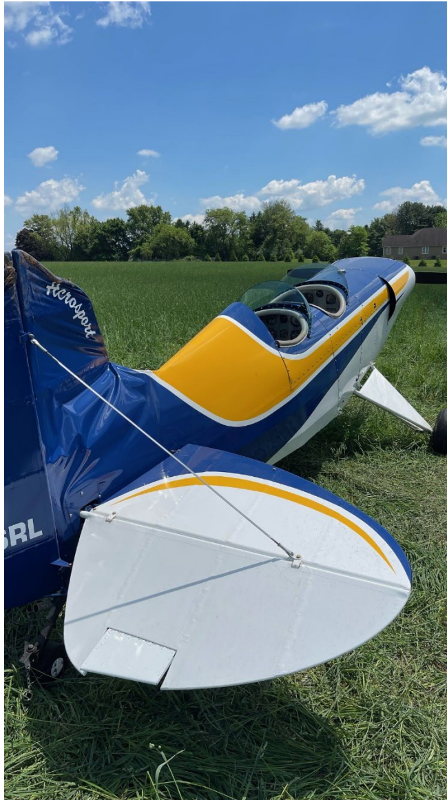
Photograph 3 - Vertical and rudder damage (Courtesy of FAA)
