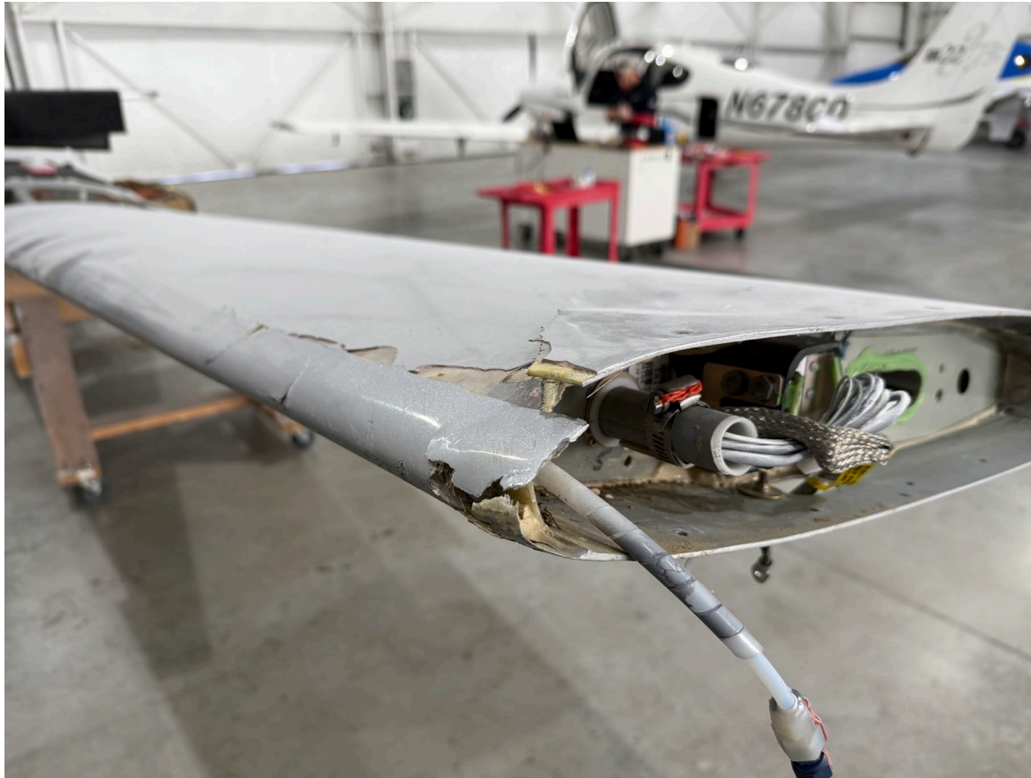
Photograph 5 - Digital Photograph From Repair Facility. View Depicting The Outer Portion of the Left Wing. Note the Damage along the Leading Edge and Also Chordwise
