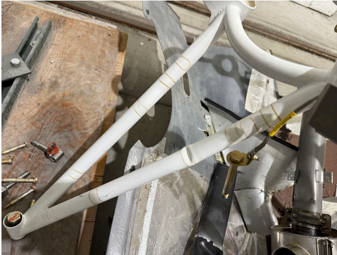
Photograph 4 - Digital Photograph From Repair Facility. View Depicting Compression Buckle in Engine Mount Tube Requiring Major Repair/Replacement
