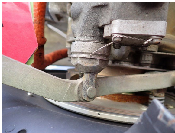
Figure 11 View of the Tested Position of the Left Beta Valve
