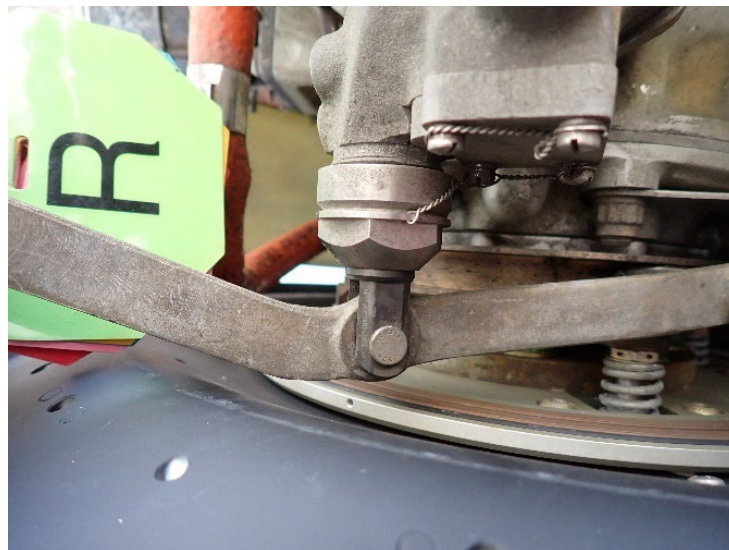
Figure 13 View of the Tested Position of the Right Beta Valve
