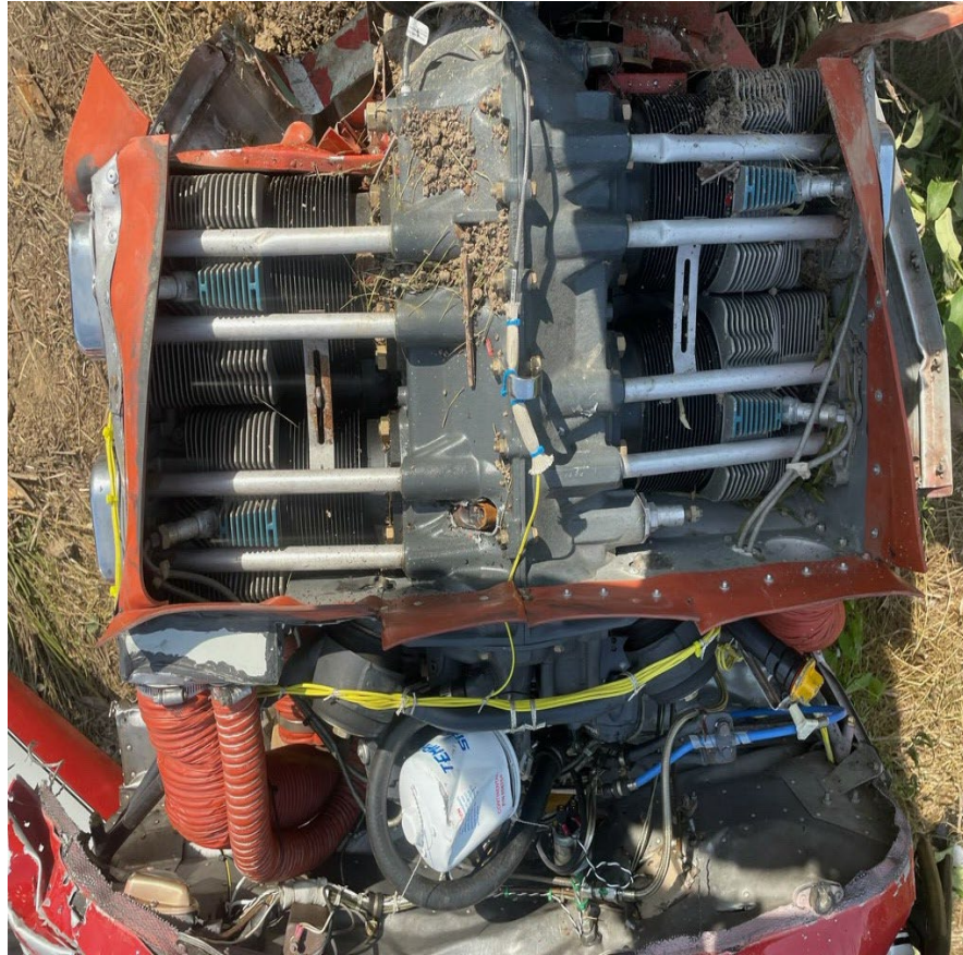
Photograph 2 - View of No. 4 connecting rod protruding to the top of the case. (FAA Photo)
