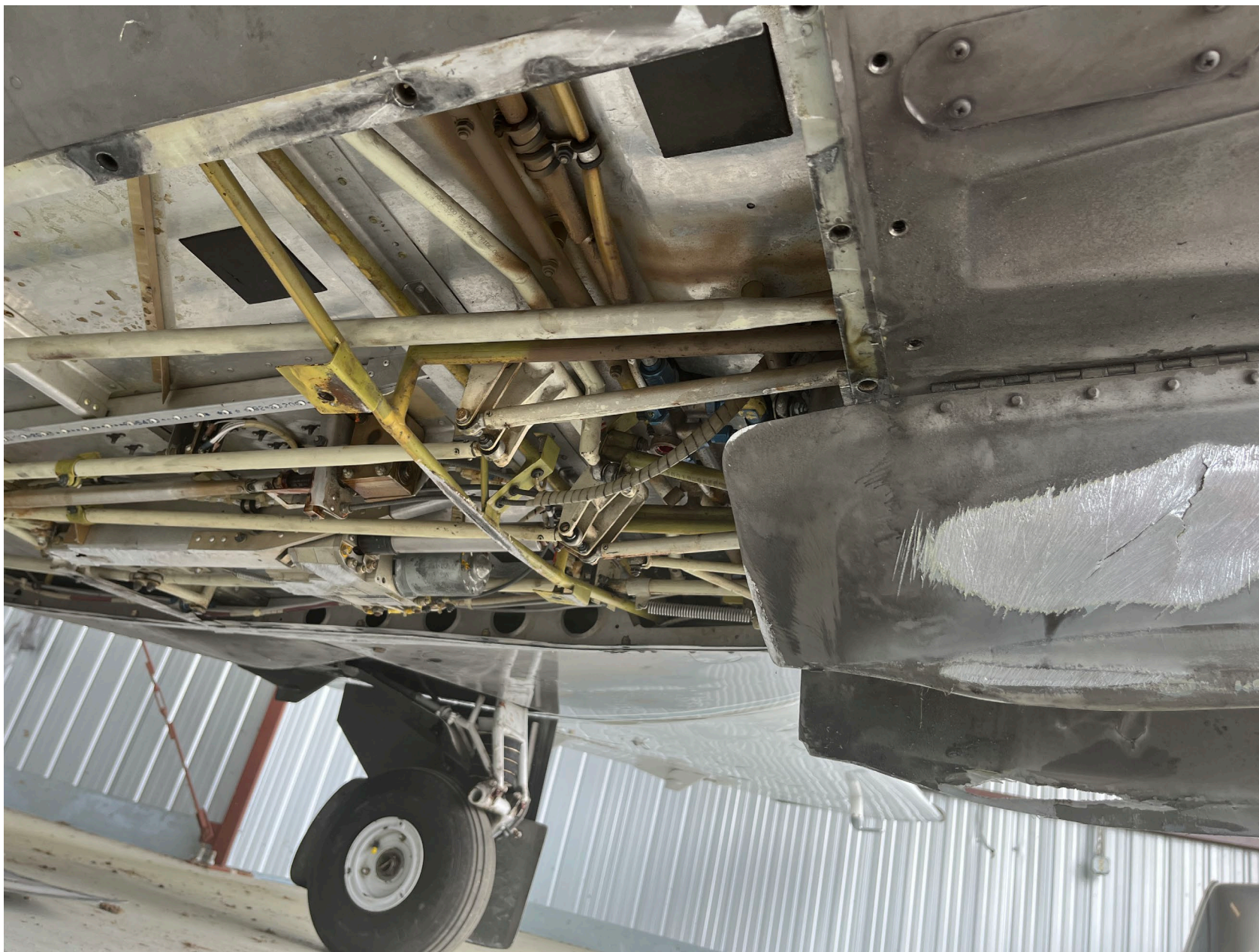
Photo 2 – Photo of Damage to the Truss Skeleton (FAA)
