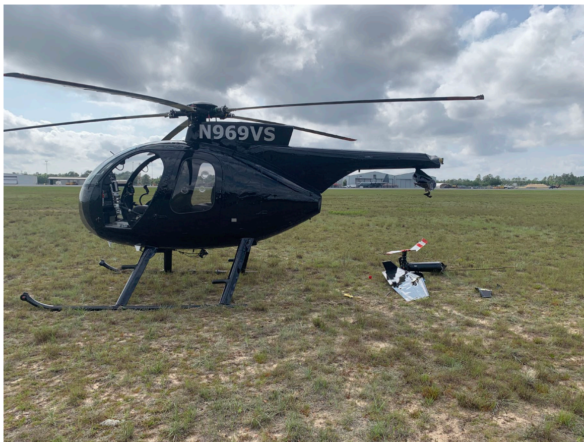
Photograph 2 - Left Side View of Damage (Courtesy of Pilot)
