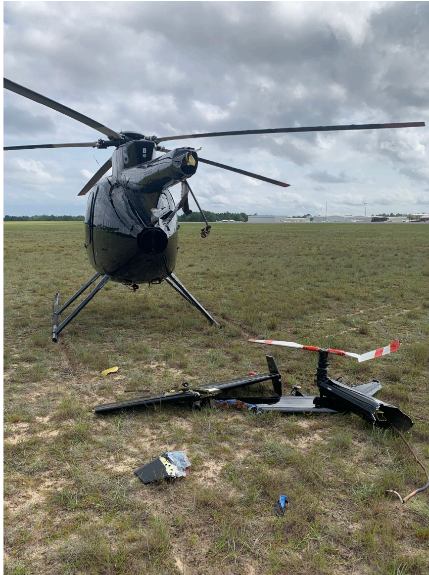
Photograph 1 - Damage to Helicopter Tail (Courtesy of Pilot)
