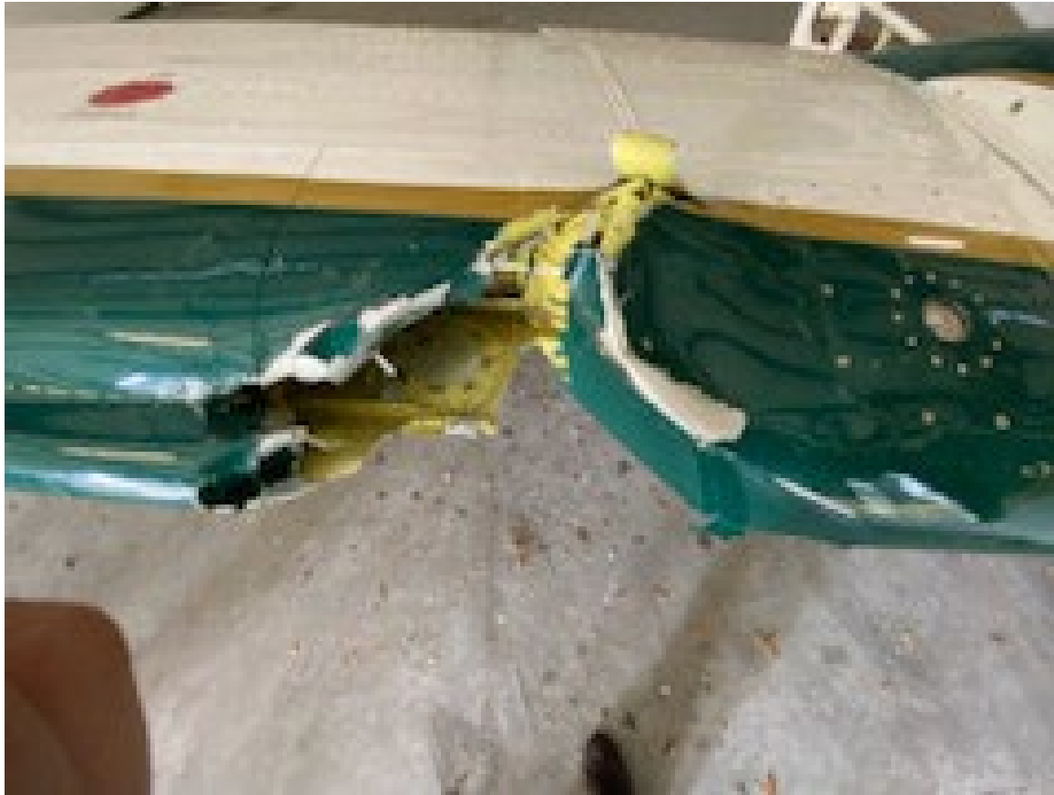
Photograph 2 - Right Wing Damage (Courtesy of FAA)
