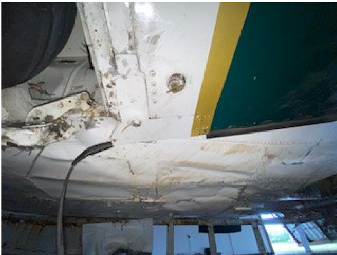
Photograph 4 - Lower Fuselage Damage (Courtesy of FAA)
