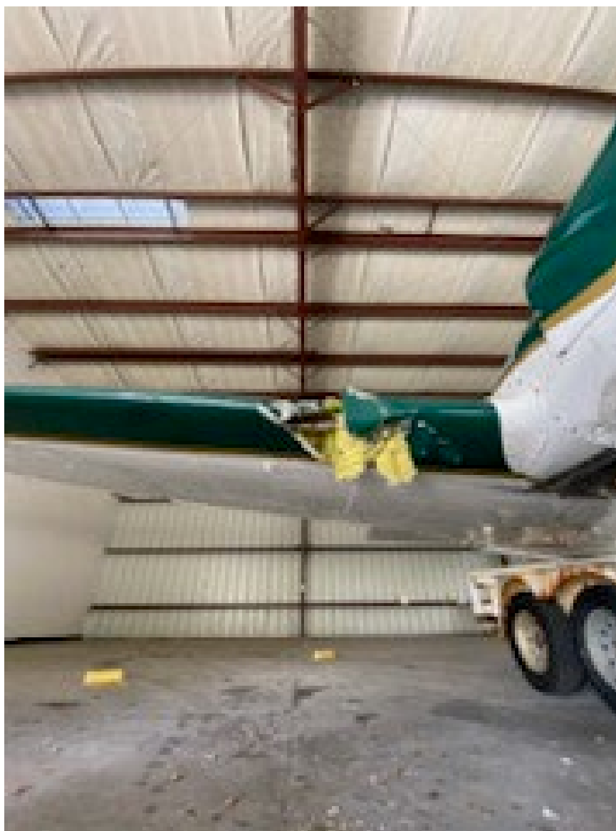
Photograph 3 - Right Wing Damage (Courtesy of FAA)
