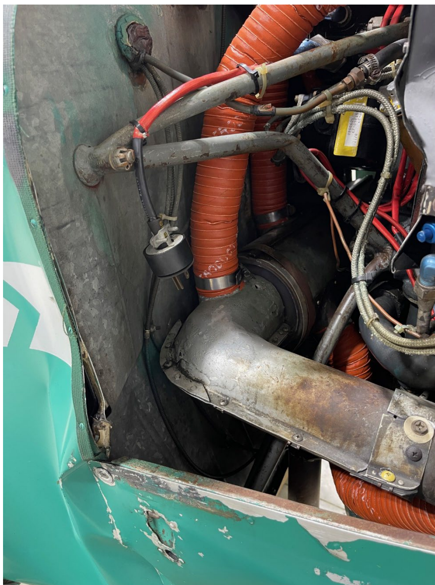
Photograph 3 - Bent engine mount (Courtesy of the pilot)
