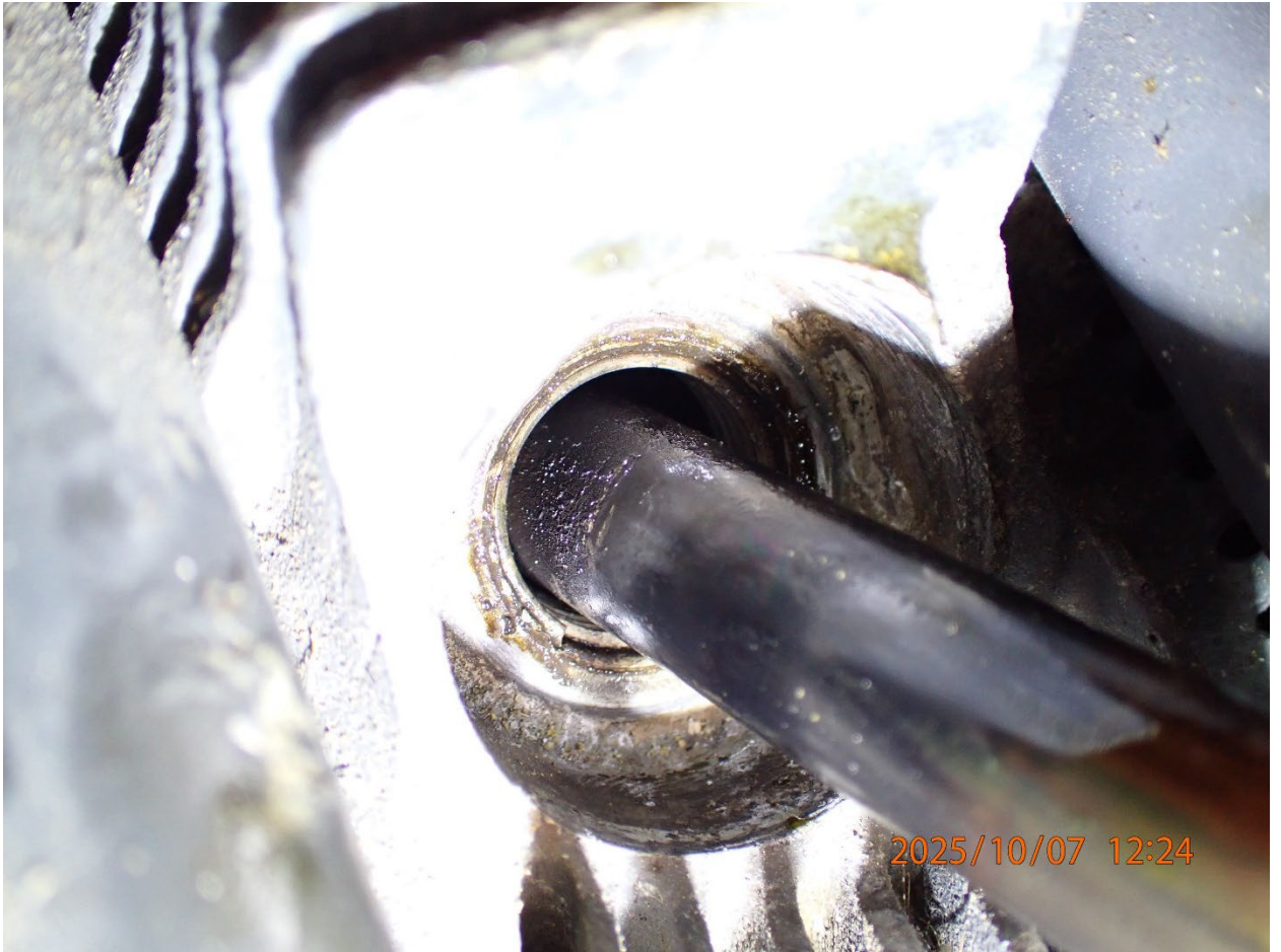
Photo 6: View of the No. 5 exhaust valve stem.
