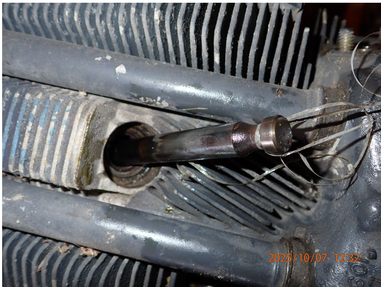
Photo 8: View of the No. 6 exhaust valve stem.
