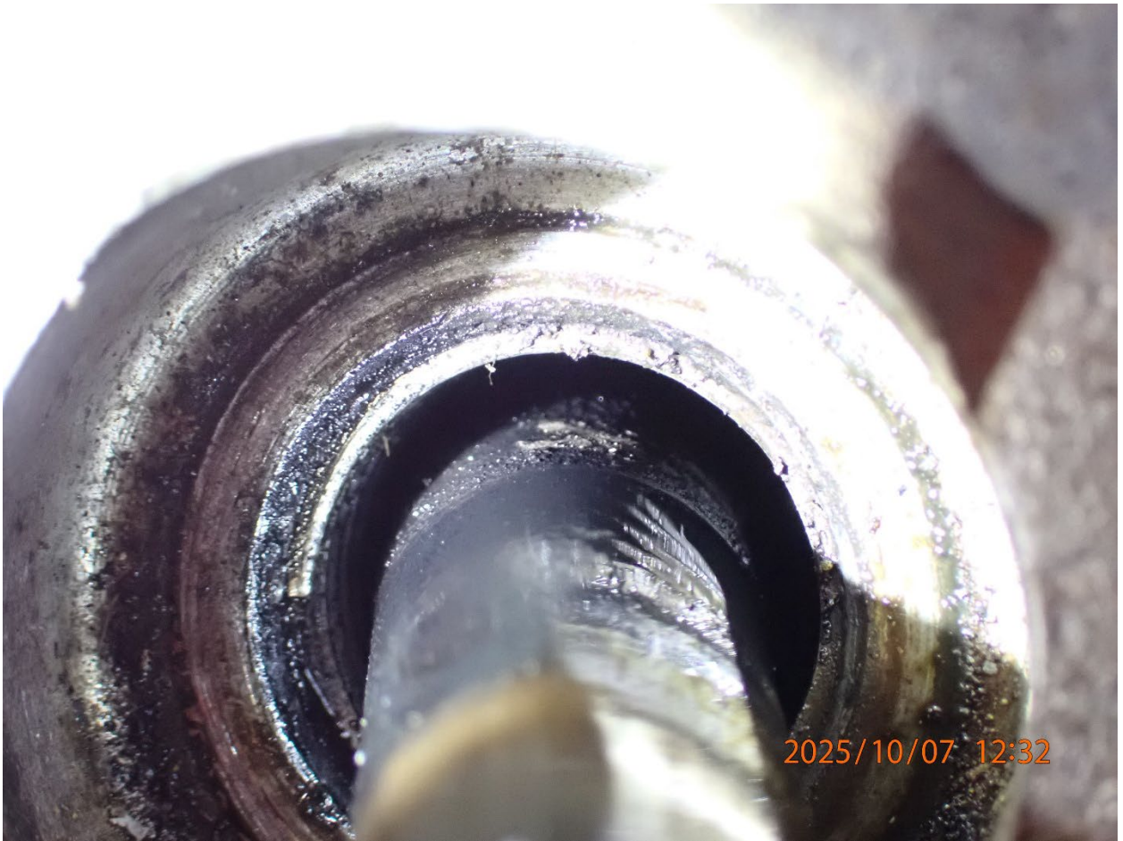
Photo 9: View of the No. 6 exhaust valve stem.
