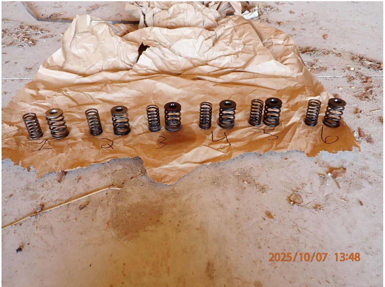
Photo 10: View of the exhaust valve springs.
