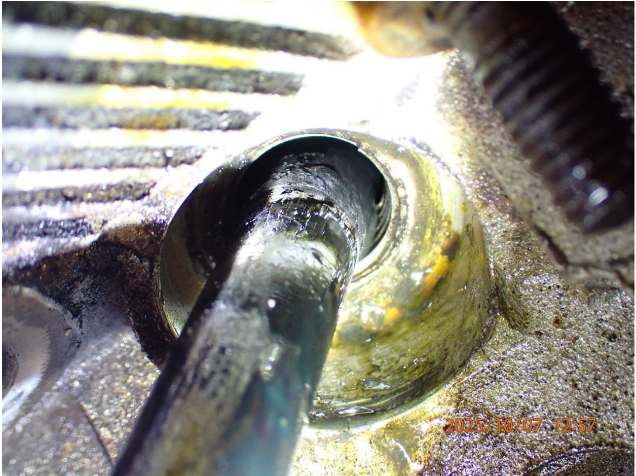
Photo 3: View of the No. 2 exhaust valve stem.
