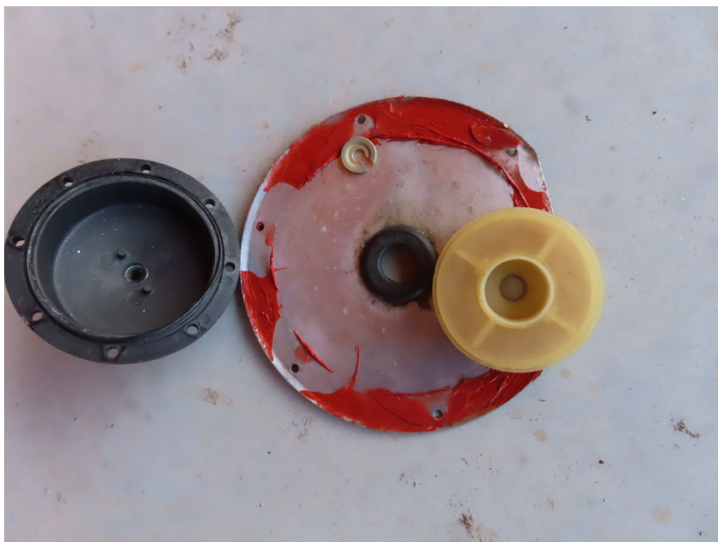
Photo 13: Disassembled fuel strainer. (Piper Photo)
