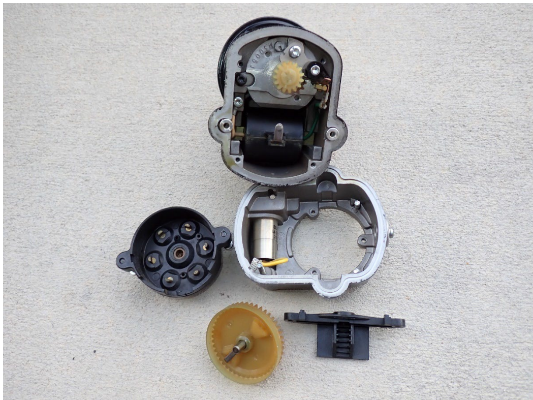
Photo 19: View of the disassembled right magneto.
