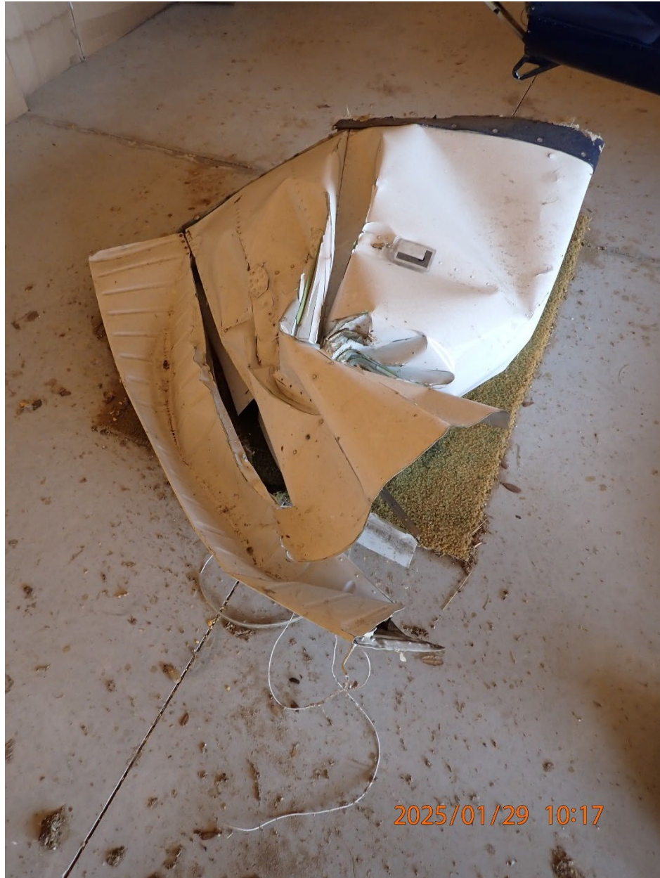
Photo 5: View of the impact separated outboard section of the left wing.
