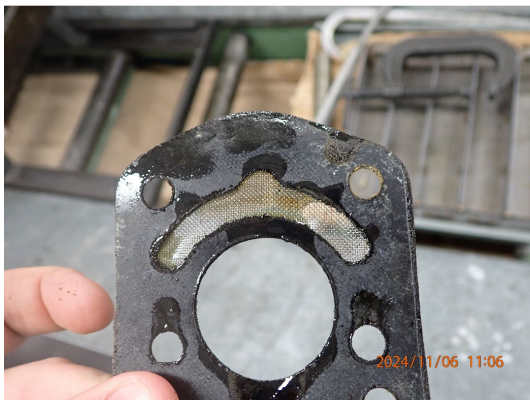
Photo 11: View of the unobstructed propeller governor oil screen.
