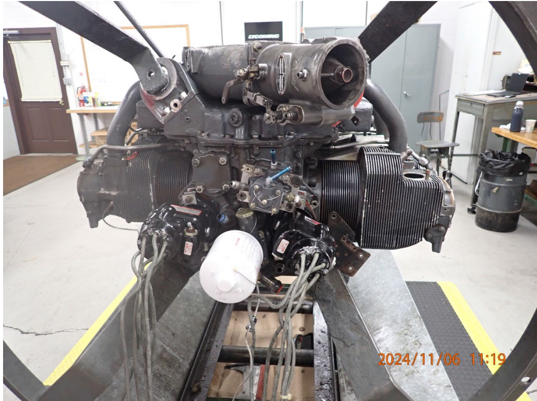
Photo 5: View of the fuel servo and fuel pump installed on the engine.
