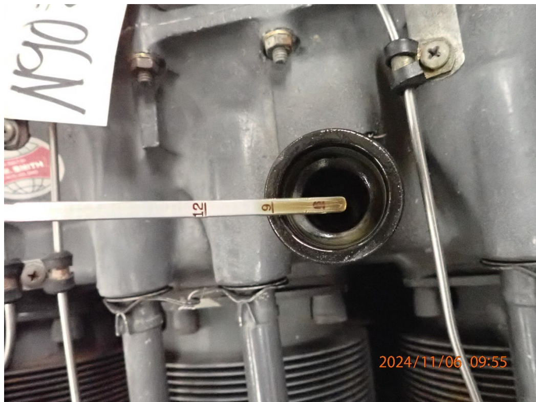
Photo 7: Oil dipstick showing about 9 quarts of oil.
