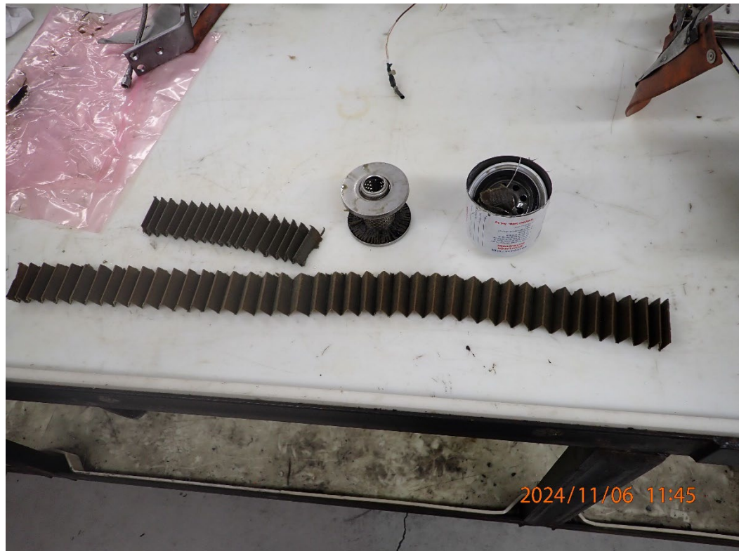
Photo 8: Oil filter removed and cut open.
