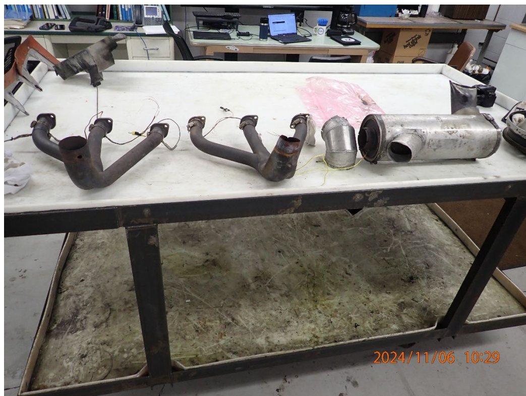
Photo 2: View of the removed exhaust system.
