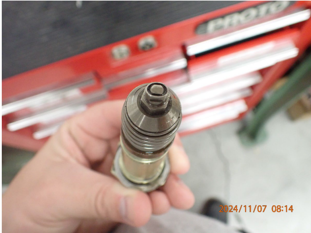
Photo 13: View of the thermostatic oil cooler bypass valve with inconsistent wear.
