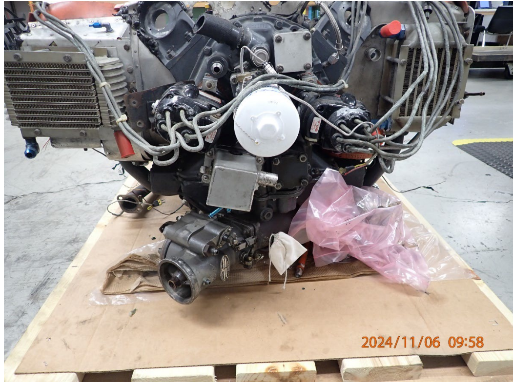
Photo 3: View of the magnetos installed in the accessory case.
