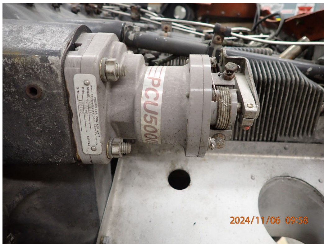
Photo 10: Propeller governor attached to the engine.
