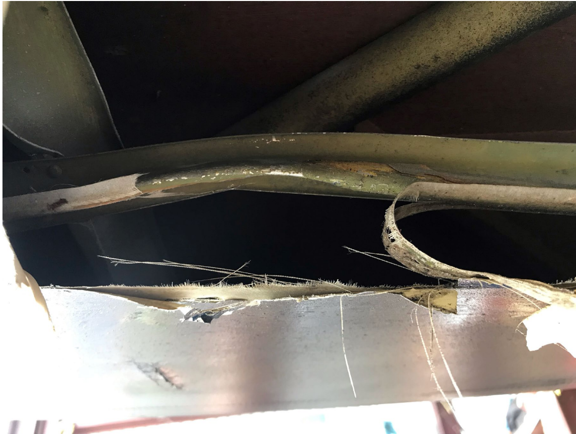
Photograph 3 - Postaccident internal wing damage (Courtesy of FAA)
