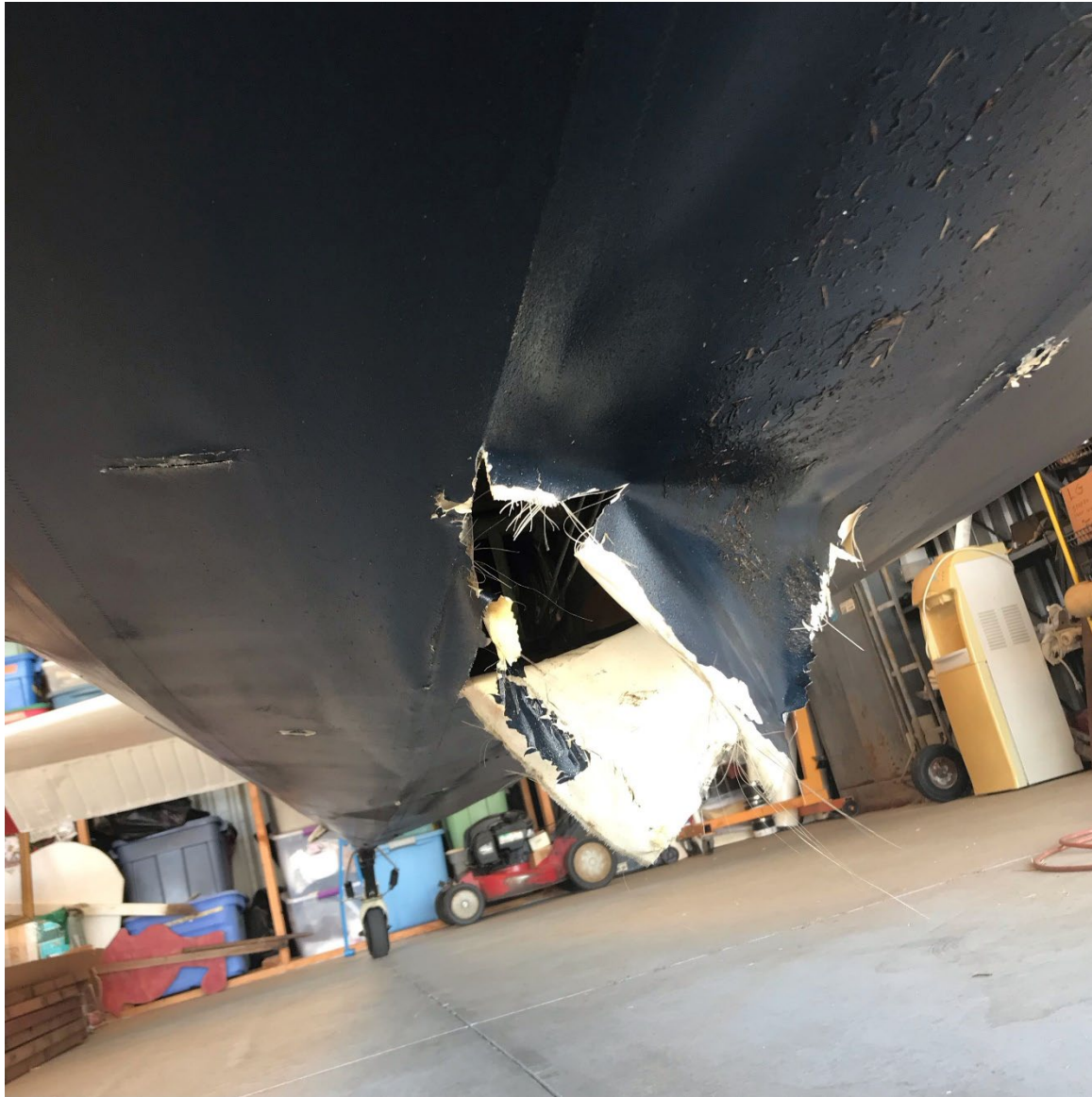
Photograph 2 - Postaccident damage to wing (Courtesy of FAA)
