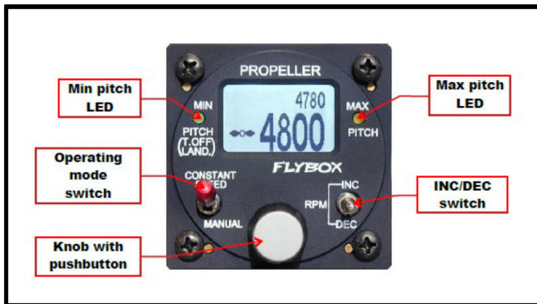
Figure 1: View of PR1-P Propeller Regulator Panel.
