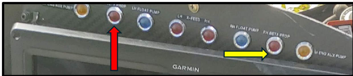
Figure 2: View of the upper central portion of the Instrument Panel showing the annunciator lights. Red arrow points to Left (LH) Beta Prop Annunciator Light while Yellow Arrow Points to Right (RH) Beta Prop Annunciator Light.
