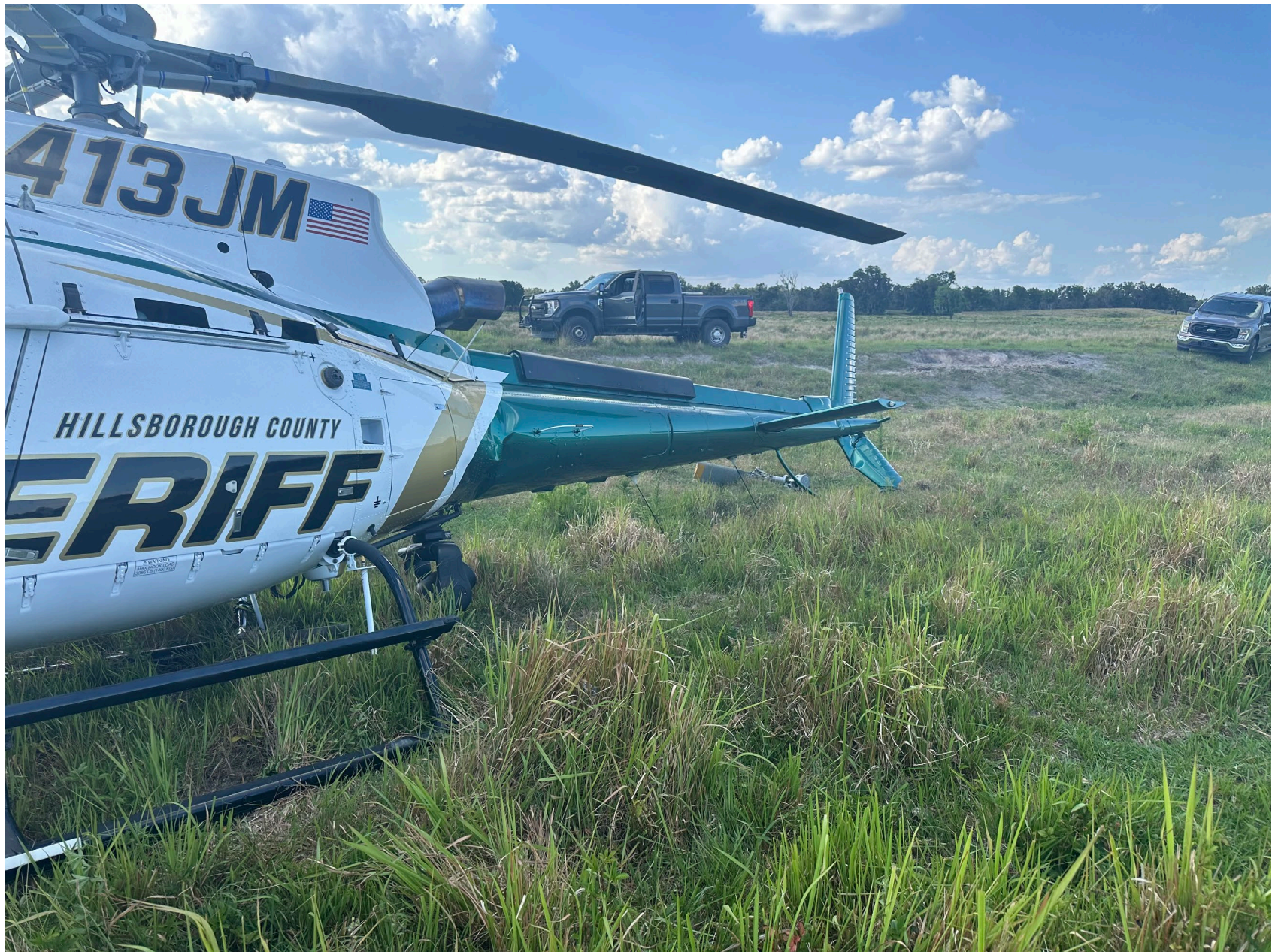
Photo 2 – View of Wrinkled Tailboom, Vertical Stabilizer, and Separated T/R Gearbox (HCSO)
