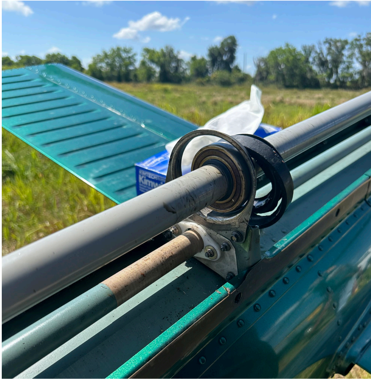
Photo 4 – View of Hanger Bearing Support Bracket with Displaced Elastomeric Bushing (HCSO)
