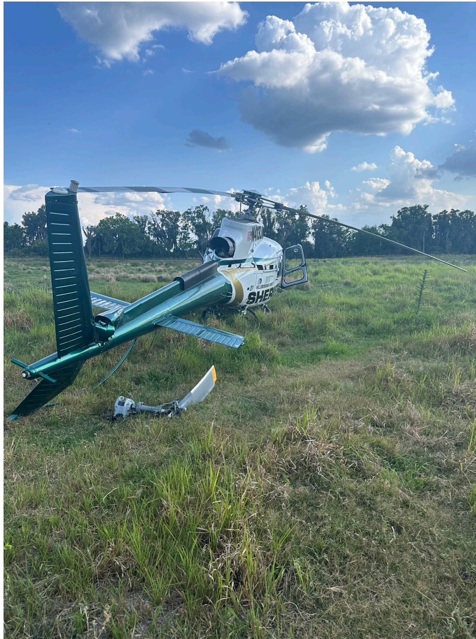
Photo 5 – View of Separated T/R Gearbox (HCSO)
