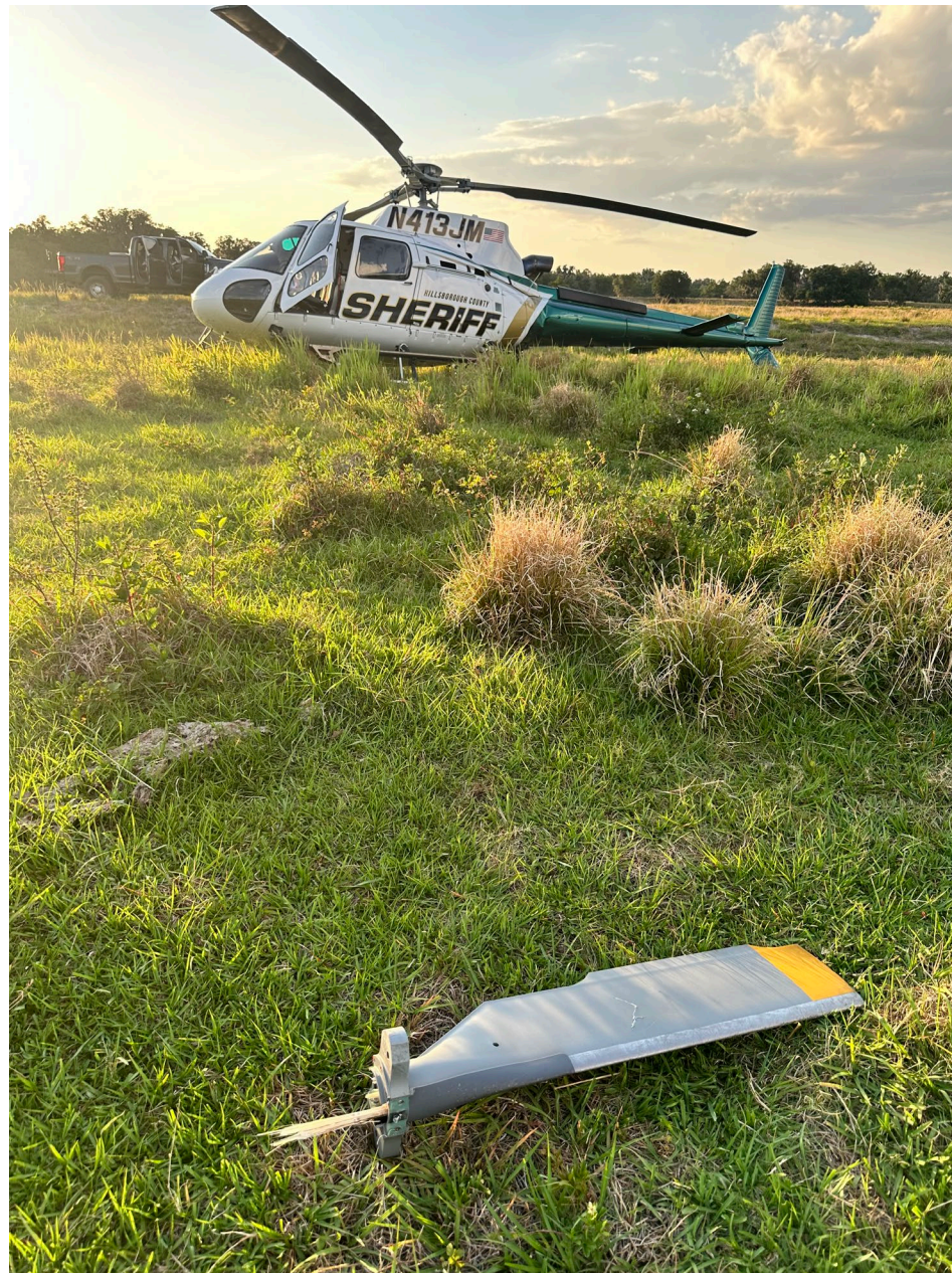
Photo 7 – View of Separated Red T/R Blade as Found (HCSO)
