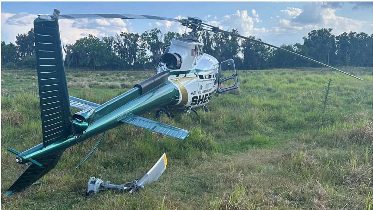
Figure 2. The accident helicopter and the separated tail rotor gearbox.
