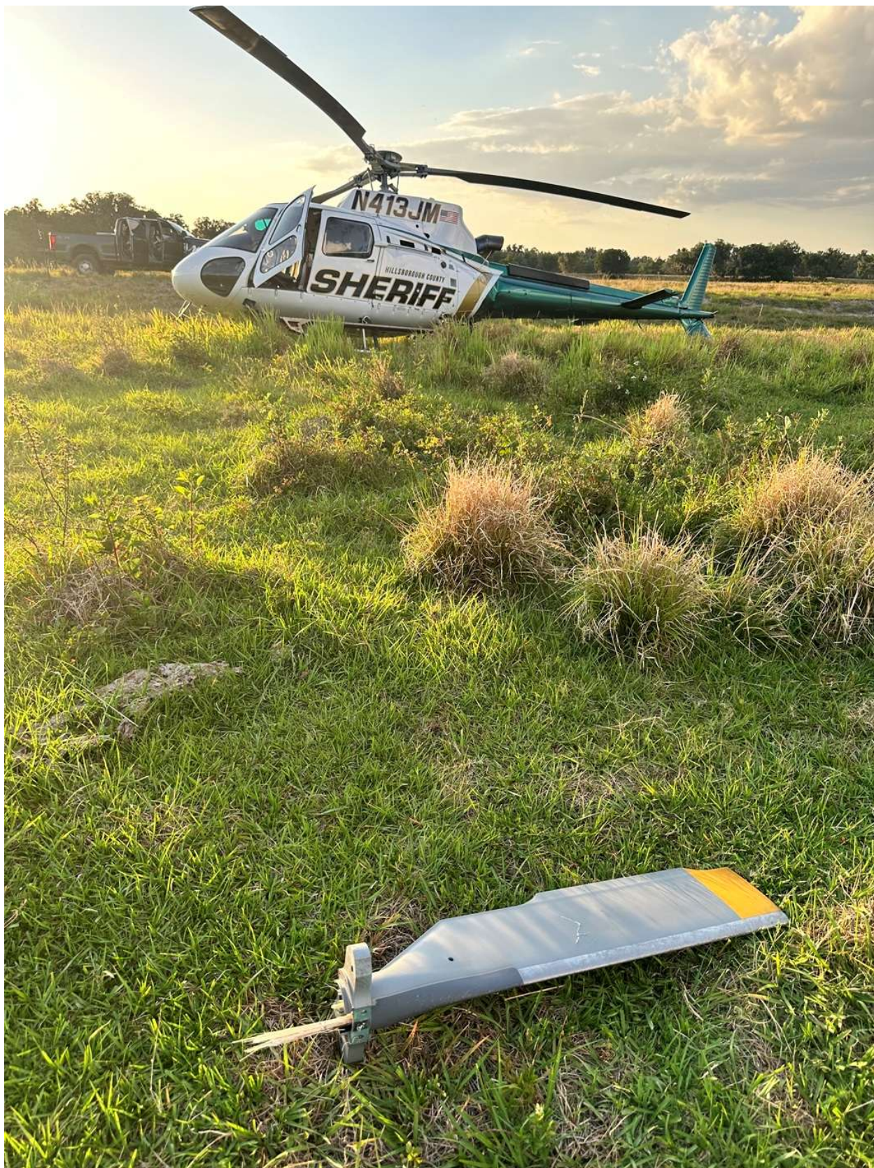
Figure 3. The separated tail rotor blade as found at the accident site.
