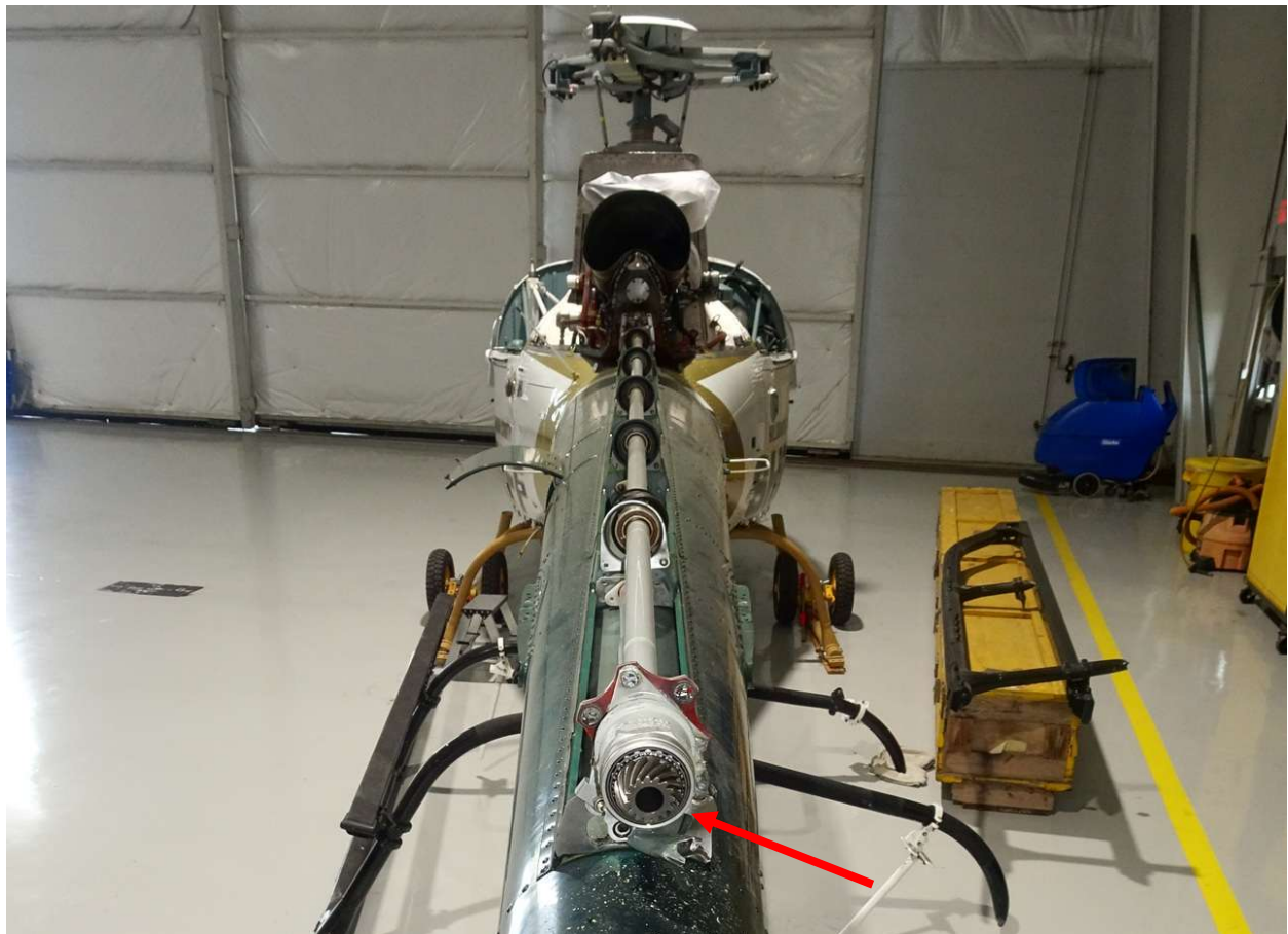
Figure 5. The tail rotor drive system. The red arrow identifies the tail rotor gearbox forward pinion.
