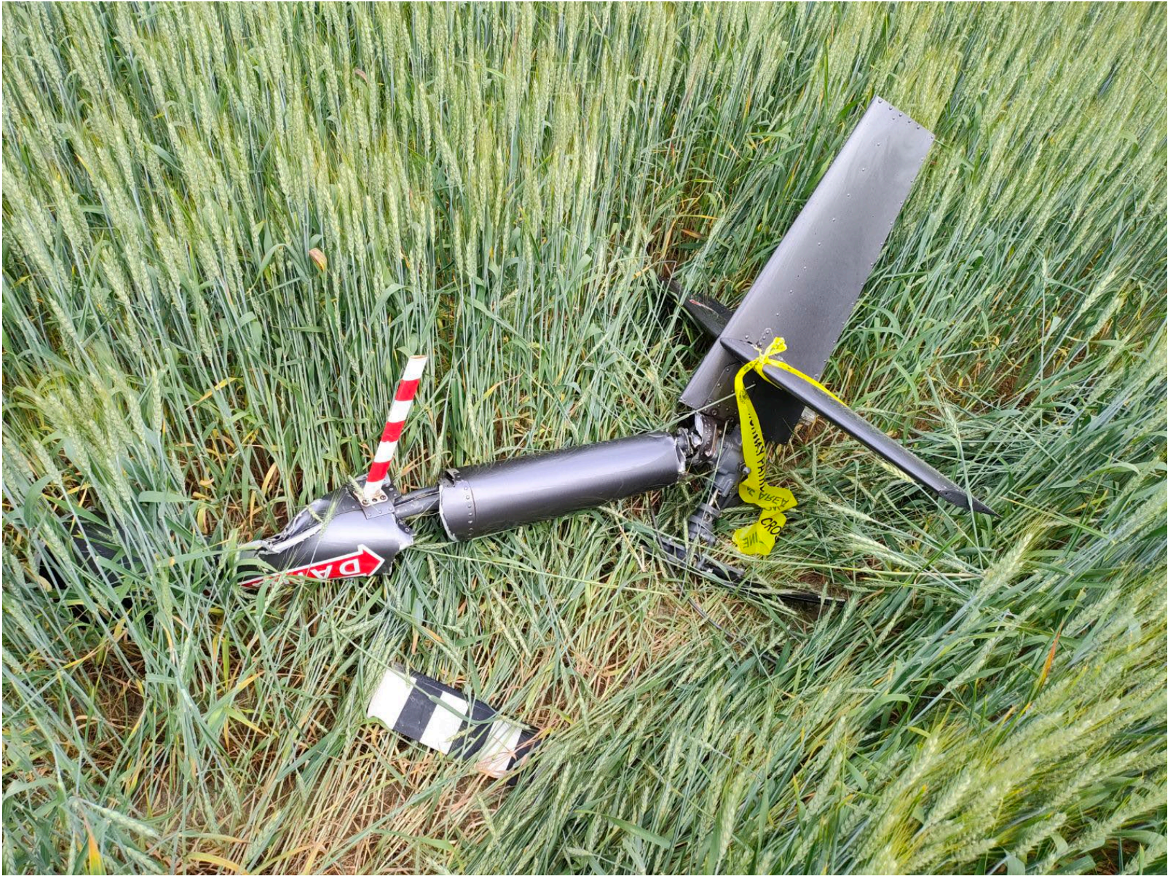
Photo 2 – View of severed tail rotor
