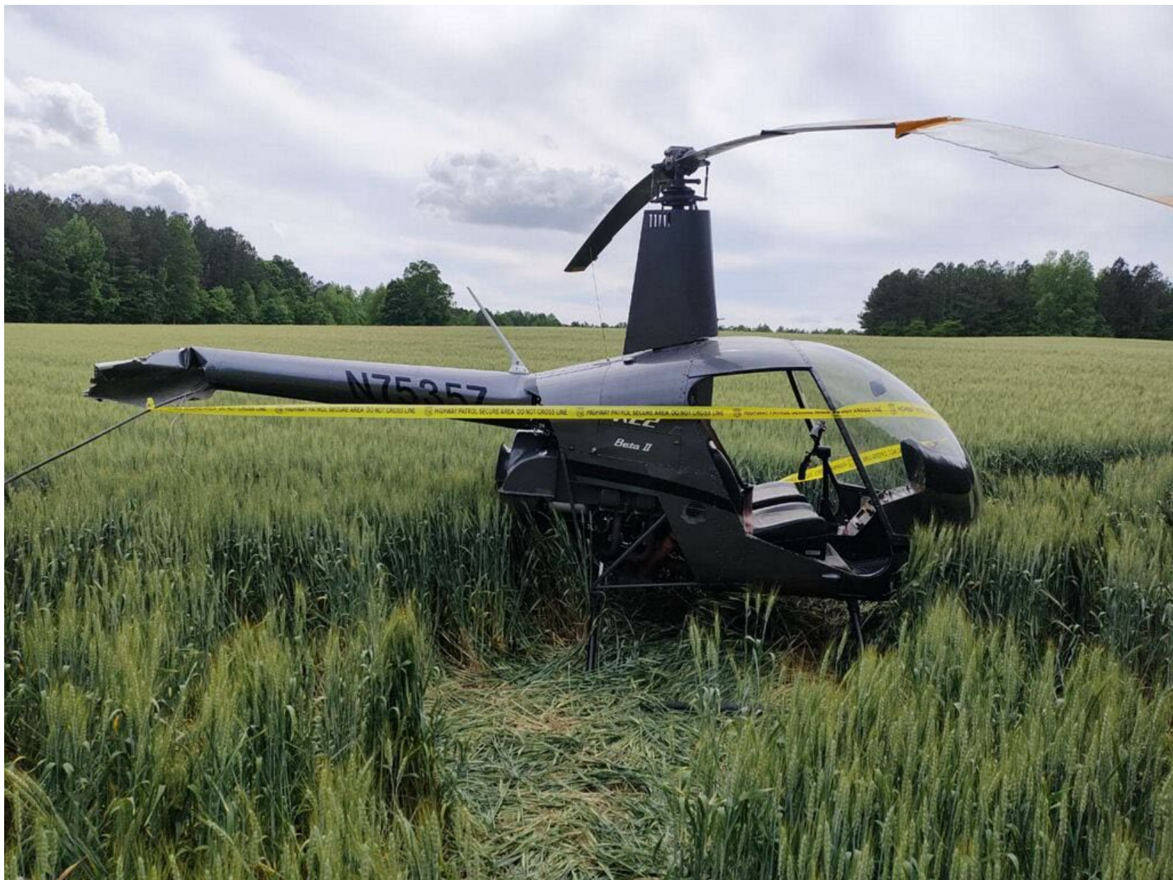
Photo 1 – View of helicopter with severed tail boom
