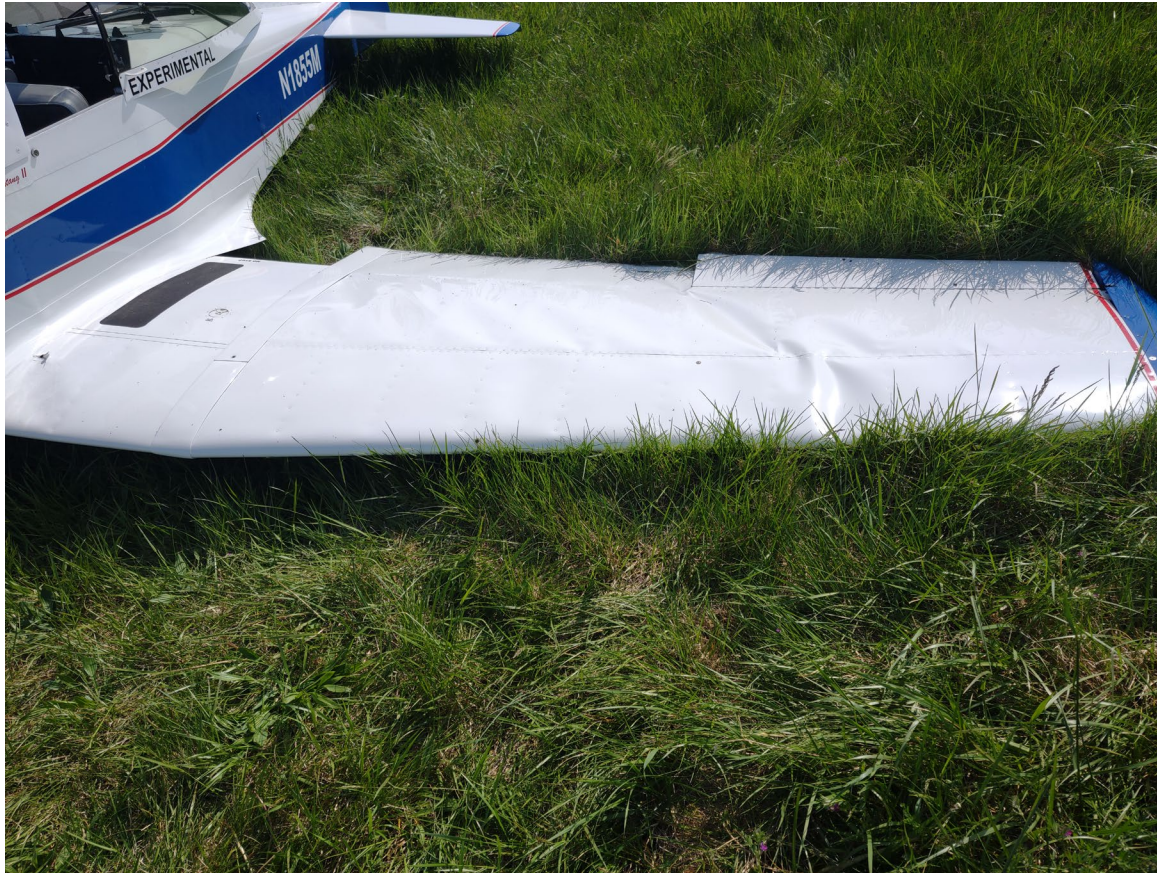
Photograph 2 - Postaccident view of left-wing damage (Courtesy of Pilot)
