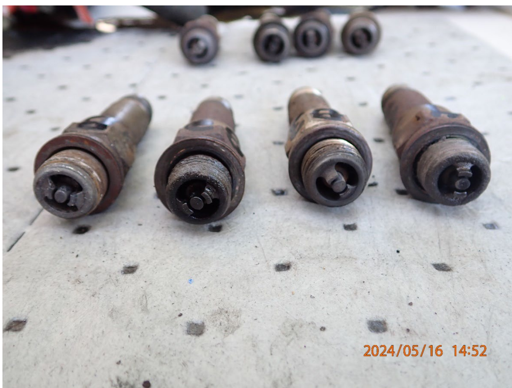
Photo 24: View of the bottom sparkplugs.
