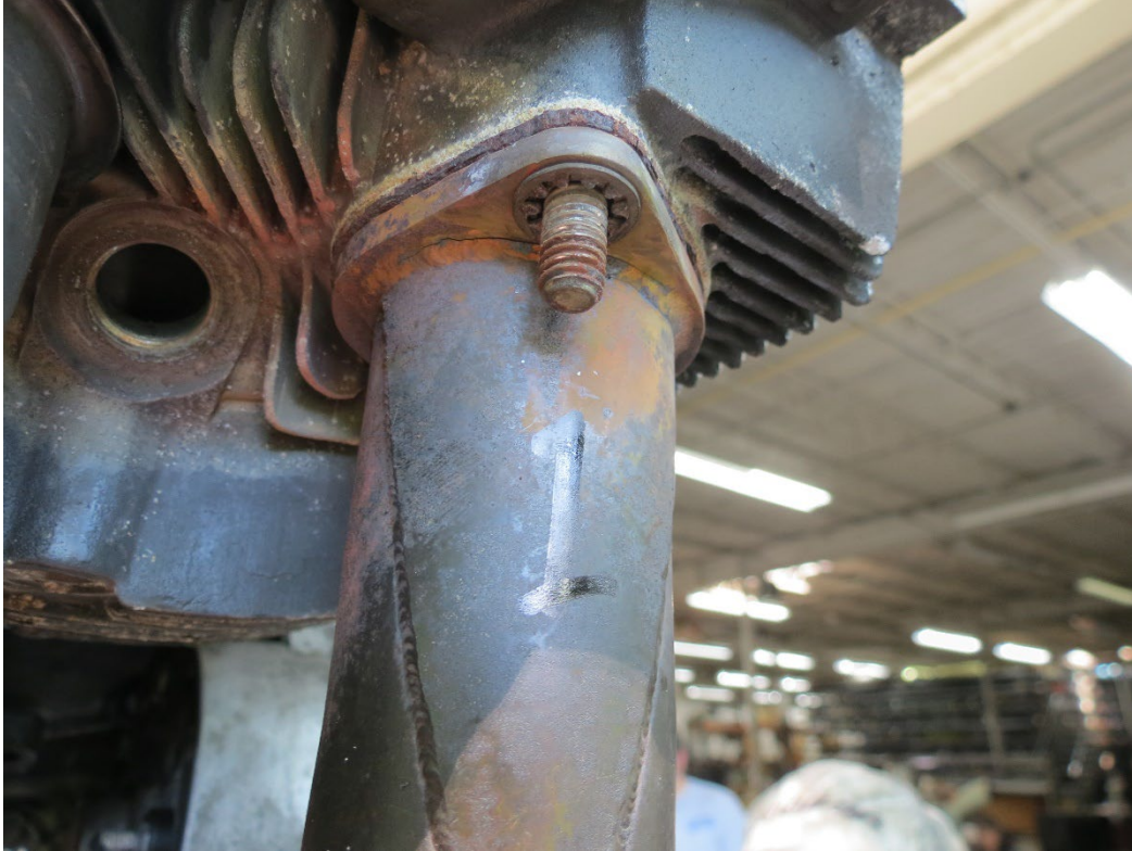
Photo 20: View of the No. 1 exhaust flange. (Lycoming Photo)
