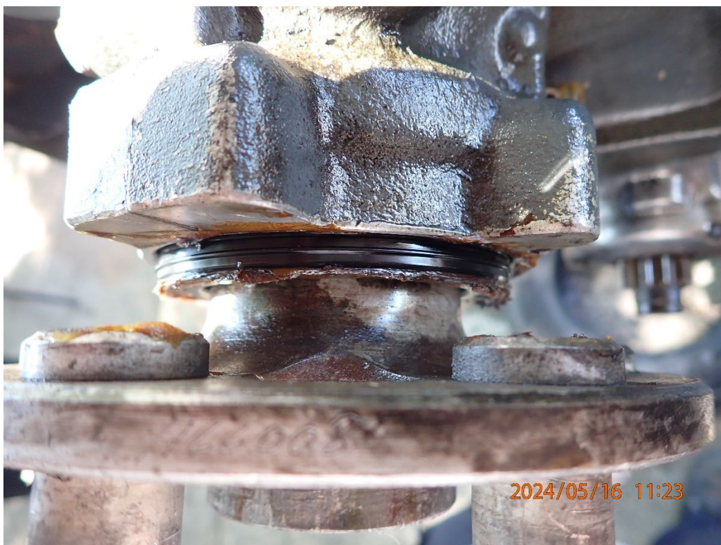
Photo 10: View of the crankcase nose oil seal as first observed.
