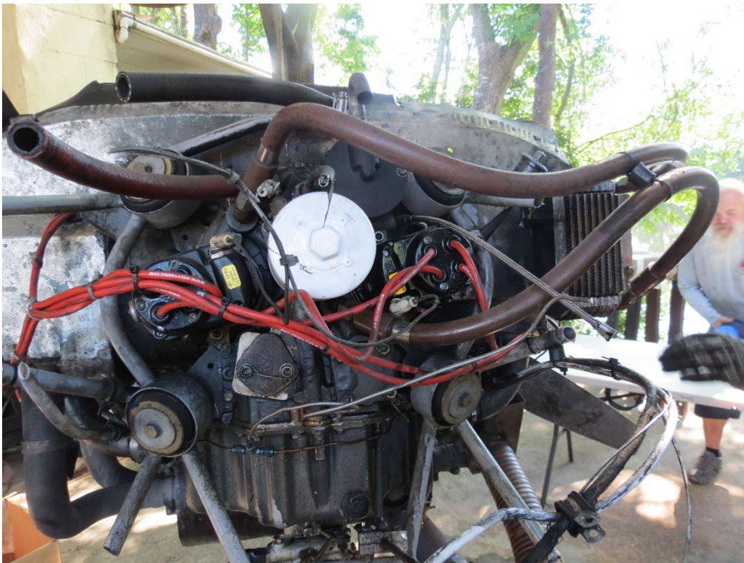
Photo 22: View of the magnetos installed on the engine.
