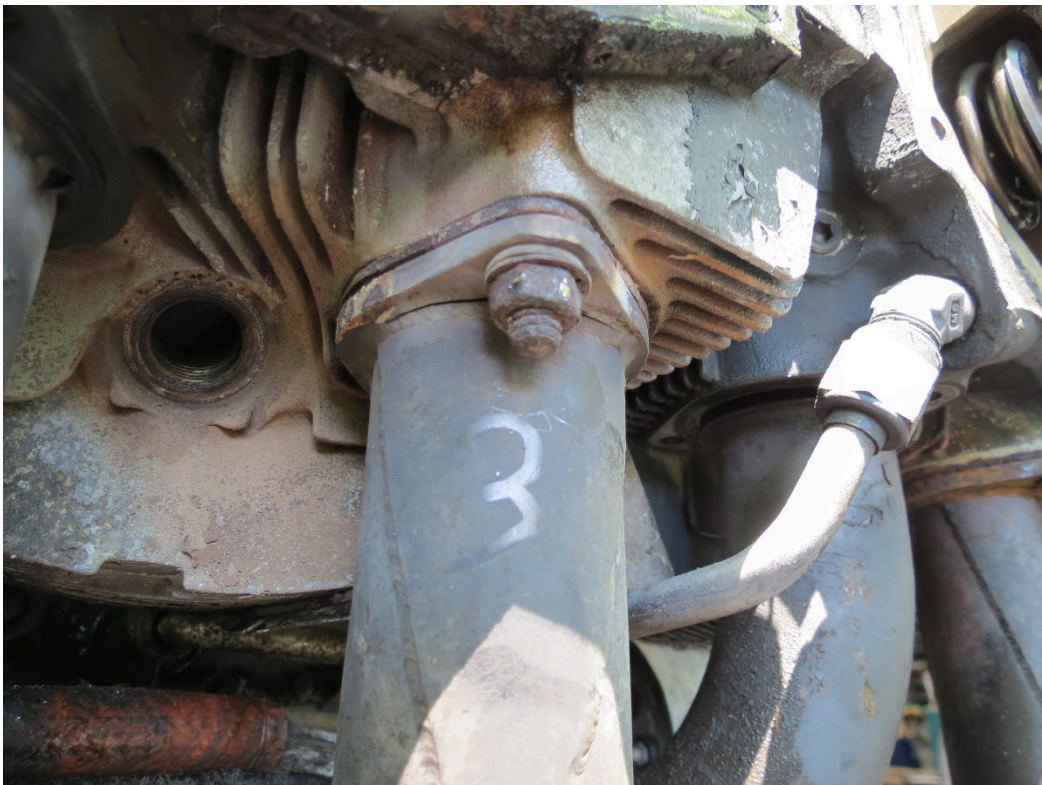
Photo 21: View of the No. 3 exhaust flange. (Lycoming Photo)
