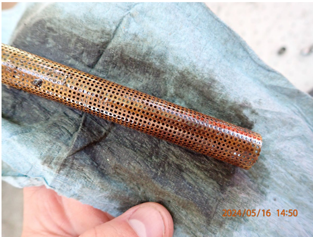
Photo 29: View of the oil suction screen.
