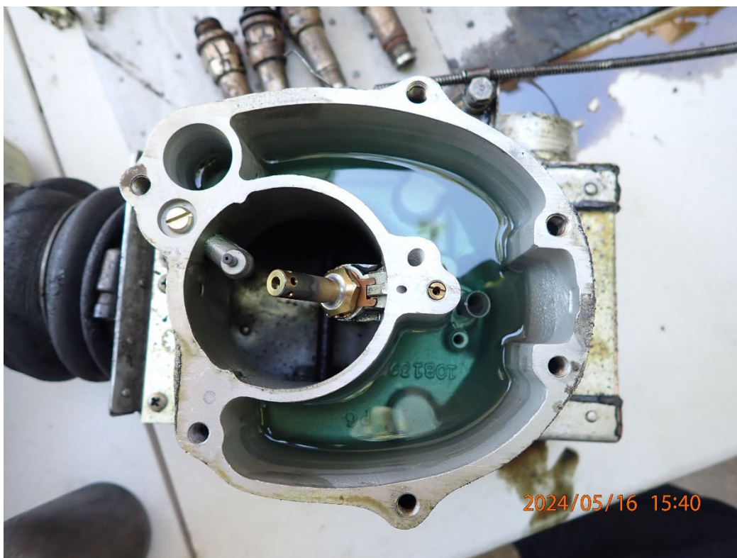
Photo 27: View of fuel in the carburetor float bowl.
