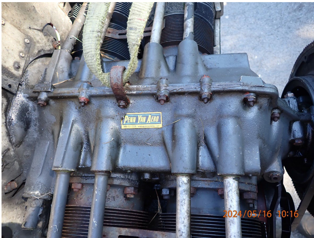
Photo 7: View of sealant on the spine of the crankcase.
