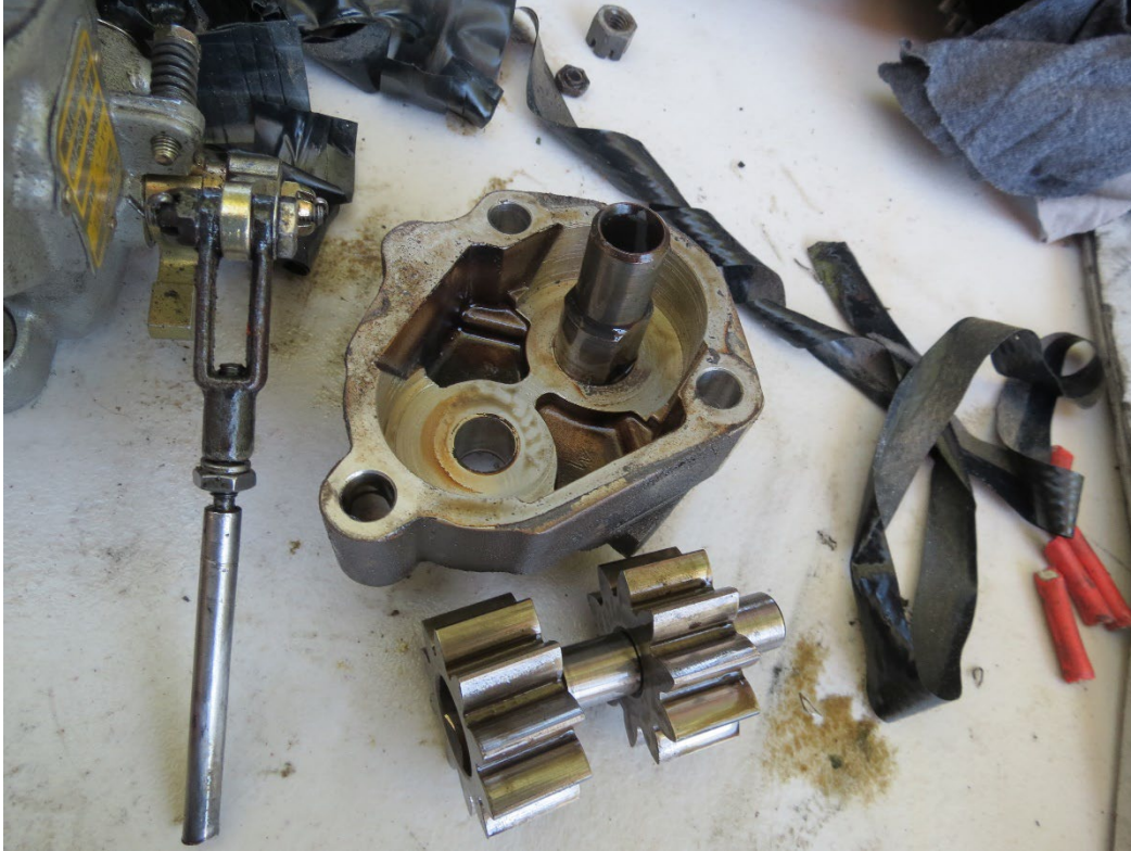
Photo 31: View of the disassembled oil pump. (Lycoming Photo)
