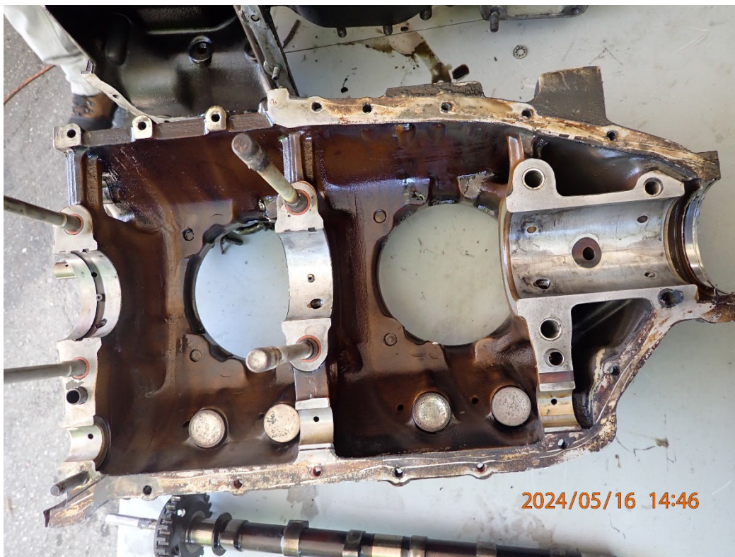
Photo 12: View of the right crankcase half.
