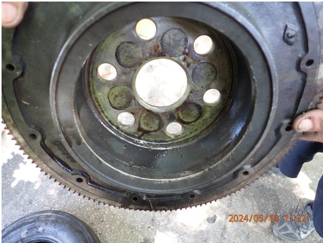
Photo 9: Oil pooled in the back of the starter gear ring.
