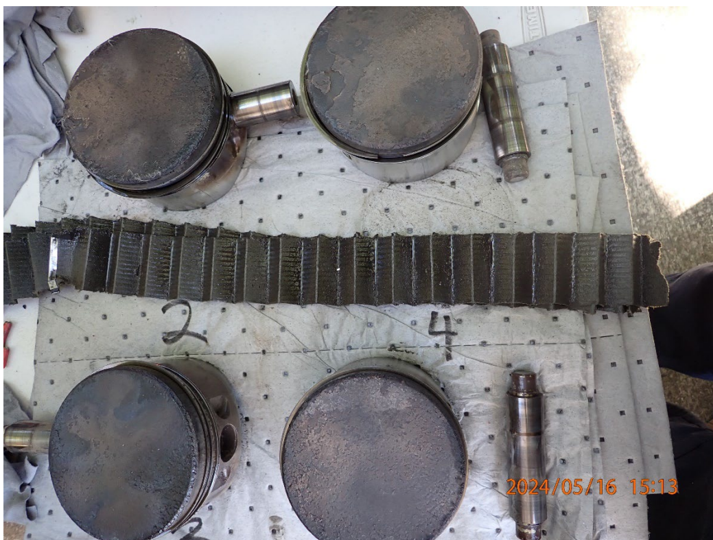
Photo 30: View of the oil filter pleats.
