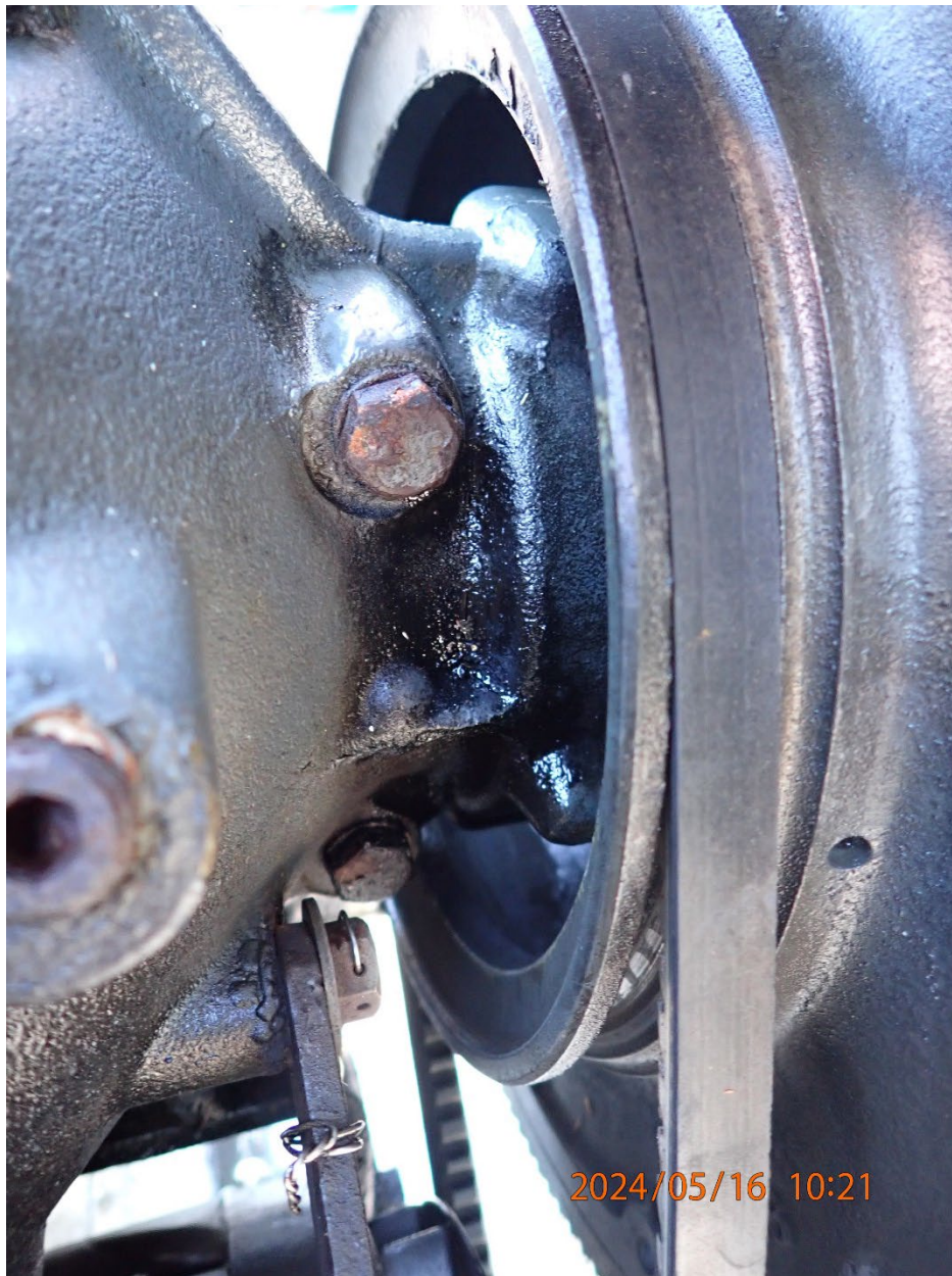
Photo 8: Oil behind the starter ring gear support.
