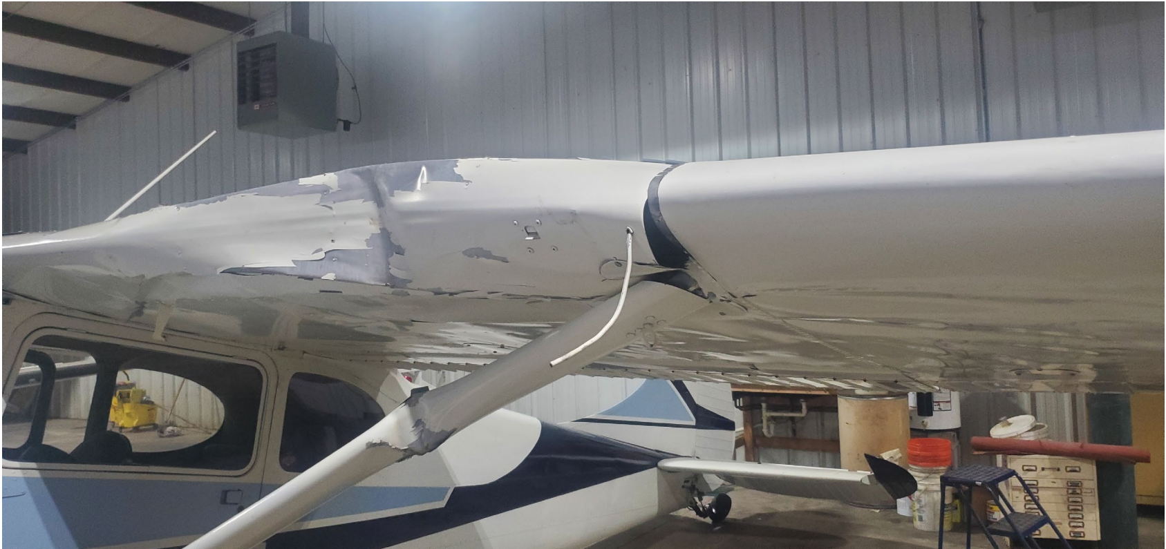
Photograph 5 - Left wing and wing strut damage (Courtesy of FAA)
