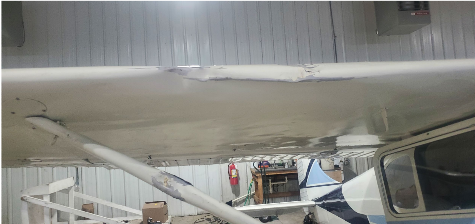
Photograph 4 - Right wing and wing strut damage (Courtesy of FAA)
