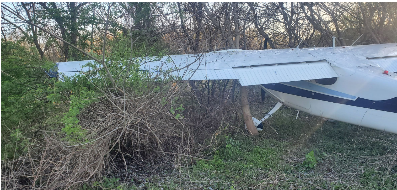
Photograph 2 - Aircraft postaccident. Note left wing damage (Courtesy of FAA)
