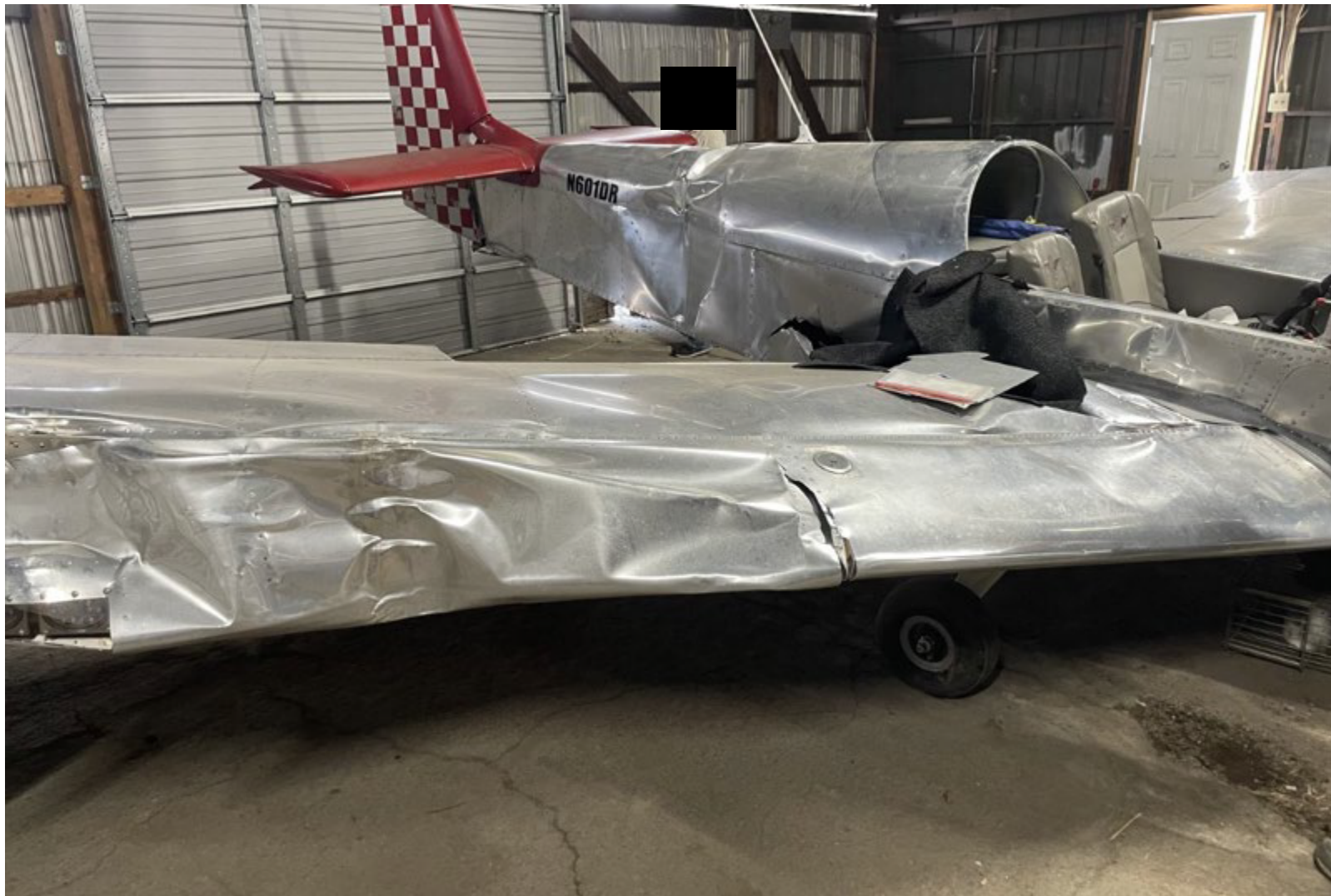
Photograph 1 - Substantial Damage to Right Wing and Fuselage (Courtesy of FAA)
