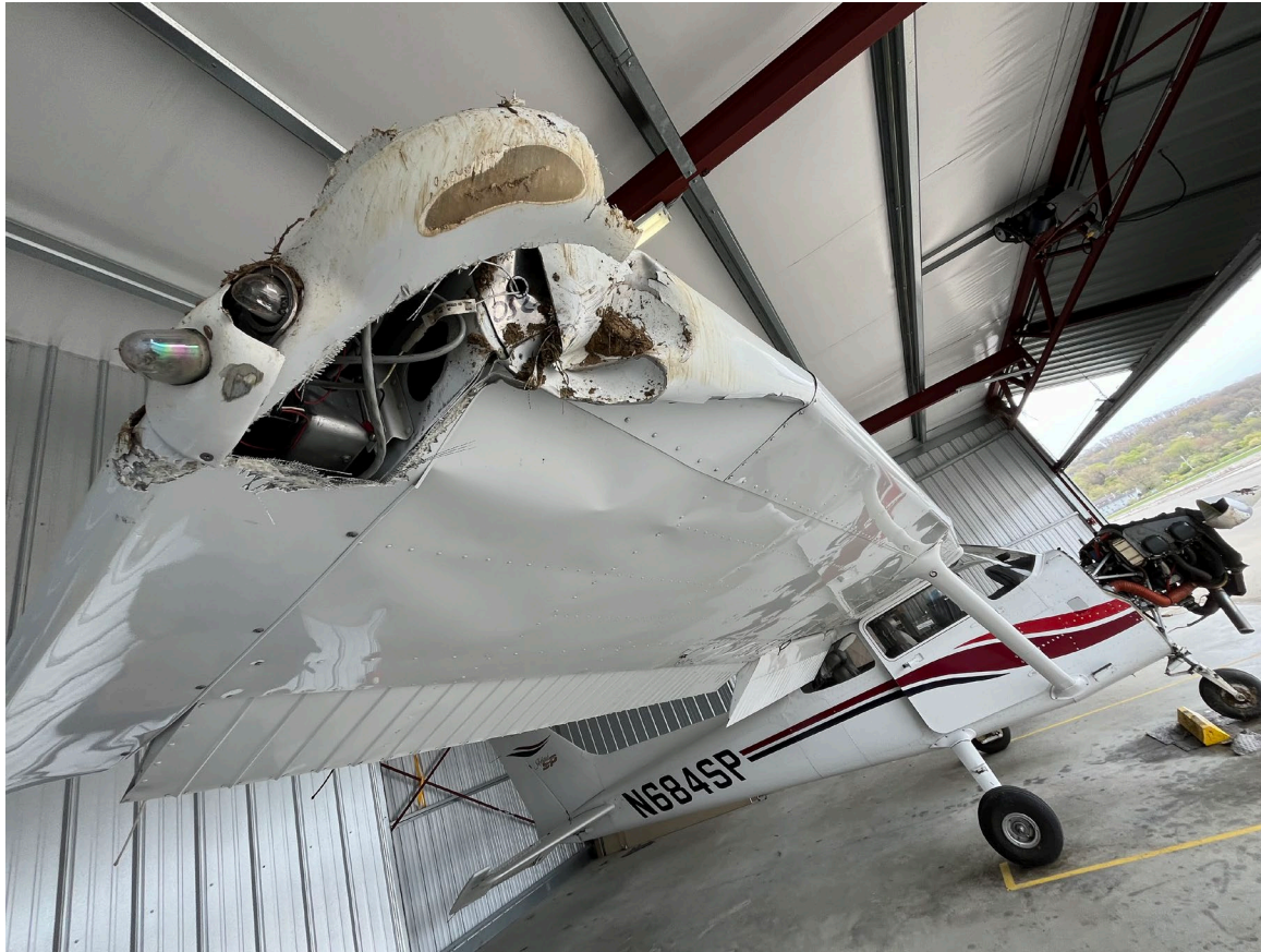
Photograph 2 - FAA Digital Photograph. Right Side View of the Airplane Following Recovery. Note the Damage Aft of the Leading Edge Skin of the Bottom Wing Skin
