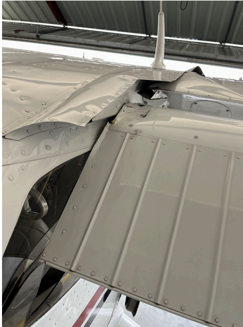
Photograph 3 - FAA Digital Photograph. Aft View of the Inboard Portion of the Right Wing. Note the Buckling of the Upper Skin of the Wing Near the Wing Root
