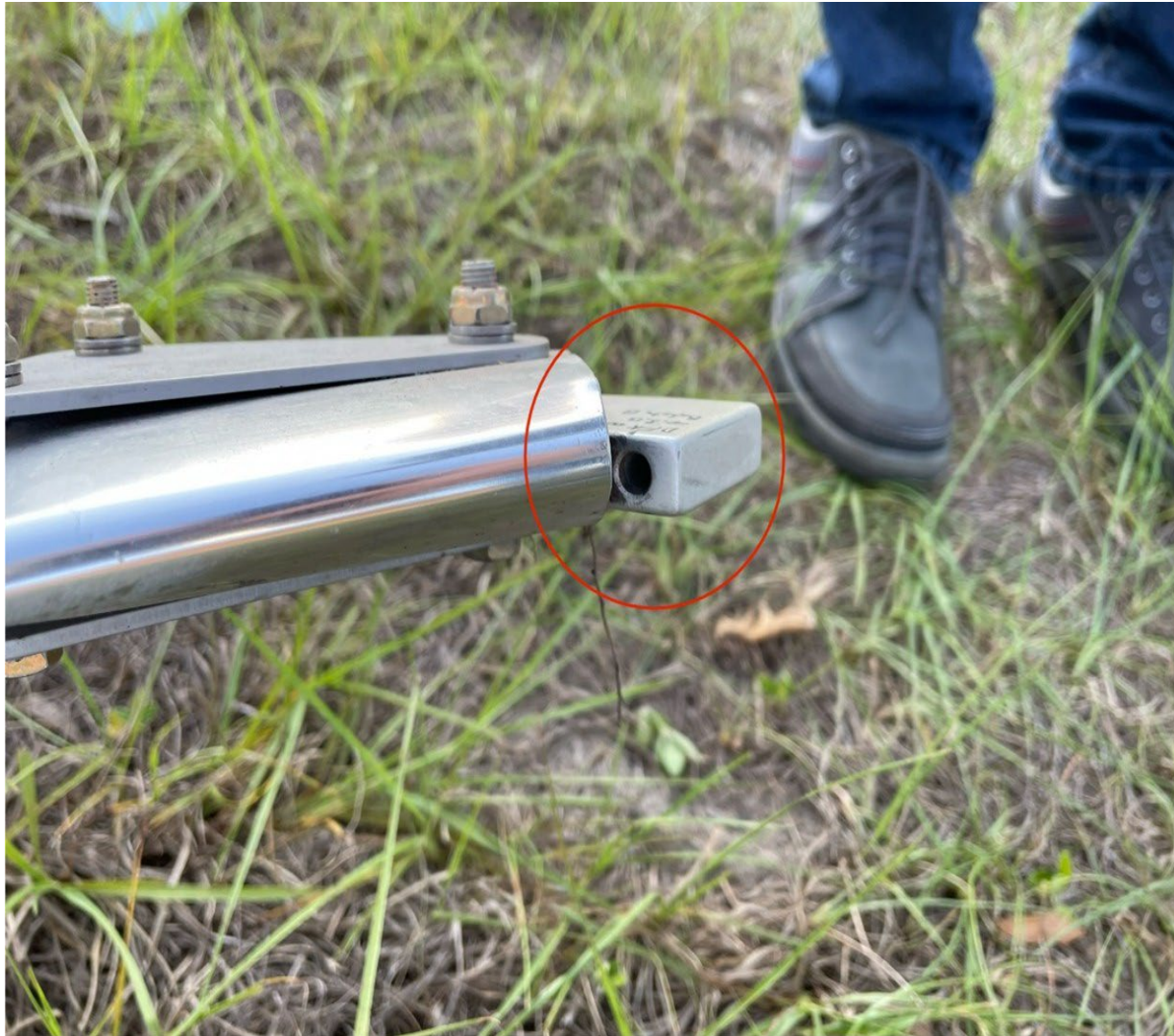
Photograph 3 - Wing Strut connection point (Courtesy of FAA)
