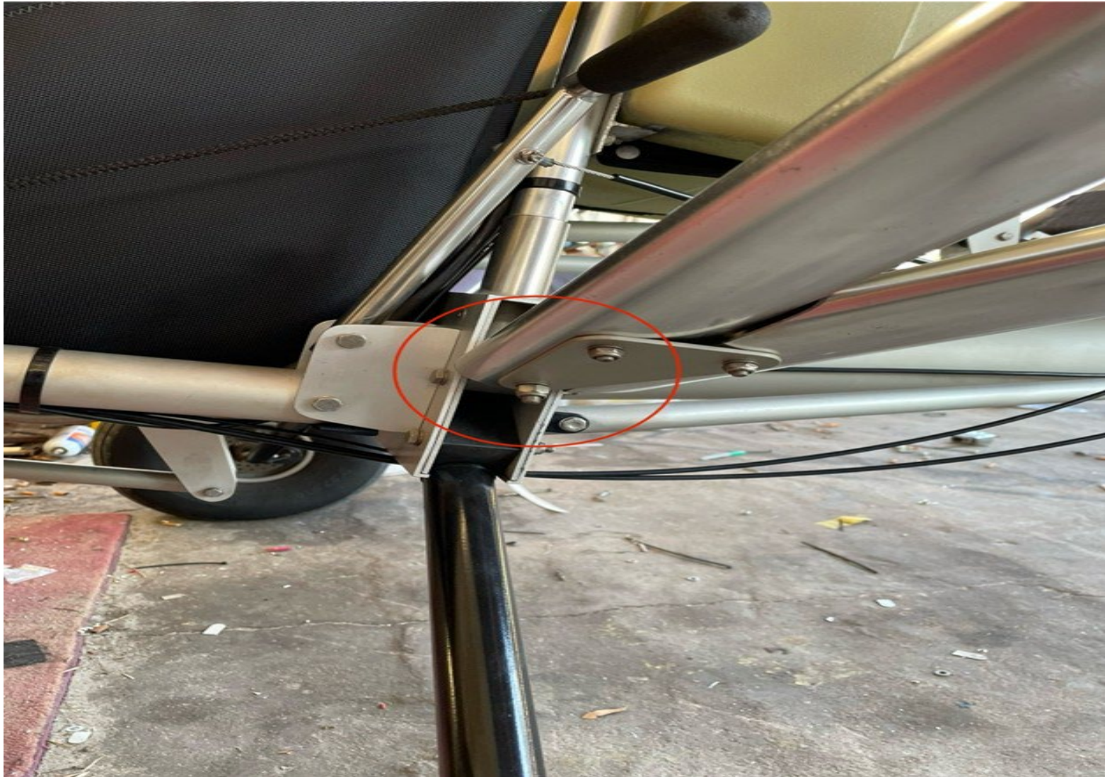
Photograph 7 - Wing connection point properly installed - Non-Accident Aircraft Side 2 (Courtesy of FAA)
