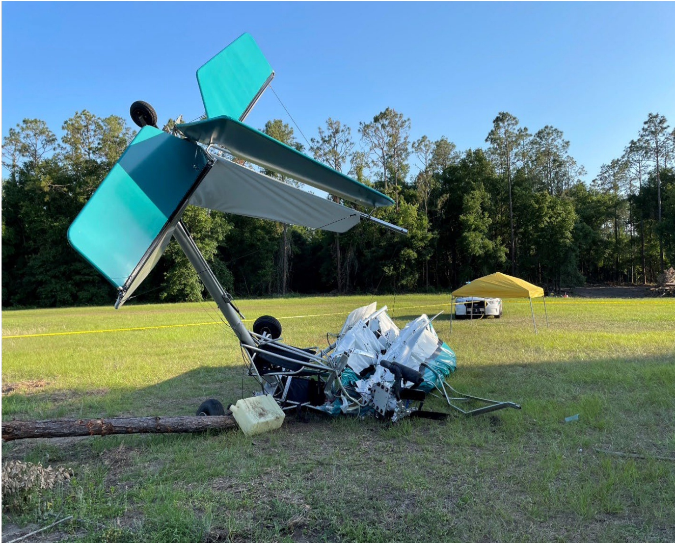
Photograph 2 - View of wreckage facing aft. (Courtesy of FAA)
