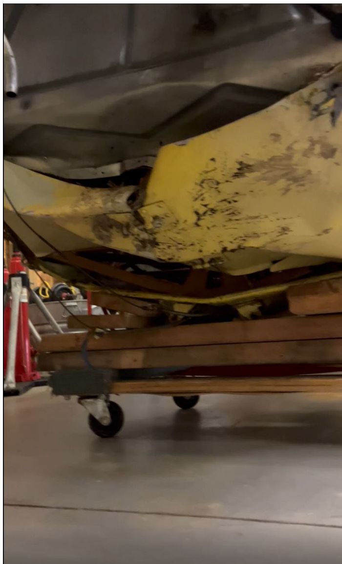
Photograph 4 - Fuselage damage (Courtesy of pilot)
