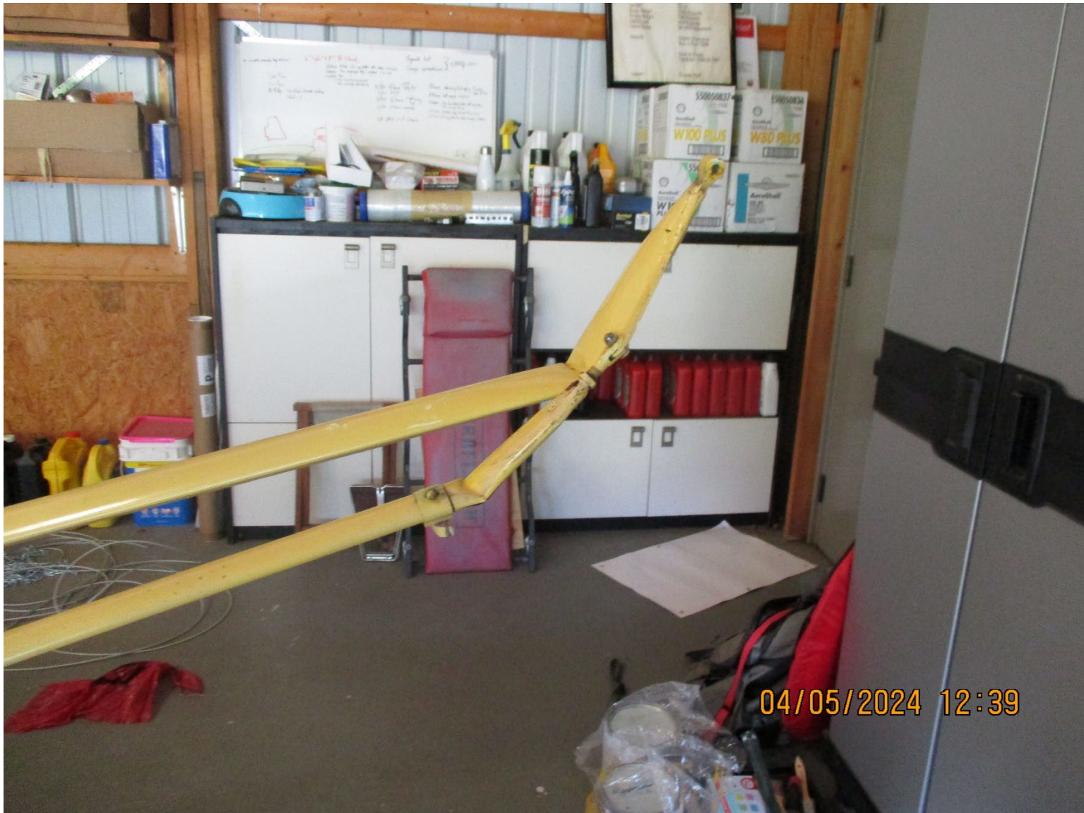
Photograph 3 - Bent wing strut (Courtesy of FAA)
