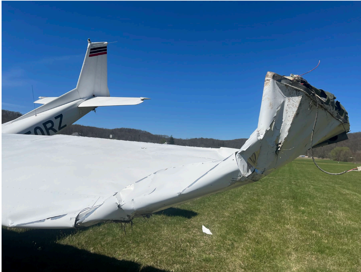
Photograph 3 - Left Wing Damage (Courtesy of FAA)
