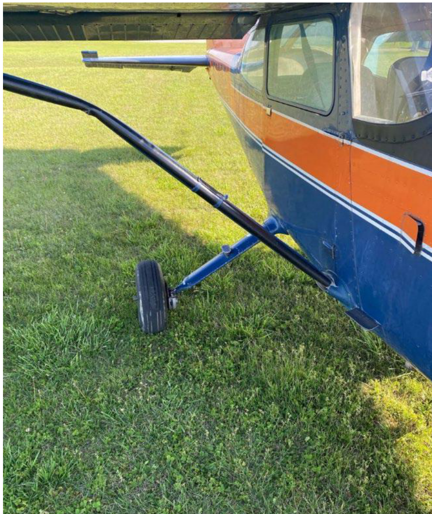
Photograph 3 - View of right wing strut damage. (Courtesy of FAA)
