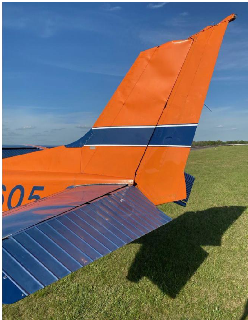
Photograph 2 - View of damaged vertical stabilizer. (Courtesy of FAA)
