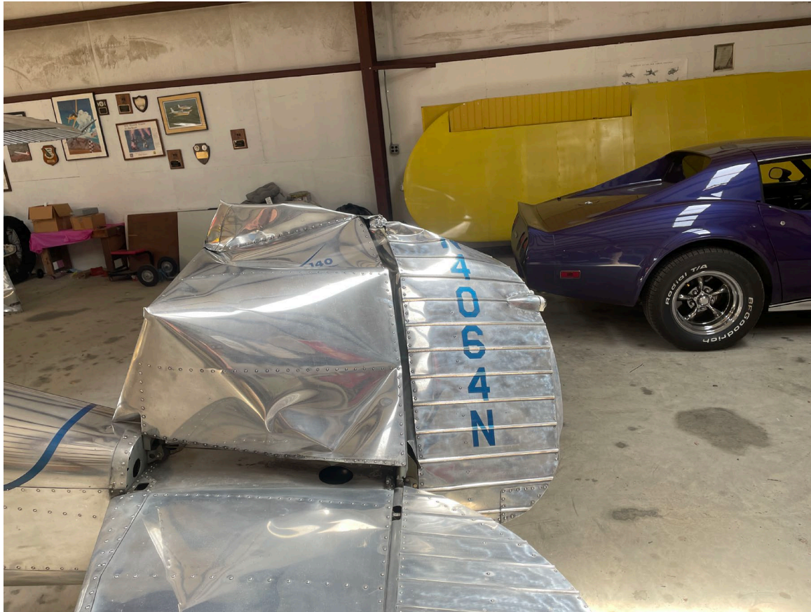
Photograph 2 - Empennage Damage (Courtesy of FAA)
