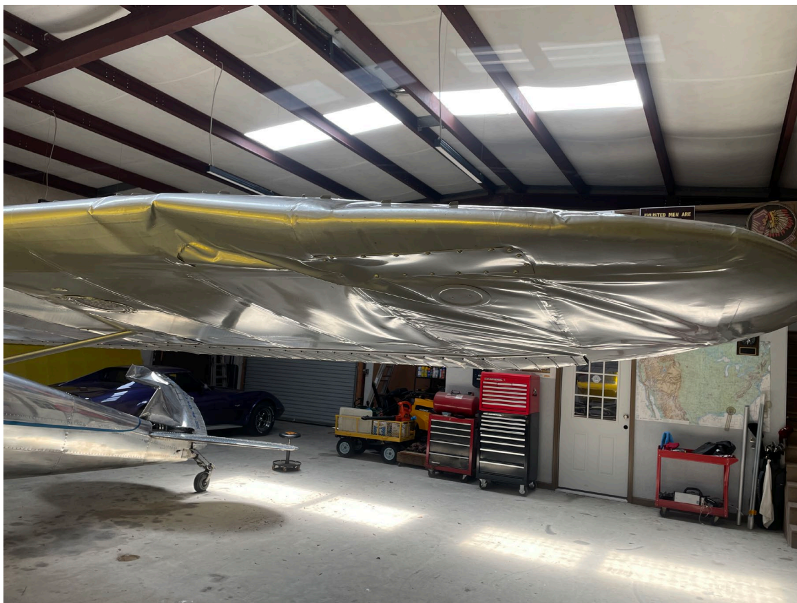
Photograph 3 - Left Wing Damage (Courtesy of FAA)
