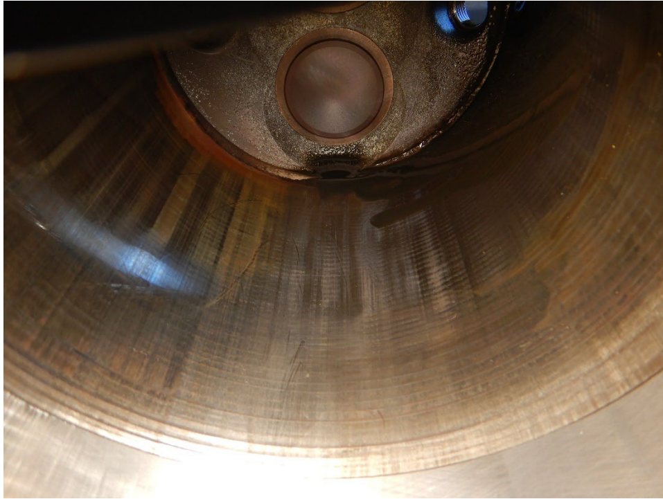
Photo 25 - Interior of cylinder No. 3 after removal of cylinder from engine.
