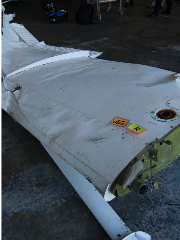
Photo 6 - View of right wing root with missing fuel cap.
