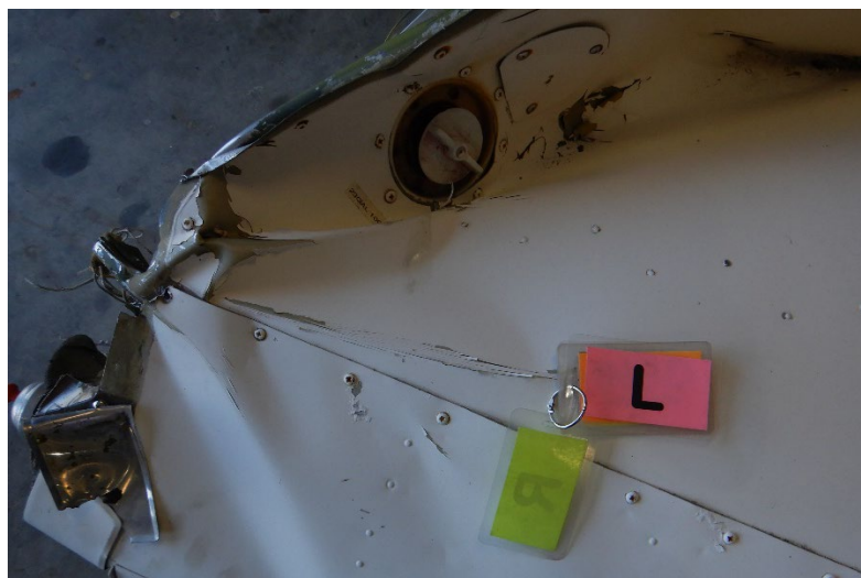
Photo 10 - Left tank fuel port with fuel cap in place.
