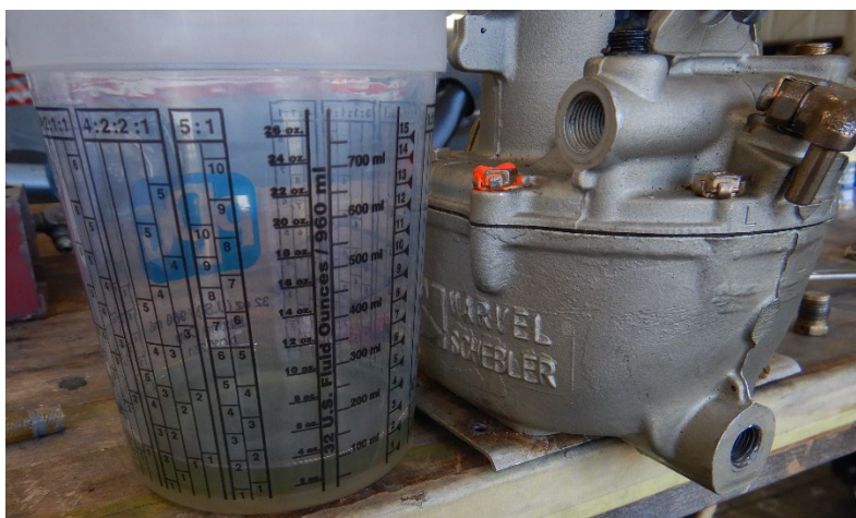
Photo 17 - Liquid recovered from carburetor bowl.
