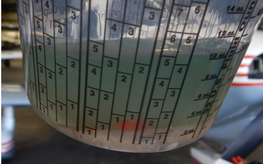
Photo 18 - Contaminated fuel from carburetor and gasolator bowls (combined).
