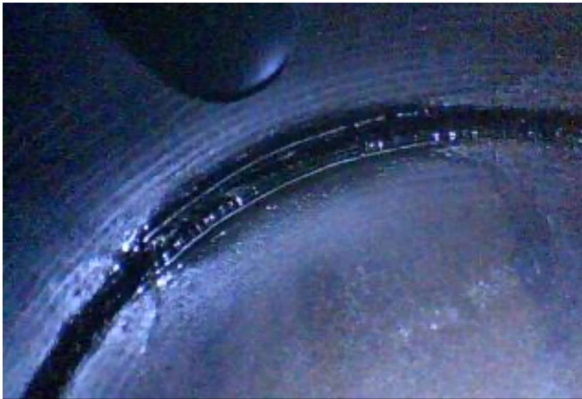
Photo 24 - Borescope photo of cylinder No. 3 with piston rings visible/gap between piston face and cylinder wall.
