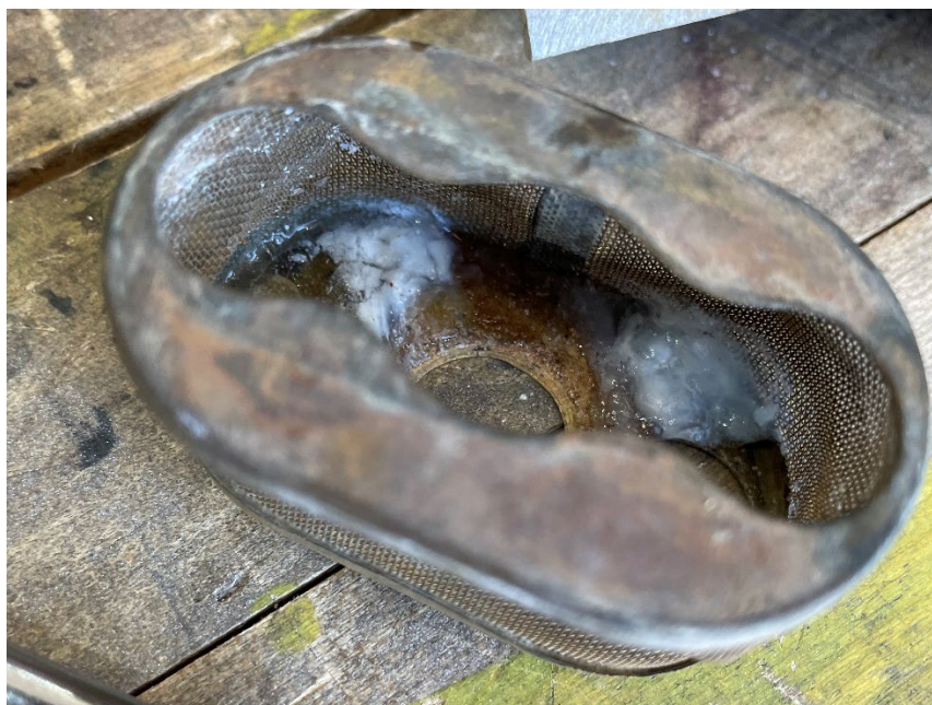
Photo 20 - White gel-like substance within gascolator stainer.
