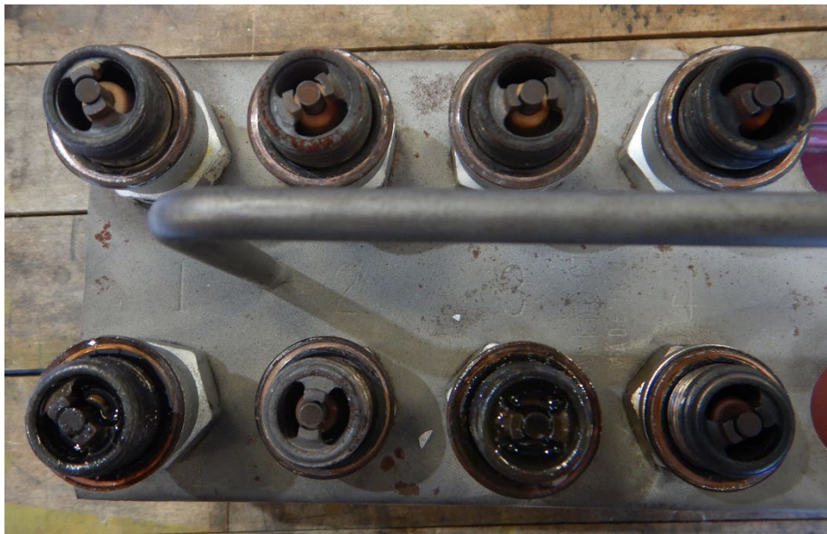
Photo 16 - Spark plugs (lower Nos. 1 and 3 oil fowled).
