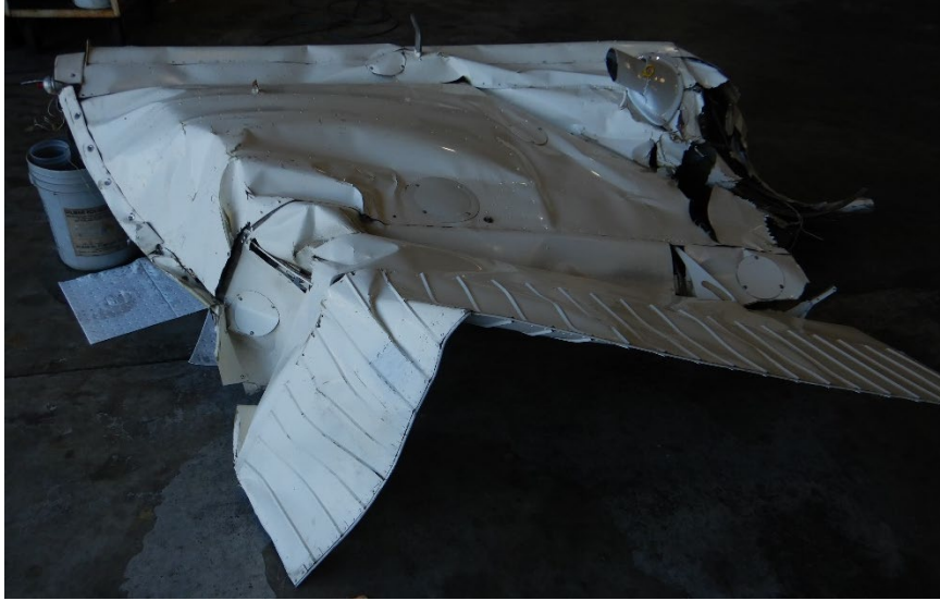
Photo 8 - View of the inboard section of left wing (inverted).
