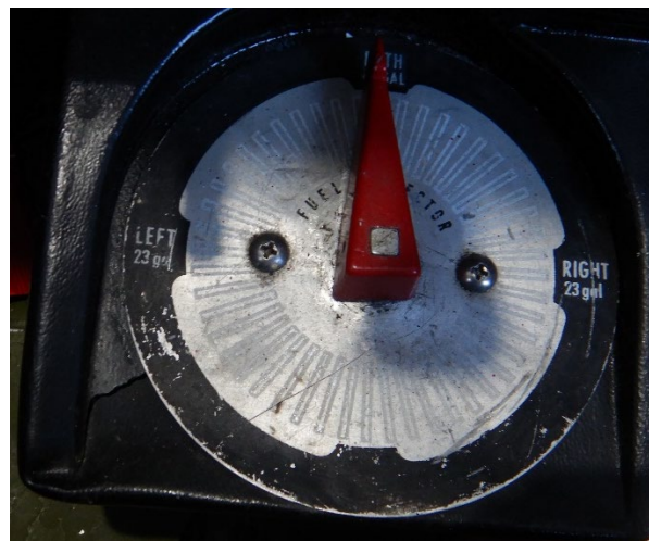
Photo 12 - Fuel selector in BOTH position.
