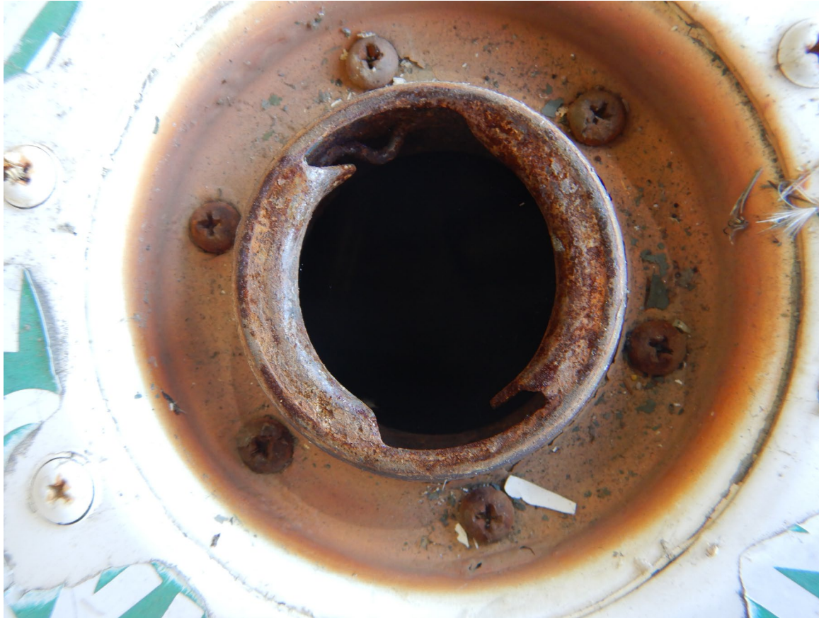
Photograph 6 - Left wing fuel filler port showing rust.
