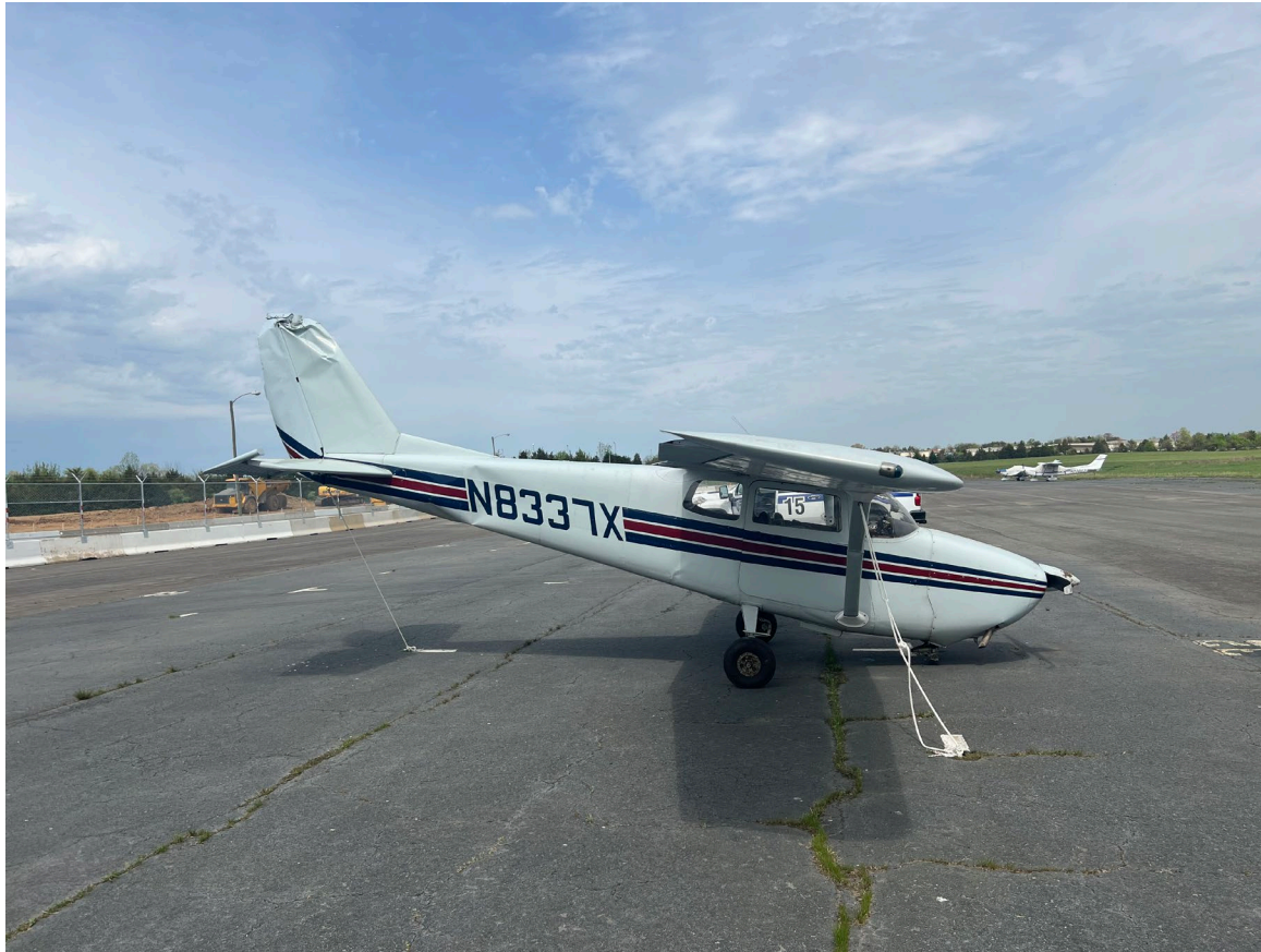
Photograph 2 - Digital Photograph From Airplane Owner. Right Side View of the Airplane Following Recovery. Note the Substantial Damage to the Vertical Stabilizer
