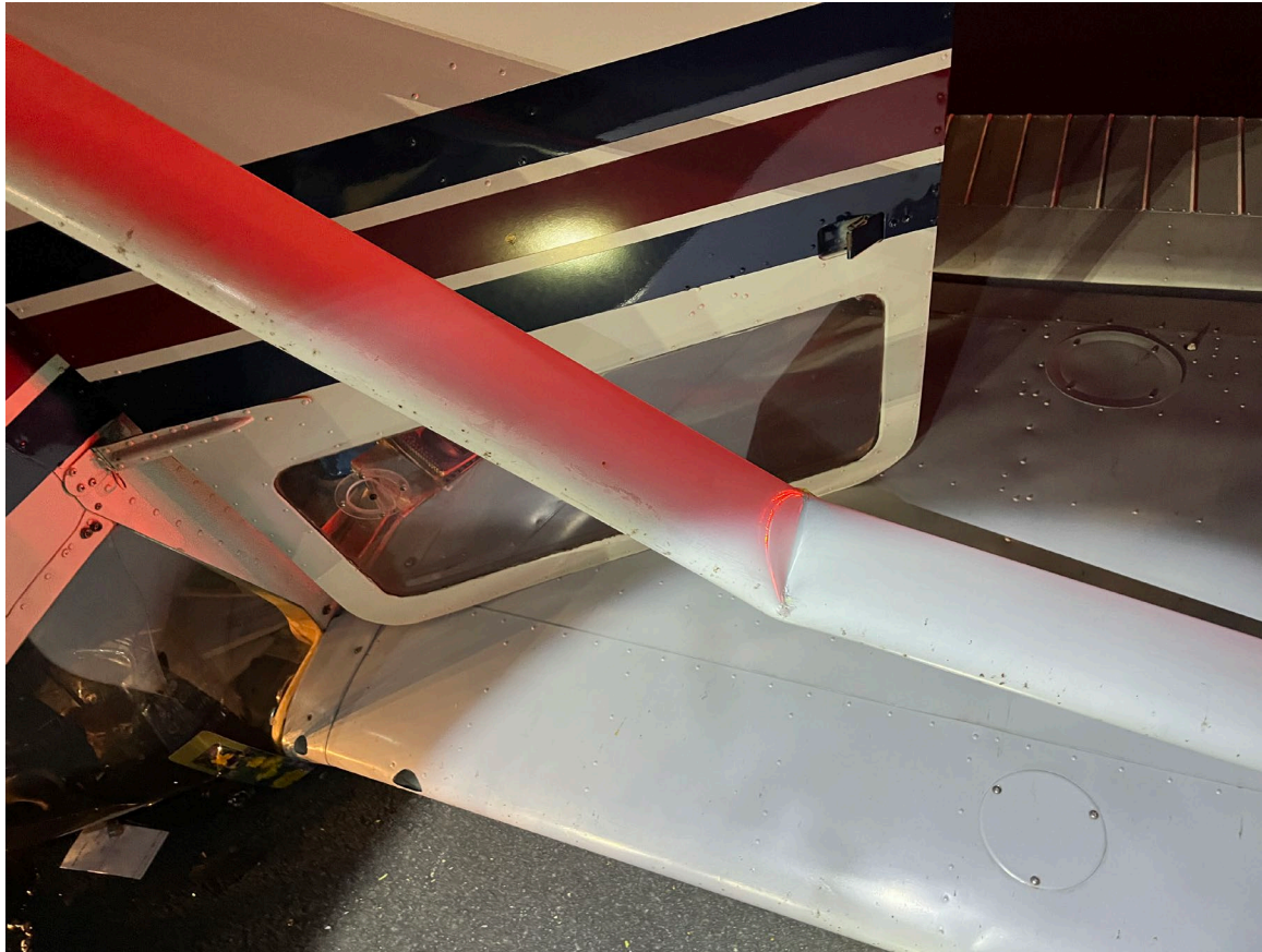
Photograph 3 - Digital Photograph From Airport Personnel. View of Damaged Right Wing Lift Strut
