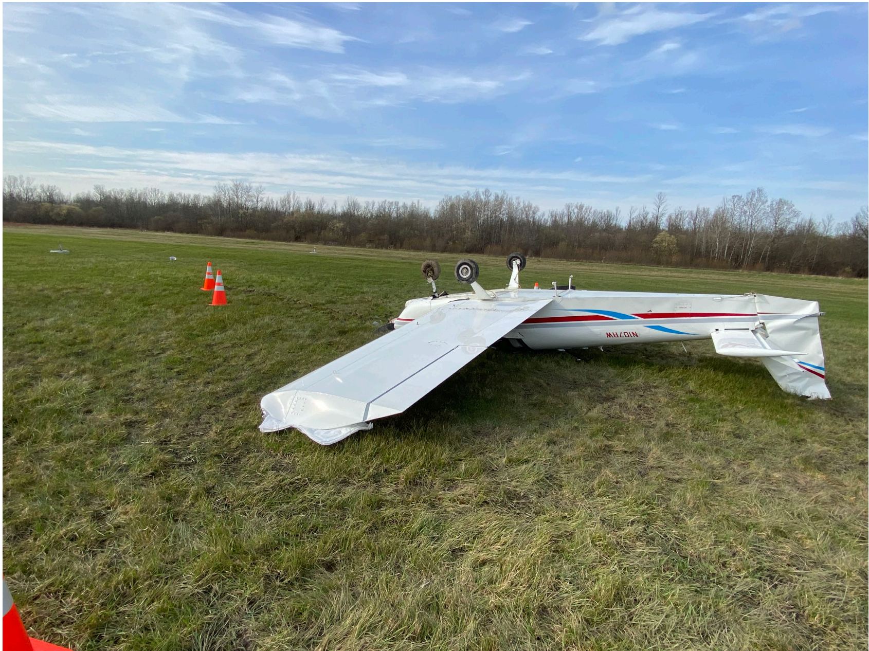
Photo 4 – View of Damage to Vertical Stabilizer as Found (FAA)
