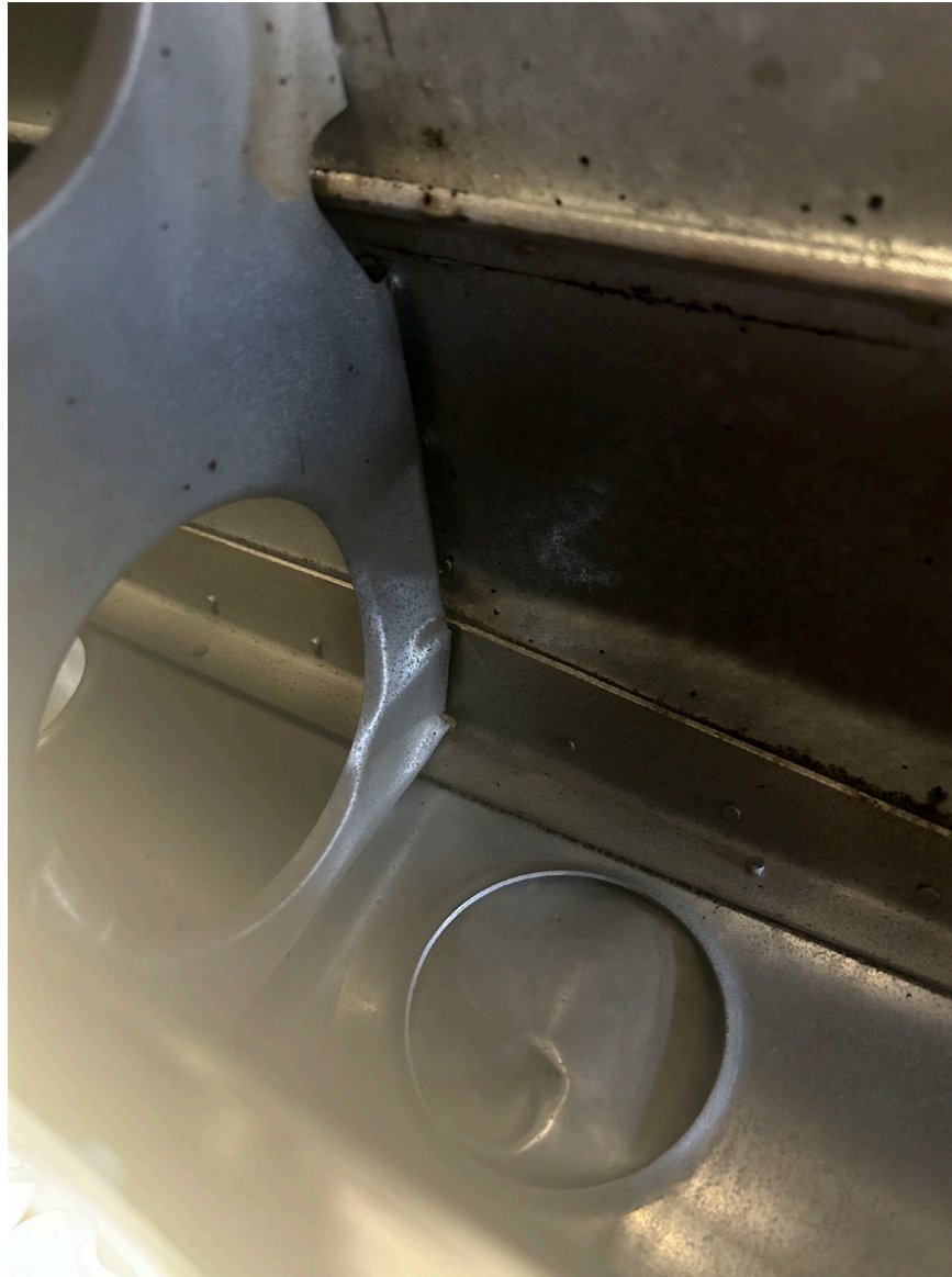
Photograph 4 - Right Wing Spar Damage (Courtesy of FAA)
