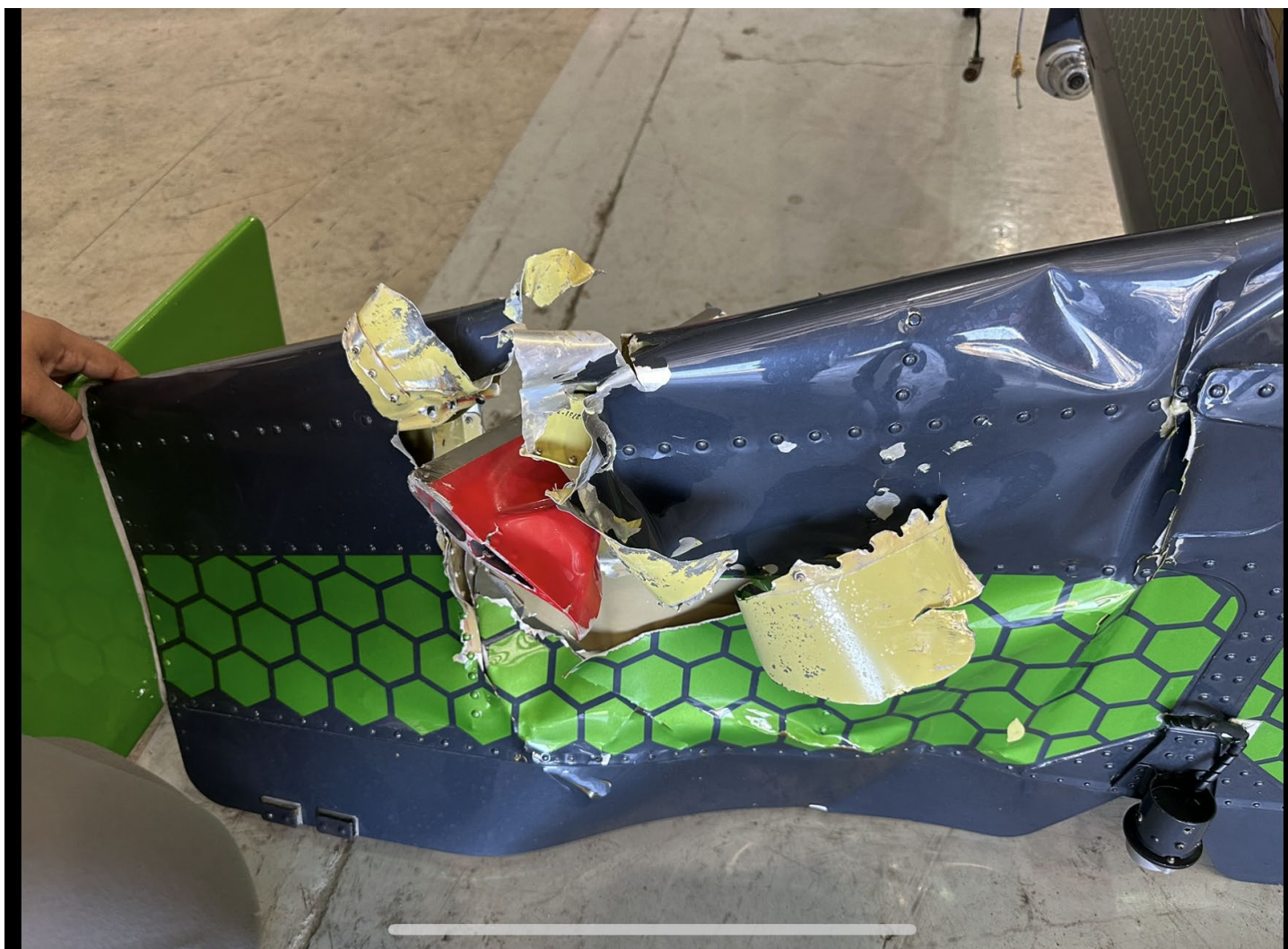
Photograph 2 - View of damage to the horizontal stabilizer. (Courtesy of FAA)
