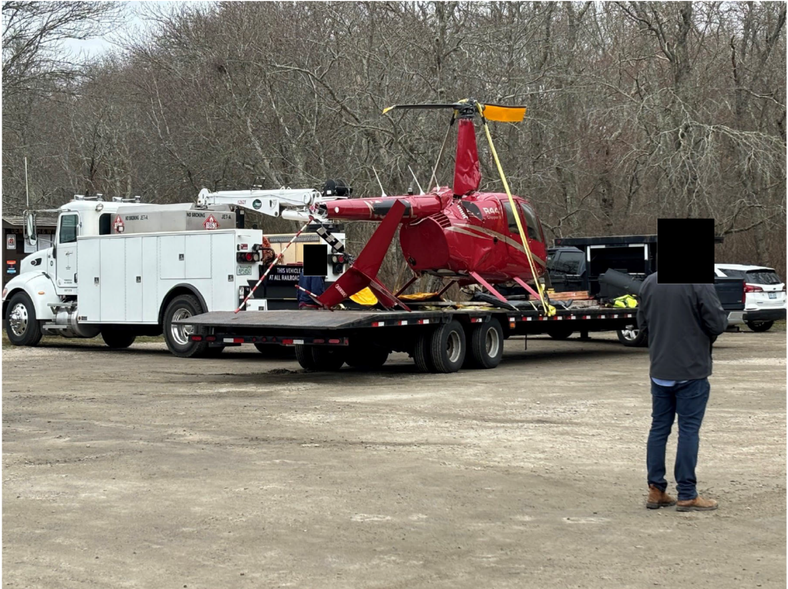
Photograph 2 - Main wreckage on trailer, note: tail boom separated (Courtesy of FAA)
