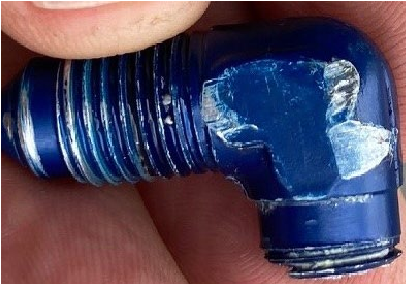
Photo 6: Additional view of the nose gear actuator hydraulic fitting (Photo Courtesy of Operator)
