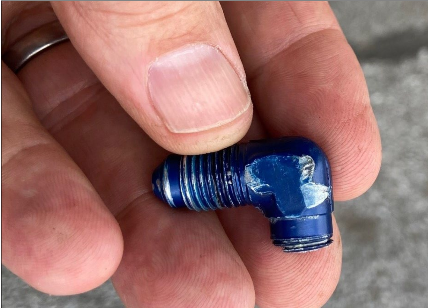
Photo 2: Nose gear actuator hydraulic fitting (Photo Courtesy of FAA)
