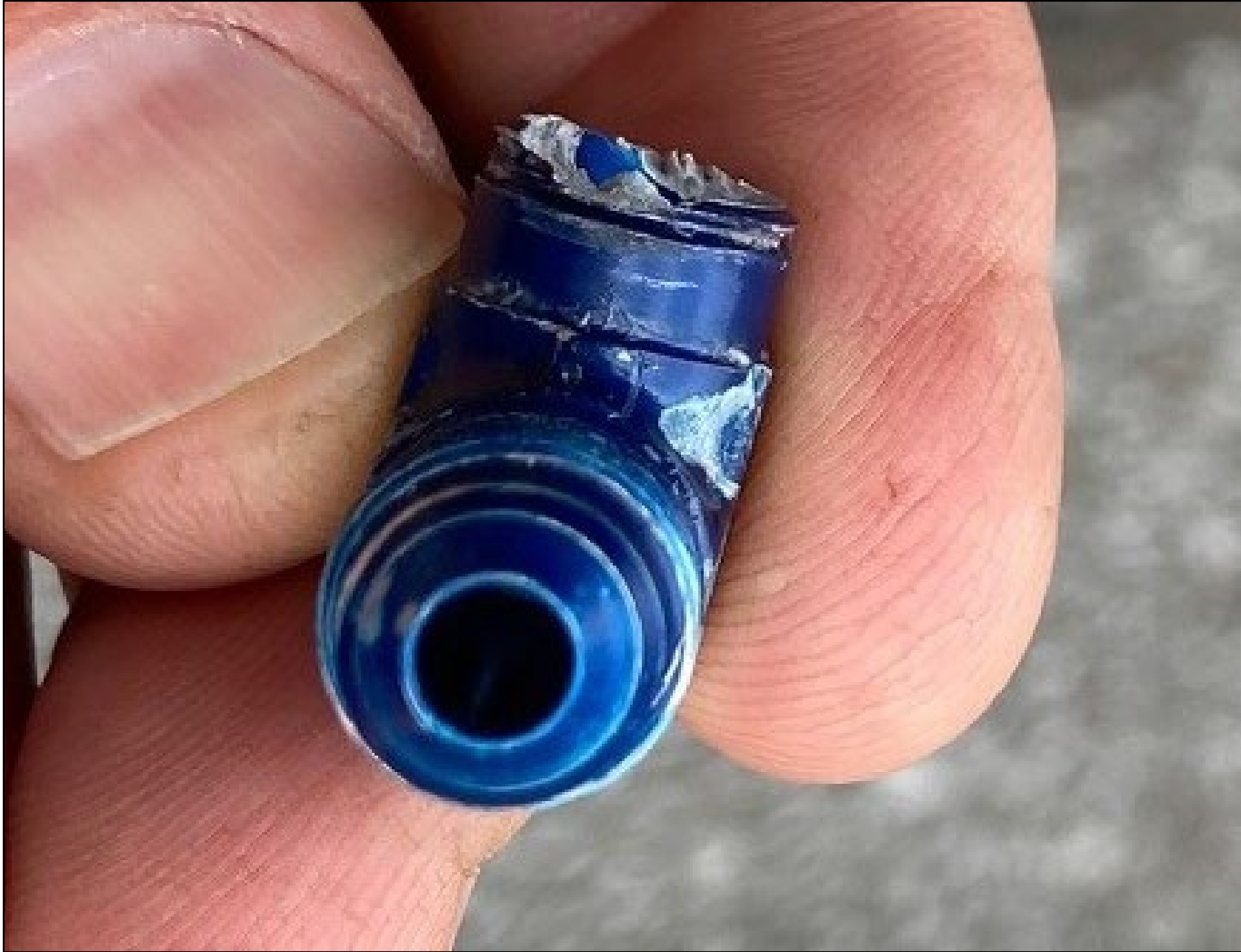
Photo 5: Additional view of the nose gear actuator hydraulic fitting (Photo Courtesy of Operator)
