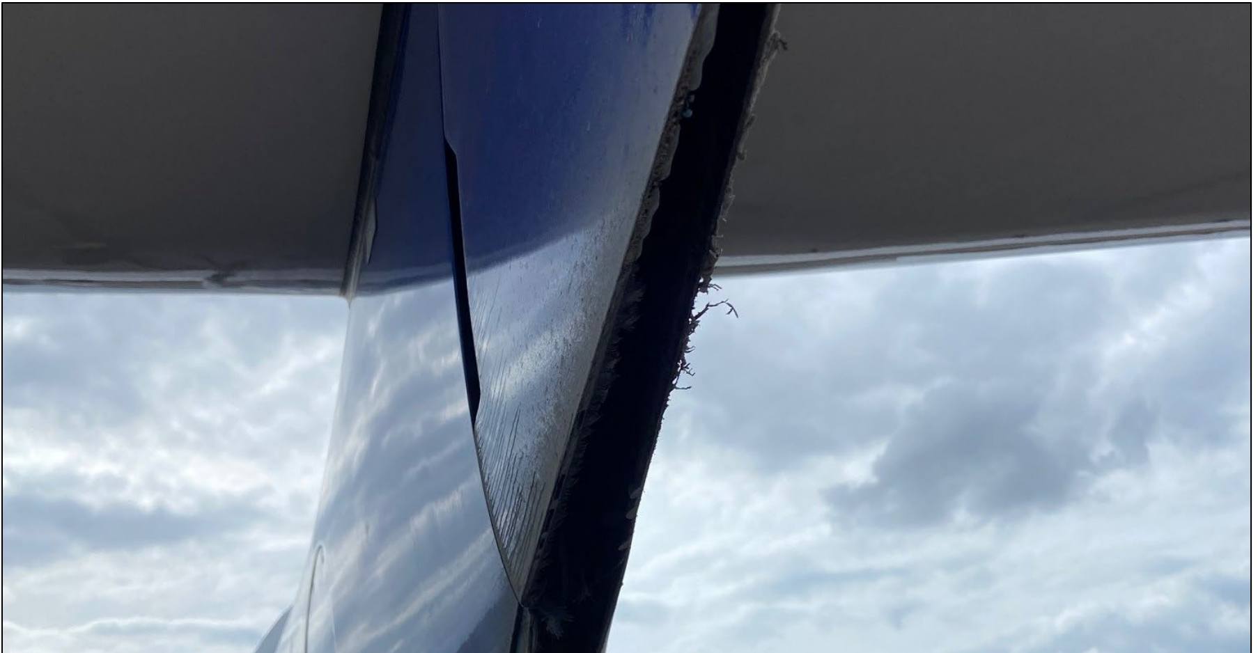
Photo 1: View of the lower rudder damage (Photo Courtesy of FAA)
