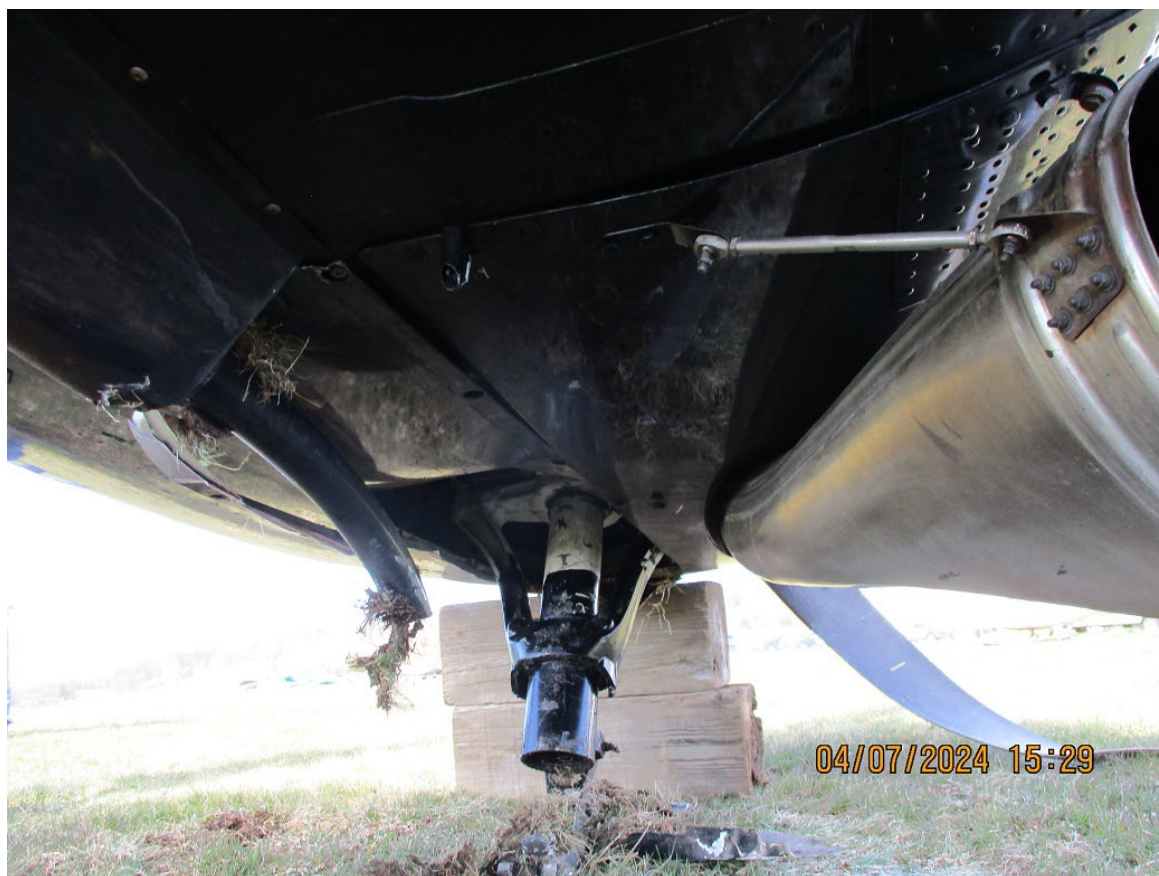
Photograph 4 - Lower Fuselage Damage (Courtesy of FAA)
