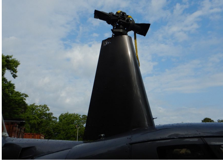
Photo 10 - View of main rotor mast with rotor blades cut for recovery.
