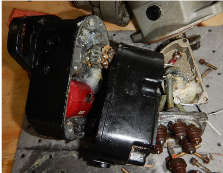
Photo 27 - View of magneto 1 upon removal and disassembly.
