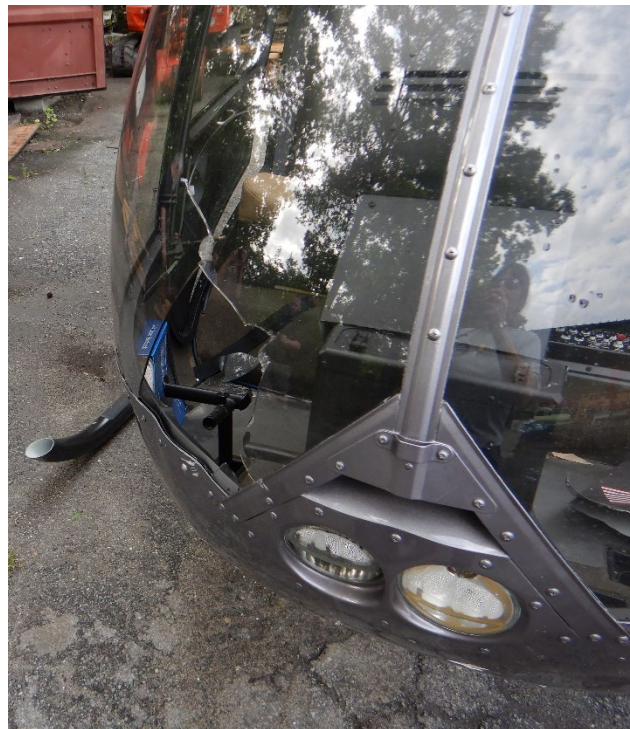
Photo 5 - View of the broken windscreen on forward right of cockpit.
