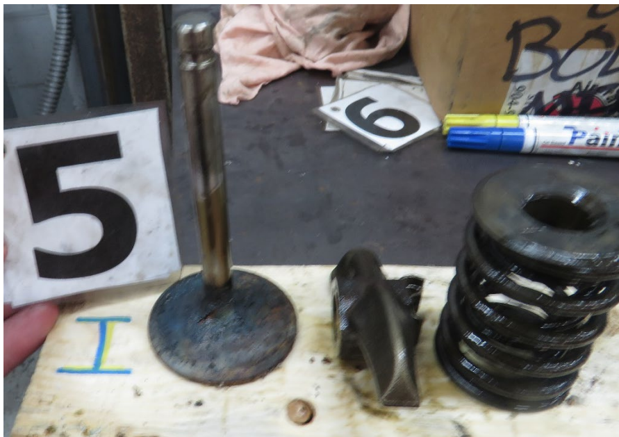
Photo 48 - View of intake valve and spring.
