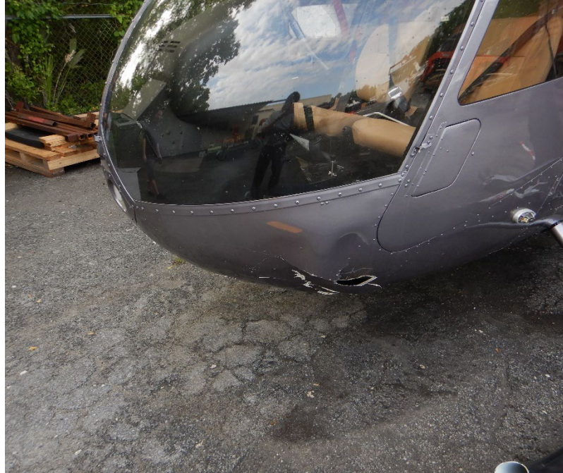
Photo 6 - View of damage to front left of fuselage and windscreen.
