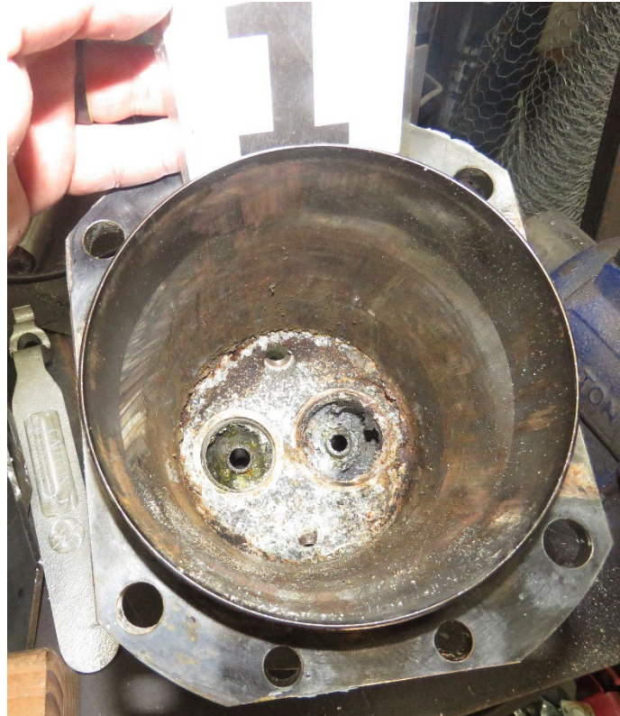
Photo 37 - View of cylinder No. 1 upon removal of valves.
