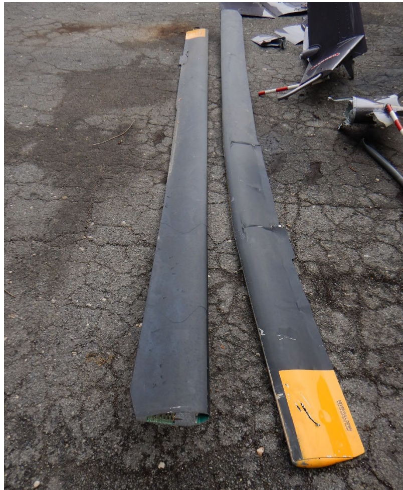
Photo 11 - View of the main rotor blades cut for recovery.
