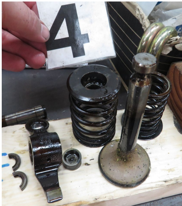
Photo 46 - View of exhaust valve and spring.
