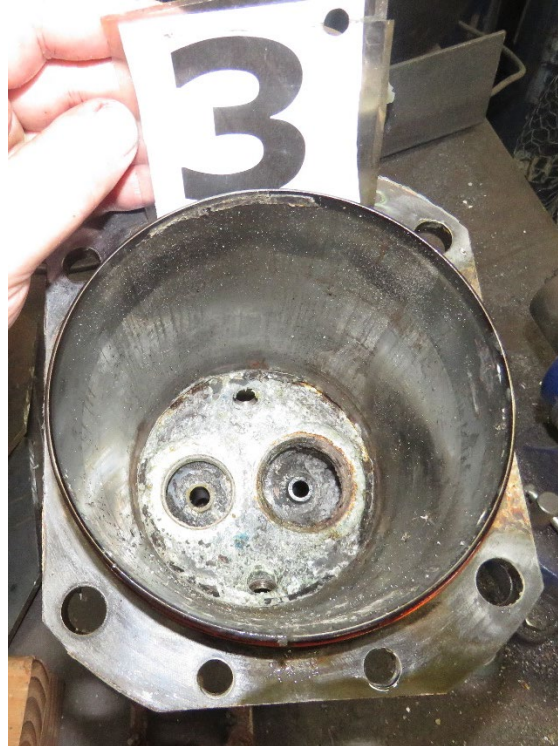
Photo 43 - View of cylinder with valves removed.
