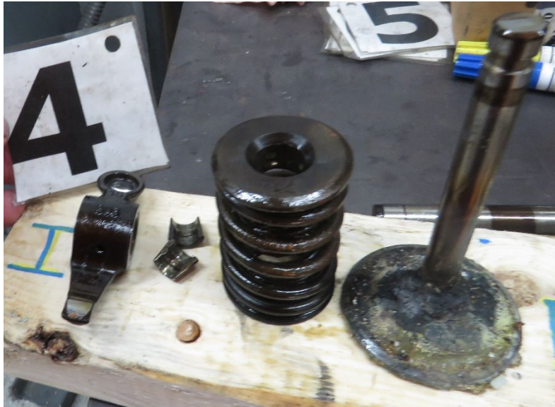
Photo 45 - View of intake valve and spring.
