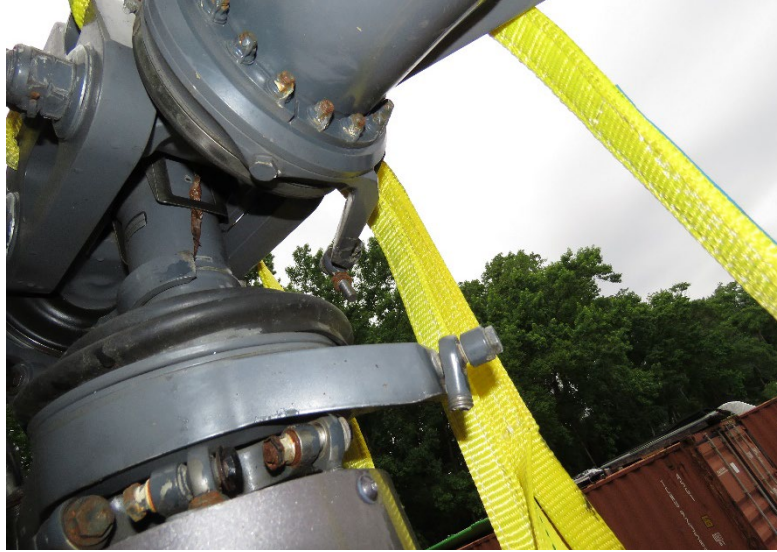
Photo 14 - View of main rotor hub and fractured pitch link.
