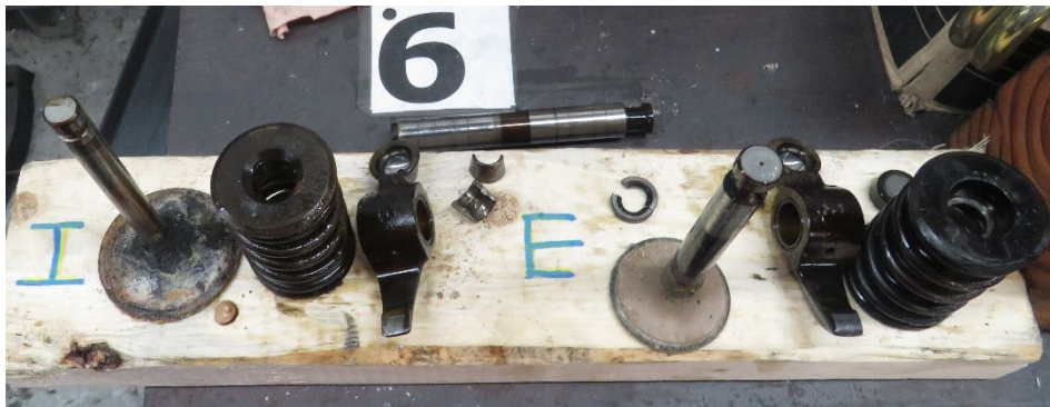
Photo 52 - View of intake and exhaust valves and springs.
