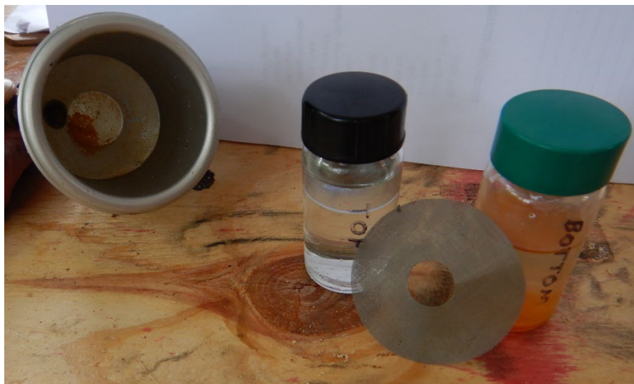
Photo 23 - View of gascolator bowl, screen and recovered contents.
