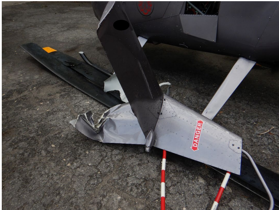
Photo 8 - View of fractured empennage.
