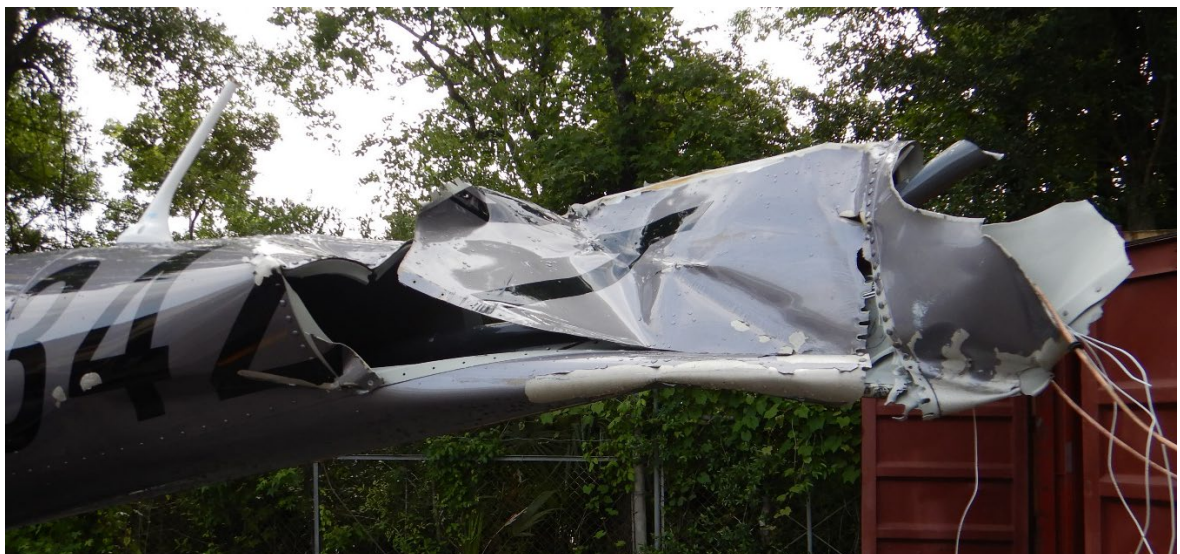
Photo 9 - Close-up view of main rotor contact on tailboom forward of the empennage.
