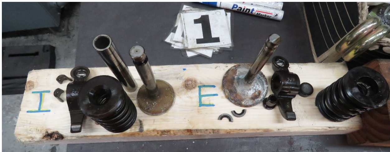
Photo 36 - View of removed valves and springs.
