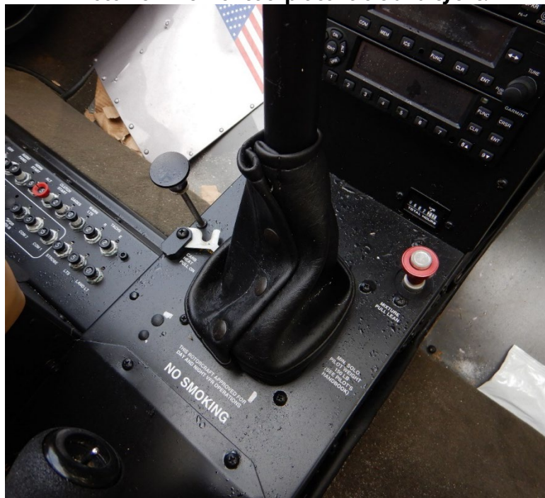
Photo 17 - View of mixture, carburetor heat and circuit breakers.
