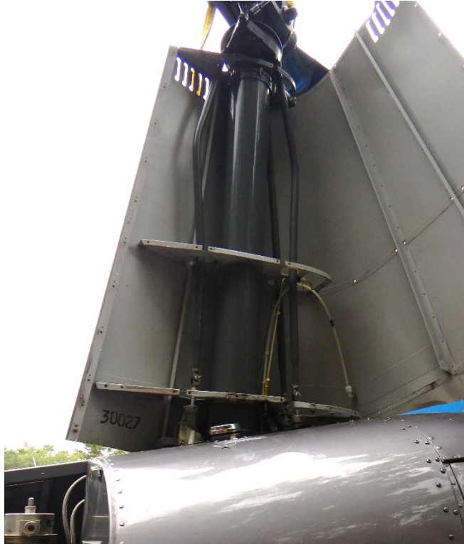
Photo 12 - View of mast fairing interior and deformed control push-pull tubes.
