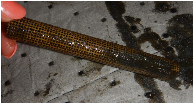
Photo 25 - View of oil suction screen.
