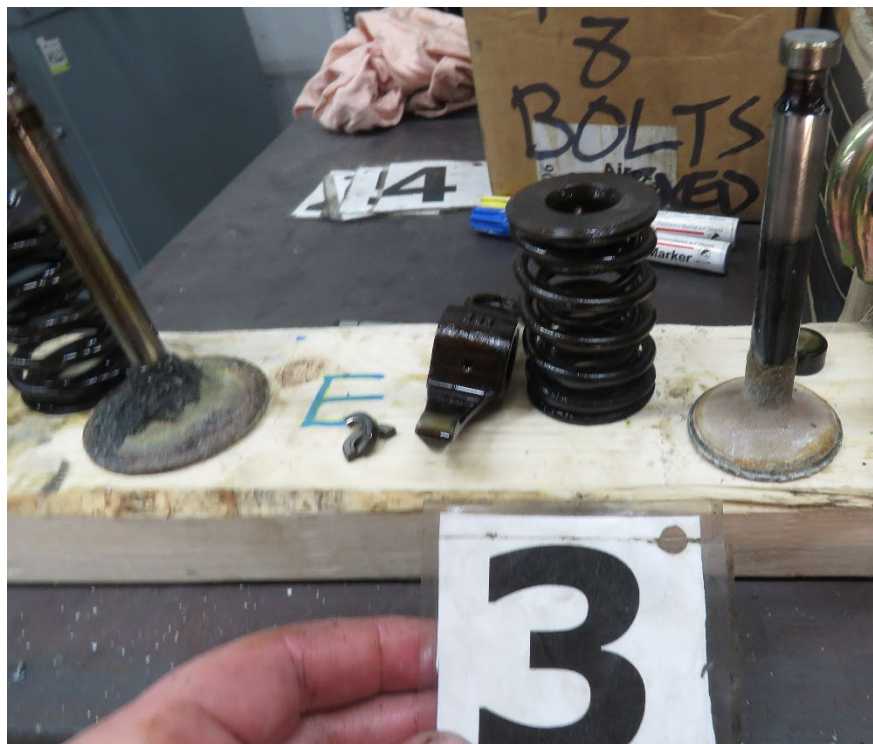
Photo 42 - View of removed valves and springs.
