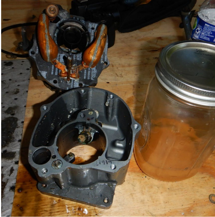
Photo 29 - Opened carburetor and drained fluid.
