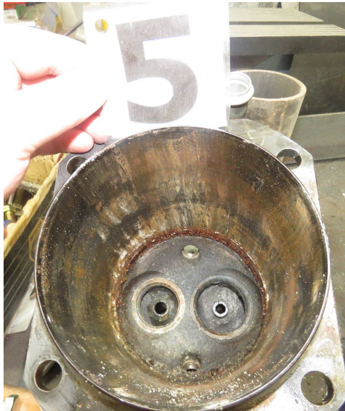
Photo 50 - View of cylinder with valves removed.
