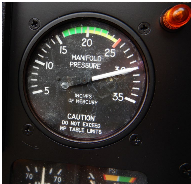
Photo 19 - View of manifold pressure gauge.
