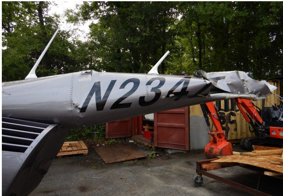
Photo 7 - Close-up view of tailcone fracture.
