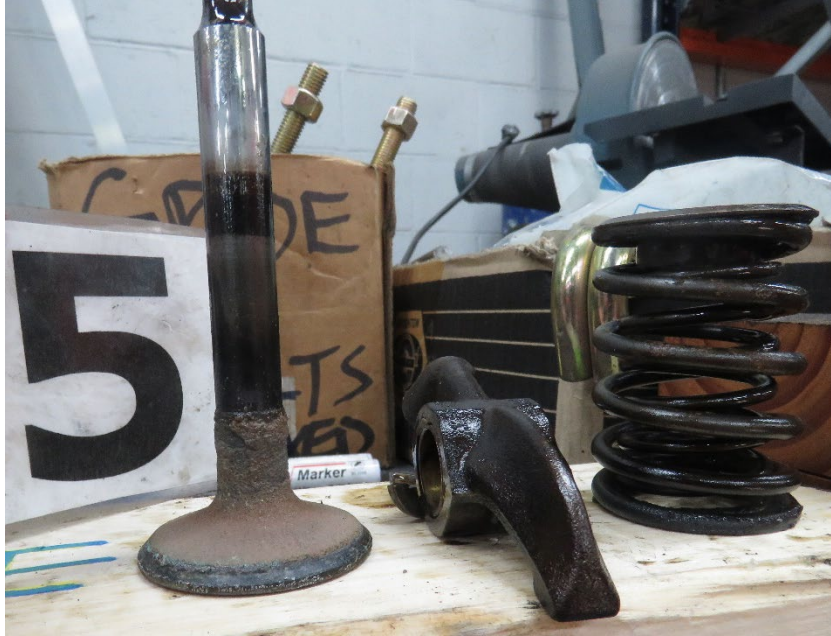
Photo 49 - View of exhaust valve and spring.
