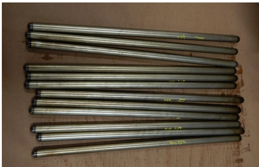
Photo 32 - View of removed pushrods.
