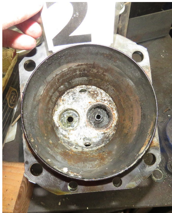
Photo 40 - View of cylinder No. 2 with valves removed.
