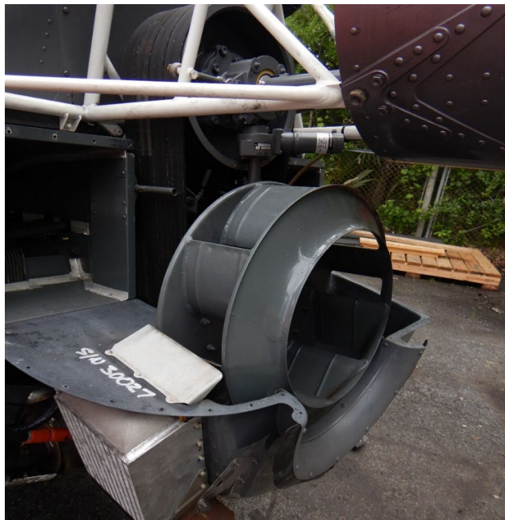
Photo 13 - View of scroll/cooling fan.
