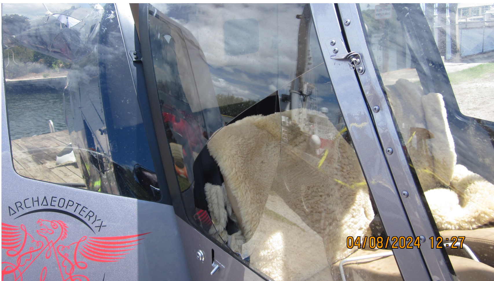
Photograph 3 - View of hole in cockpit window. (Courtesy of FAA)
