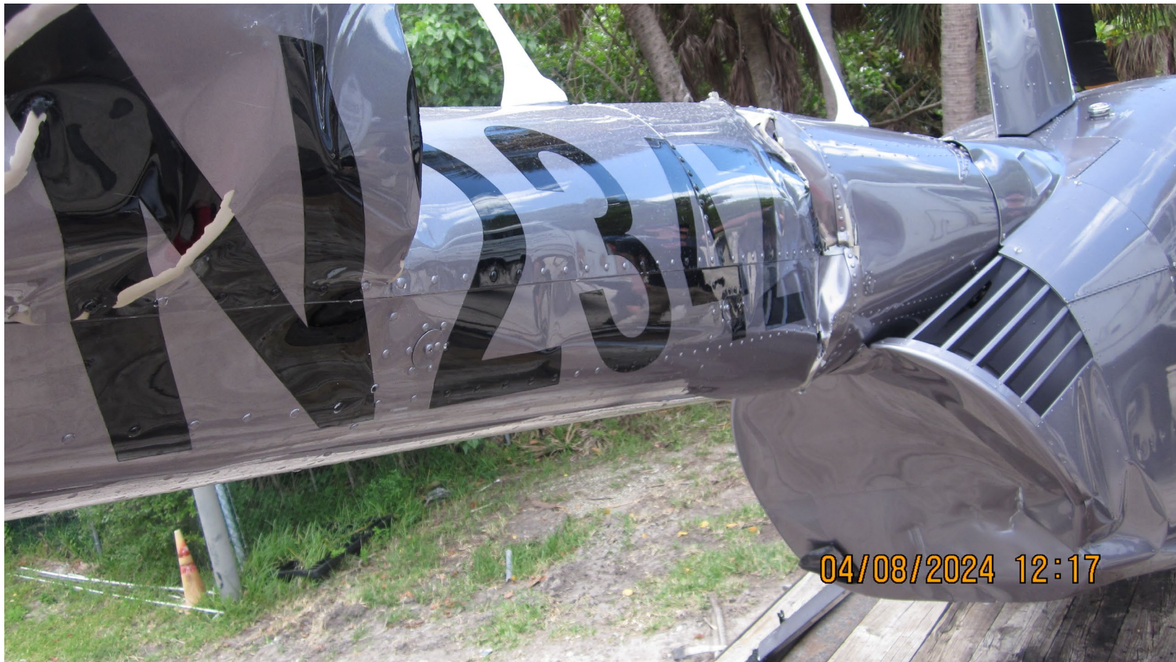
Photograph 2 - View of tailcone damage. (Courtesy of FAA)
