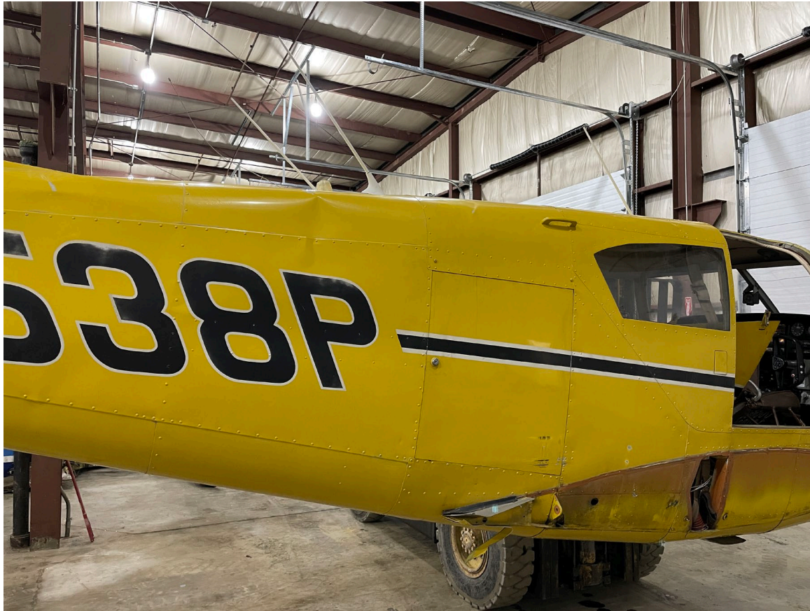
Photograph 3 - Right Side of Aft Fuselage. Note Compression Wrinkle in Fuselage Skin (Courtesy of FAA)
