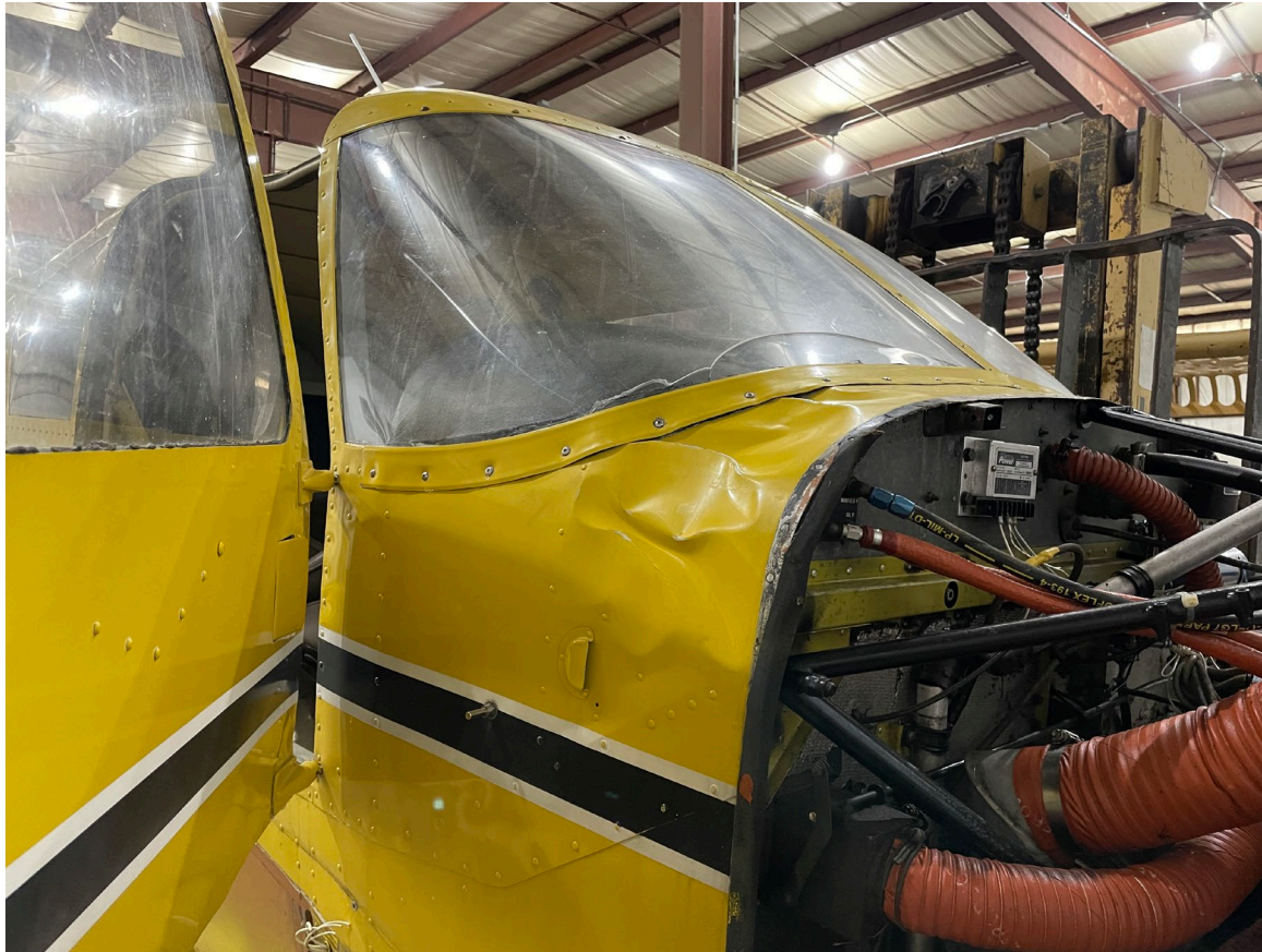
Photograph 4 - Right Forward Quartering View of the Forward Fuselage. Note the Extensive Skin Damage Aft of the Firewall (Courtesy of FAA)
