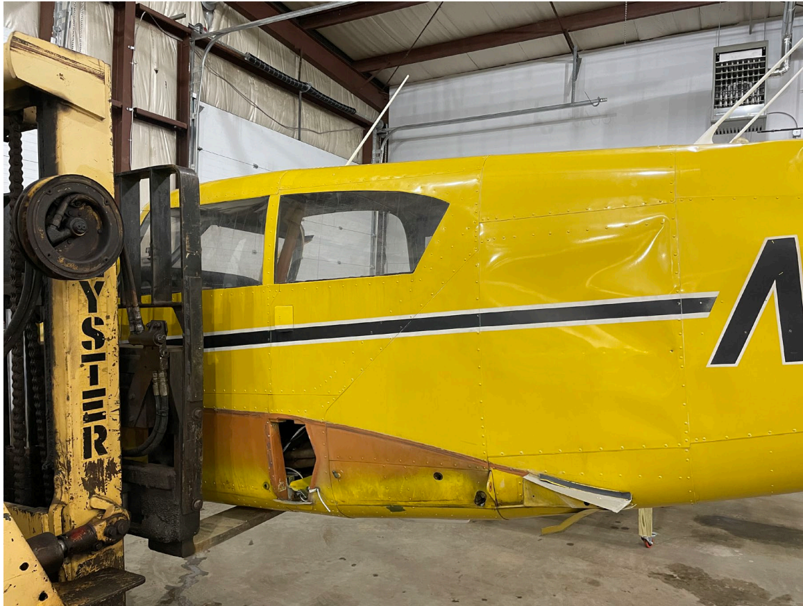
Photograph 2 - Left Side View of Aft Fuselage. Note large Dent (Courtesy of FAA)
