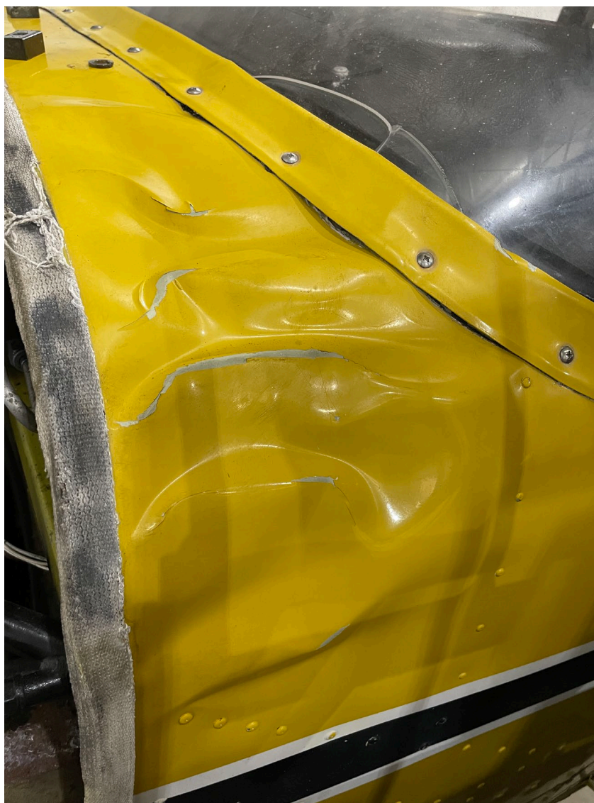
Photograph 5 - Left Side View of the Forward Fuselage. Noted the Extensive Skin Damage Aft of the Firewall (Courtesy of FAA)
