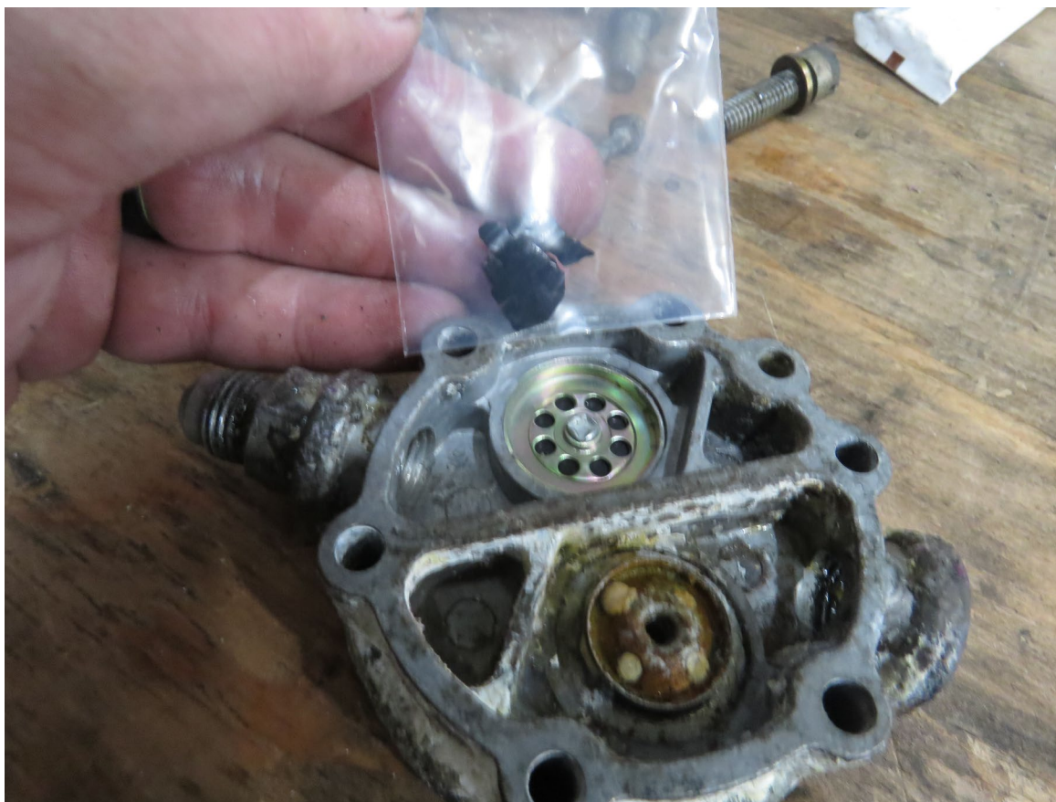
Photograph 6 - View of the Disassembled Engine-Driven Fuel Pump Showing the Foreign Object Found Inside the Pump (Courtesy of Lycoming)
