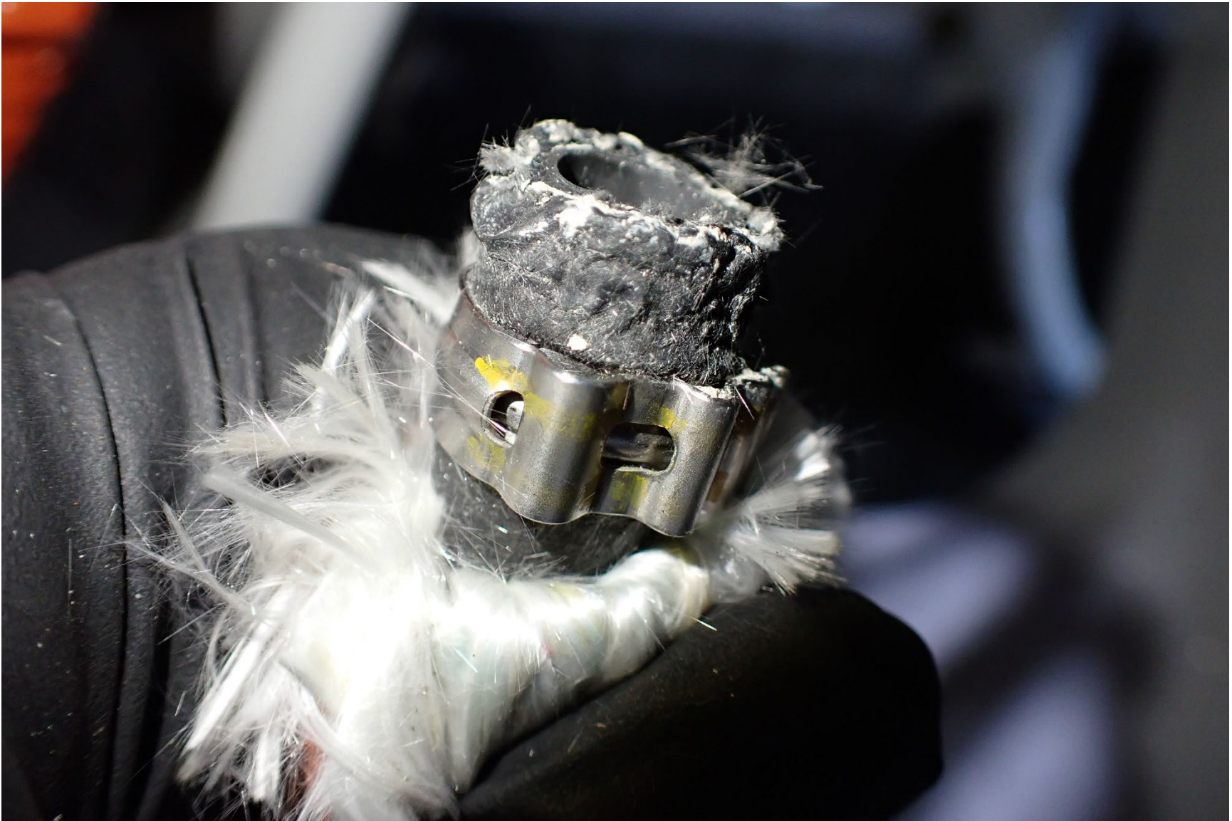
Photograph 5 – Disconnected fuel line with clamp installed
