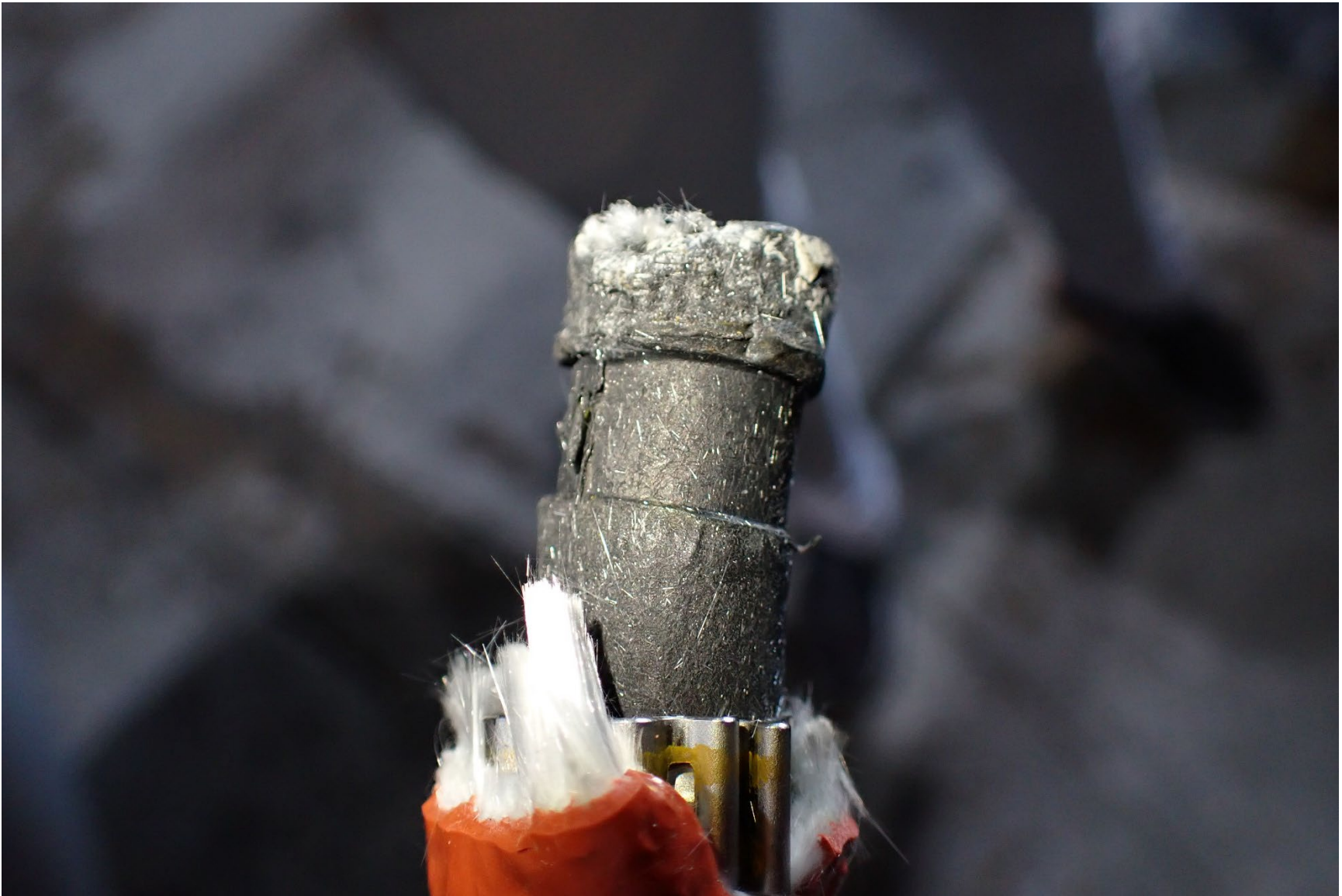
Photograph 7 – Disconnected fuel line after clamp was moved
