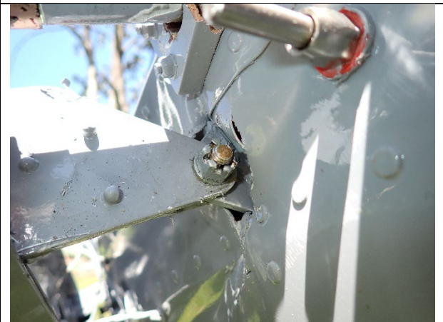
Photograph 4: Right, rear wing attach bolt and nut with missing securing pin
