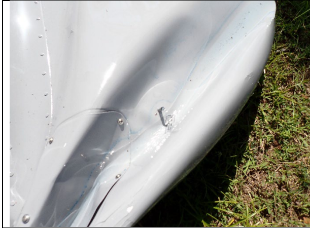
Photograph 5: Fuel draining from the right fuel vent
