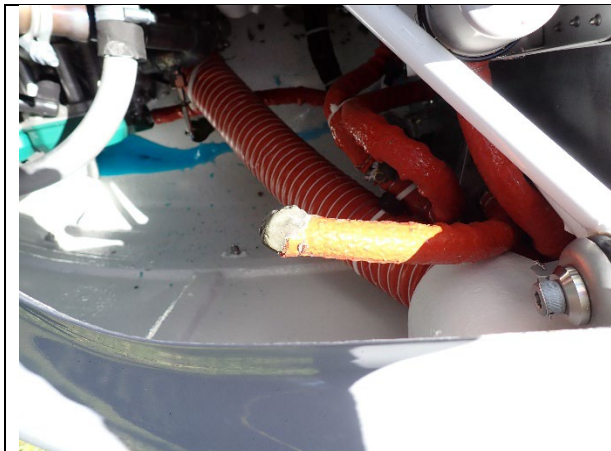
Photograph 7: Disconnected fuel line (with putty)
