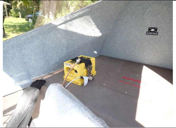
Photograph 10: ELT installed with disconnected wiring
