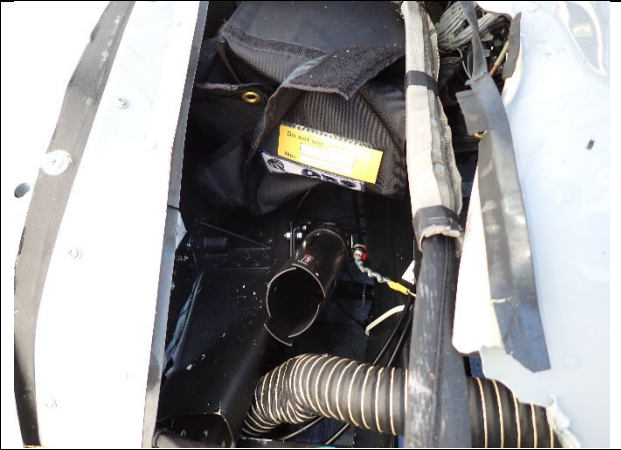
Photograph 2: Whole airplane parachute system rocket launch tube
