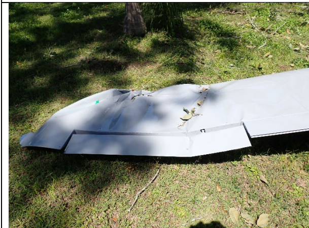
Photograph 3: Damage to the right wing
