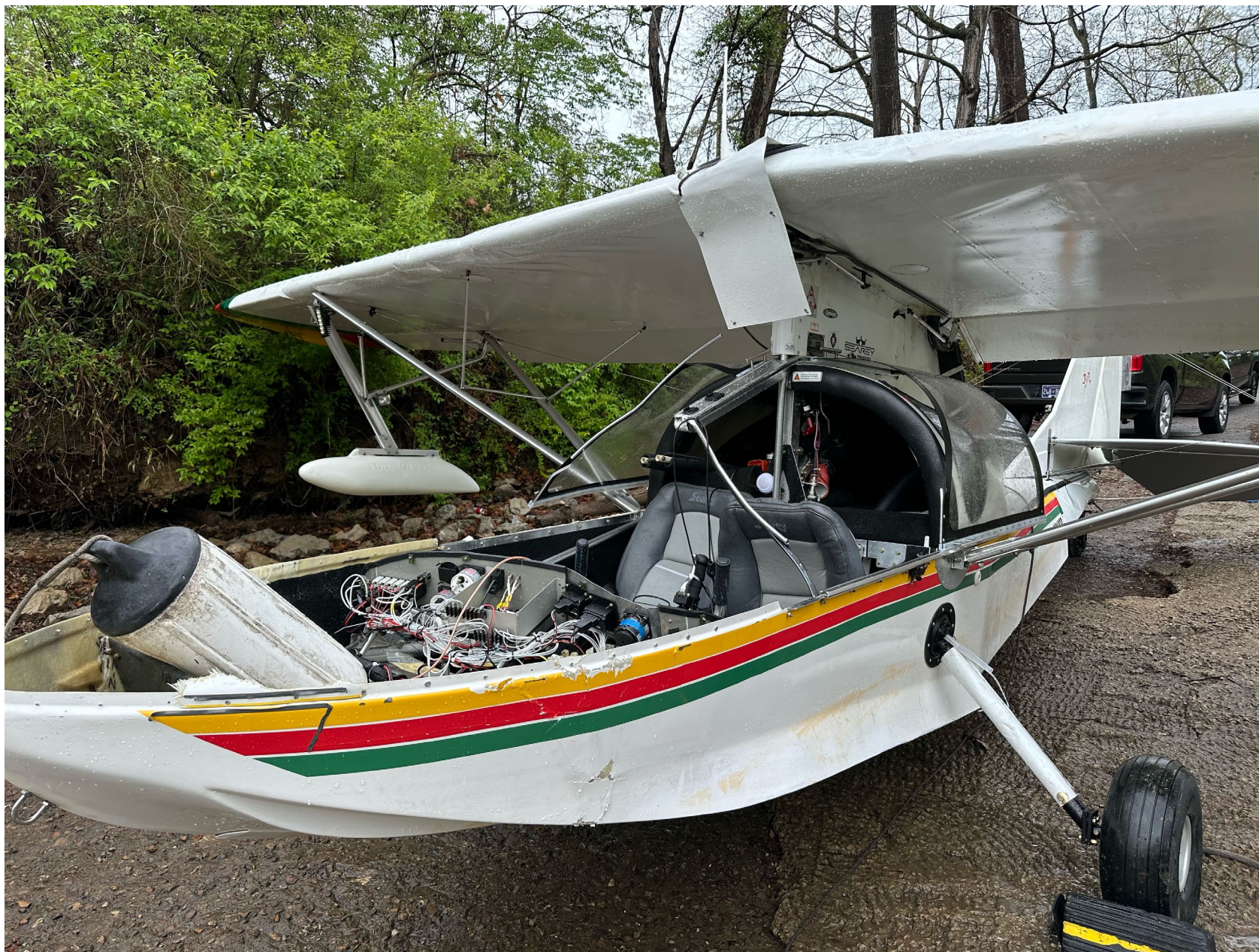
Photo 2 – View of Structural Damage to Hull and Center Beam above Cockpit (FAA)
