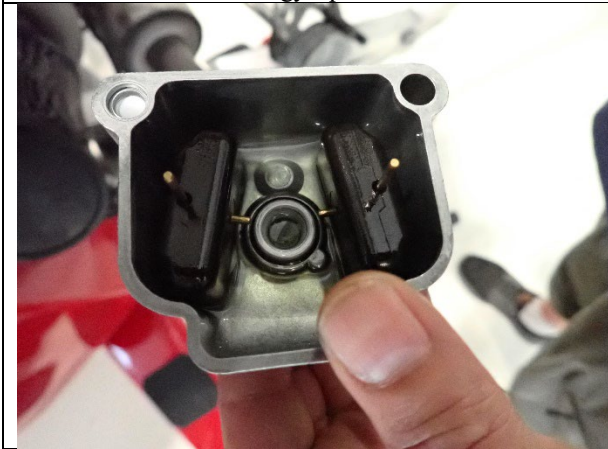
Figure 7: Carburetor "A" bowl and floats with fuel
