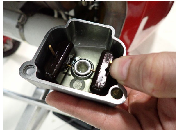
Figure 8: Carburetor "B" bowl and floats with fuel
