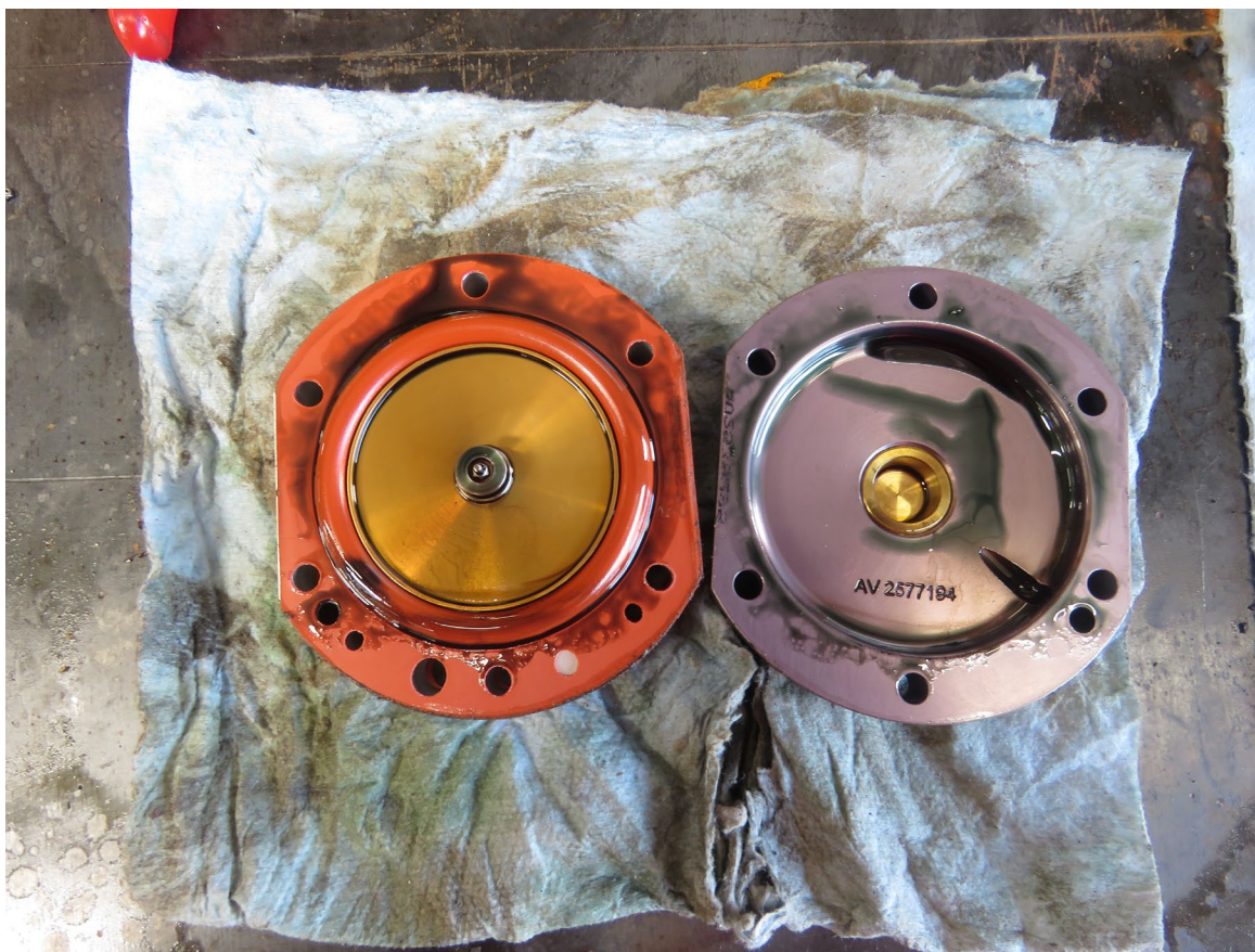
Photograph 3 - View of contamination found in the fuel servo. (Courtesy of Lycoming)
