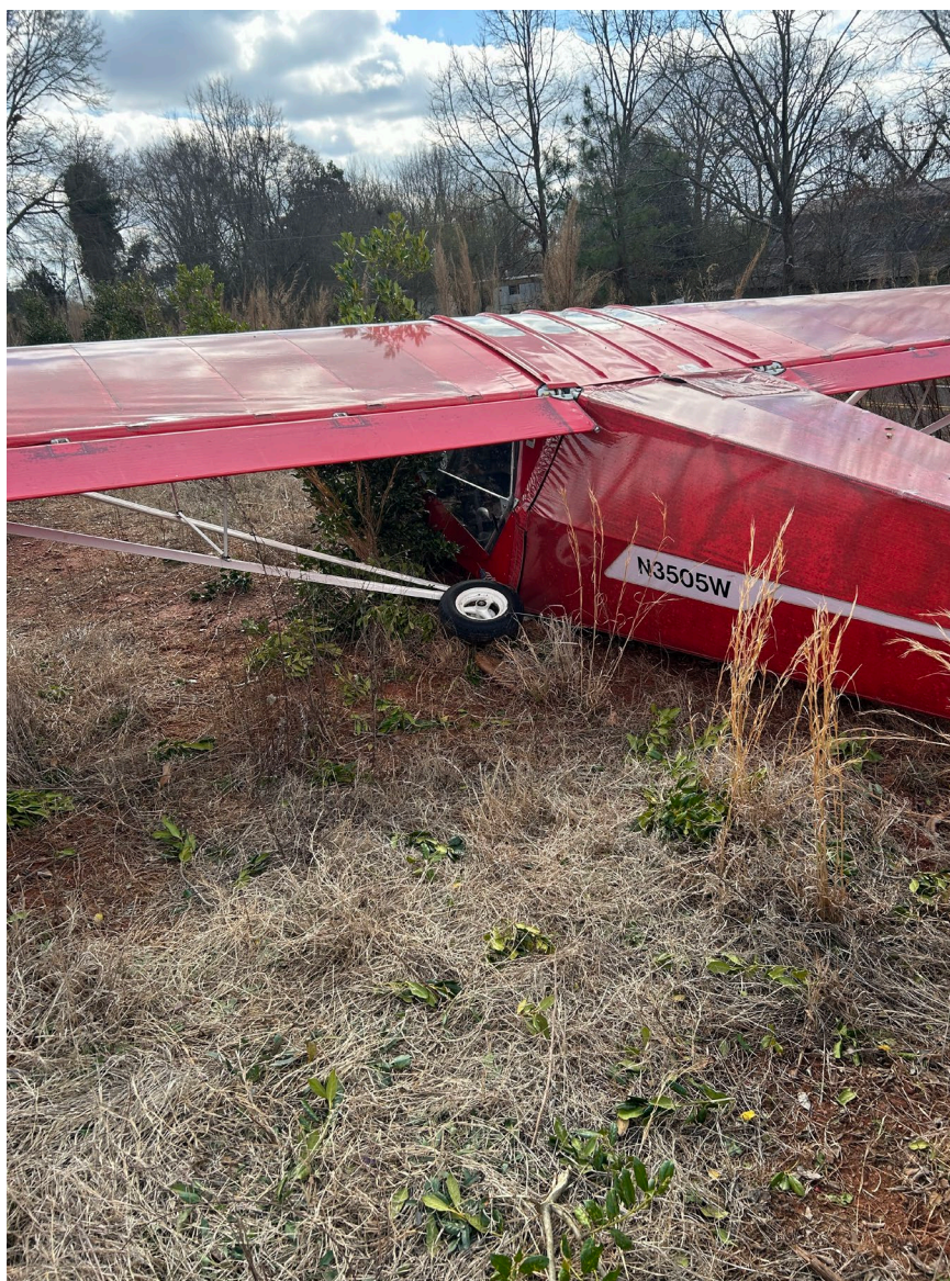
Photograph 2 -Collapsed Gear and Fuselage Damage (Courtesy of Owner)
