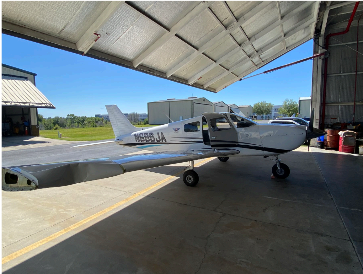
Photograph 2 - FAA Digital Photograph. Right Forward Quartering View of the Airplane. Note the Damage to the Leading Edge of the Right Wing Near the Wingtip
