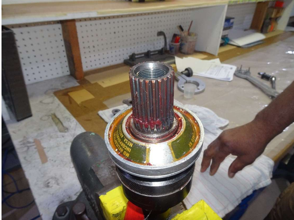
Figure 4. The output splines of the clutch subassembly.
