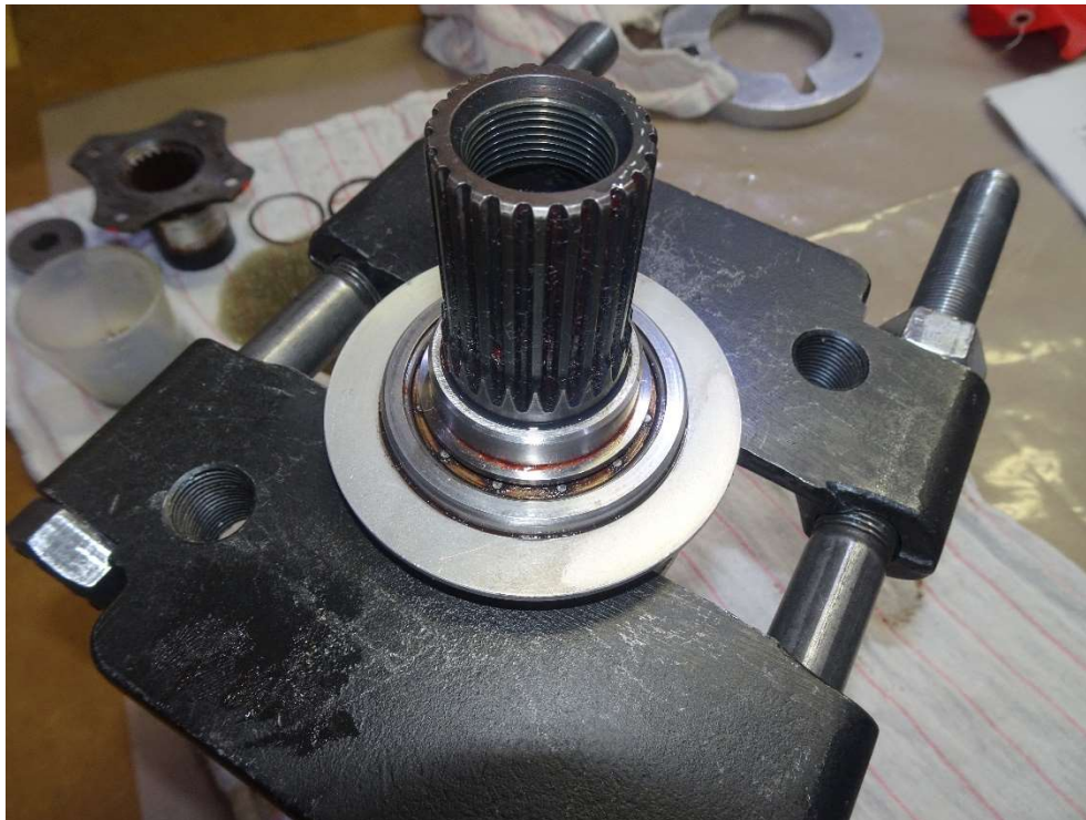
Figure 5. The output bearing and lower bearing carriers. (Tool to remove the output bearing is installed in this photo.)
