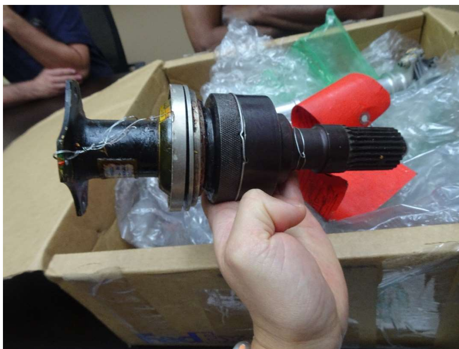
Figure 3. The overrunning clutch subassembly.
