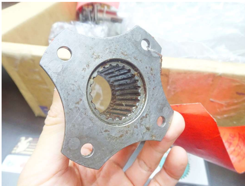
Figure 2. The main transmission input coupling.
