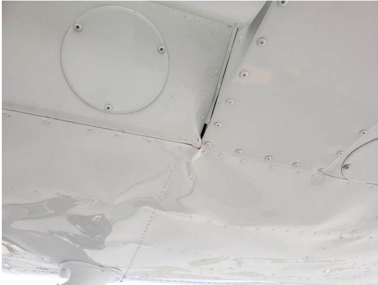
Photograph 3 - Lower Surface of Wing (Courtesy of Embry Riddle)
