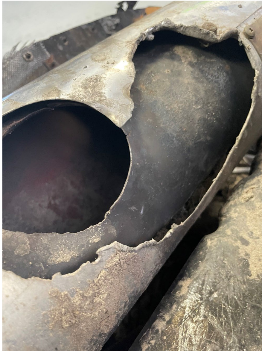
Photograph 3 - Muffler with missing pipe and melted cover. (Courtesy of FAA)
